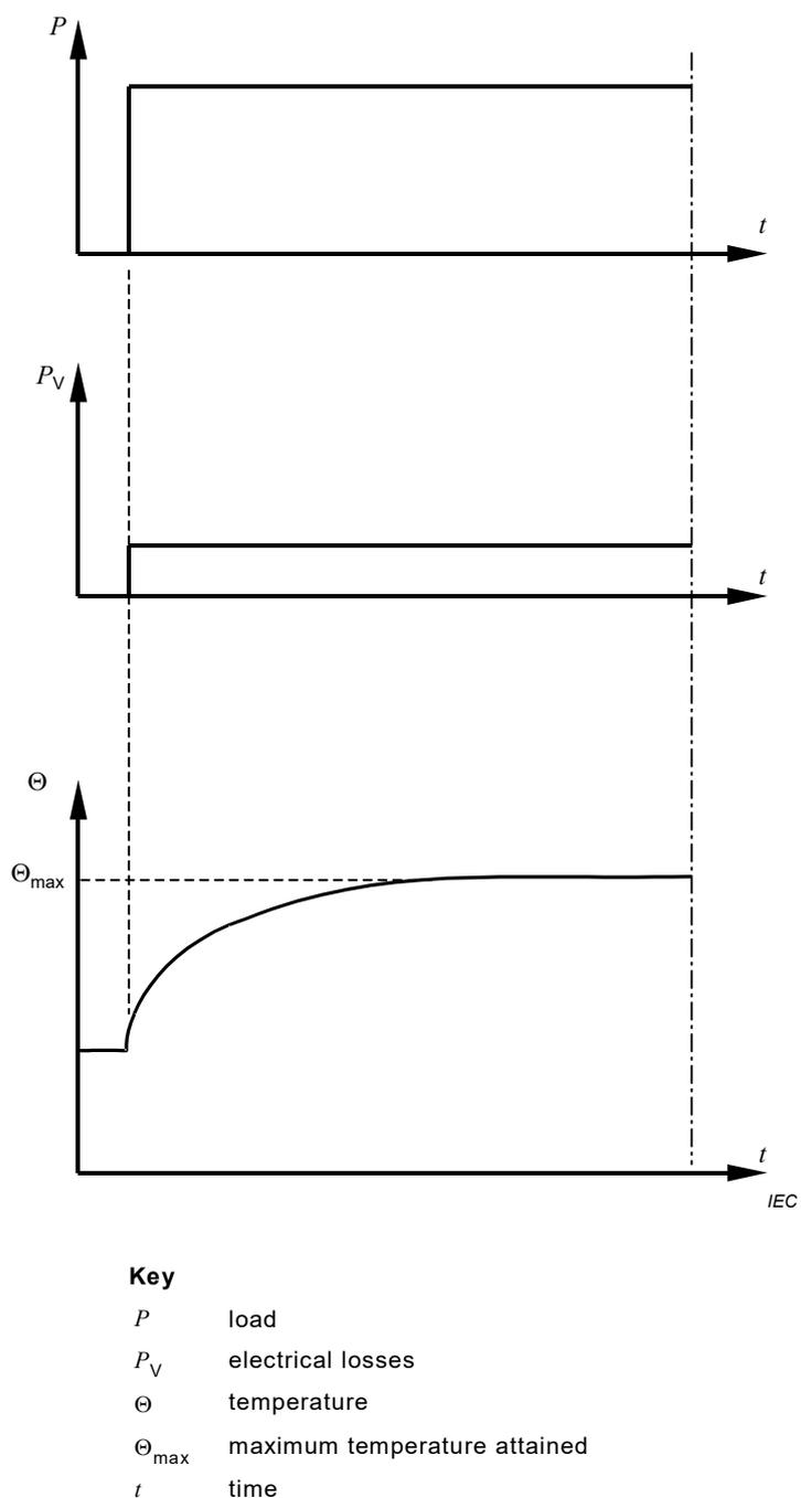
**Figure 1 – Continuous running duty – Duty type S1**
