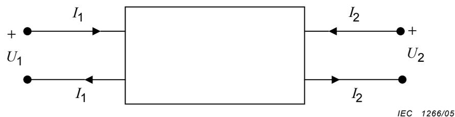
**Figure 1 – Conventions concerning signs in electric circuits**
