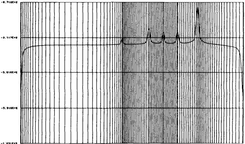
FIG. 11—Pipe with defect buried in mud, voltage mV.
