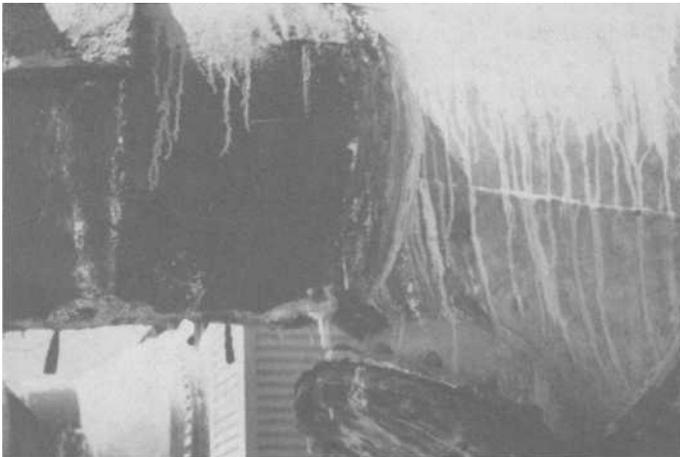
FIG. 3—Perforations in steel pipe.
