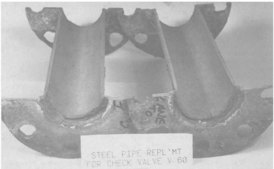
FIG. 2—Steel pipe replacement section attached to copper-nickel pipe after cleaning.
