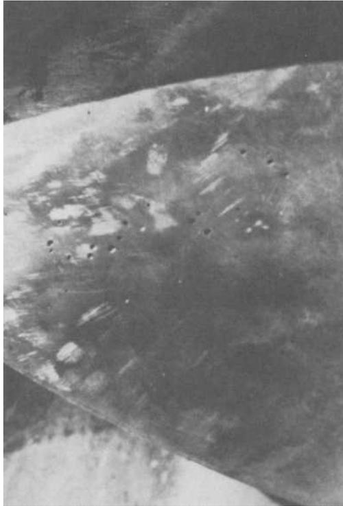
FIG. 4—Pitting of Alloy 20 impeller.
