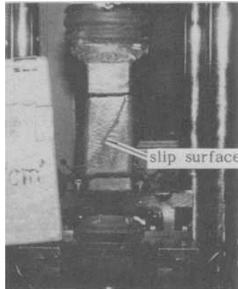
FIG. 17—Specimen after plane strain test (Seto sand, \sigma_x = 4 \text{ kgf/cm}^2 ).
