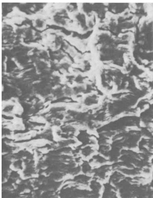
(b) \Delta K = 23.9 \text{ ksi}\sqrt{\text{in.}} ( 26.5 \text{ MPa}\sqrt{\text{m}} ) |5\mu\text{m}|
