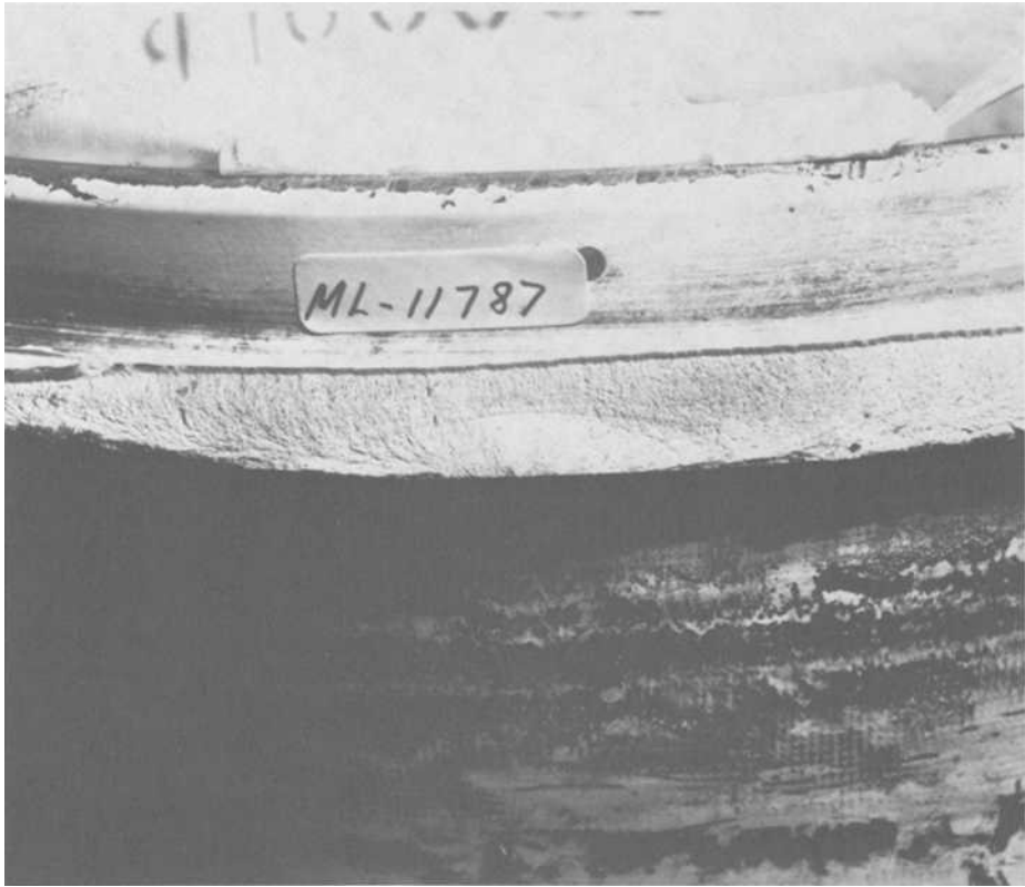
FIG. 7— Fracture surface of a typical wheel flange failure in service.
