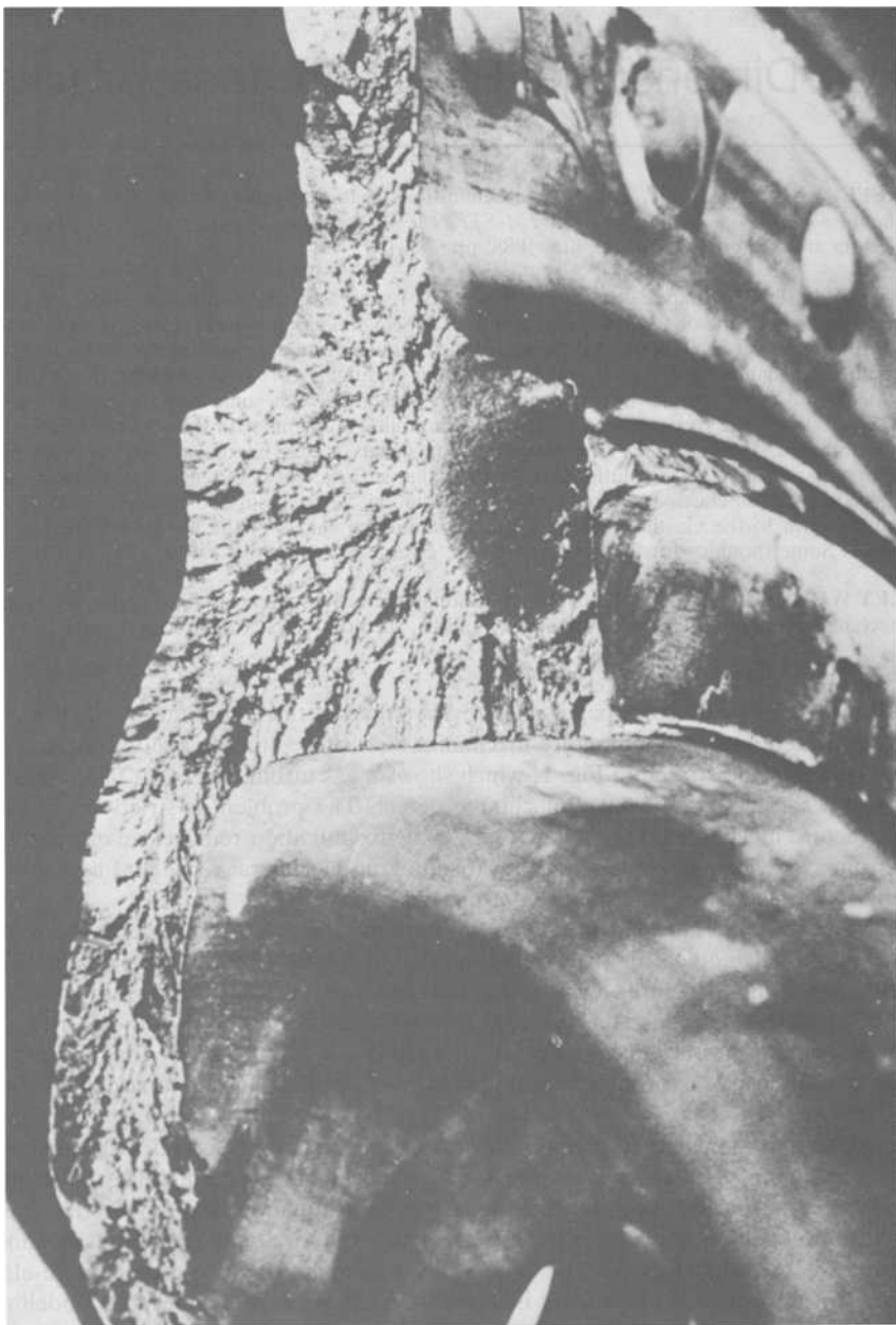
FIG. 1— Surface crack growing in a rotor part.
