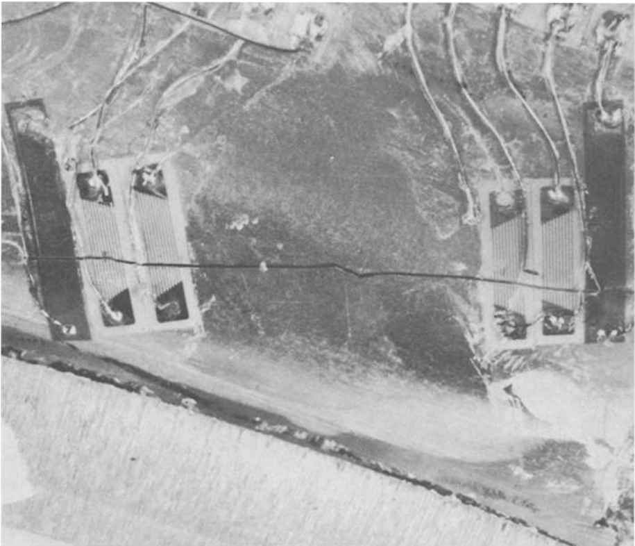
FIG. 6—Crack growth in a wheel flange with crack propagation and crack detection gages.
