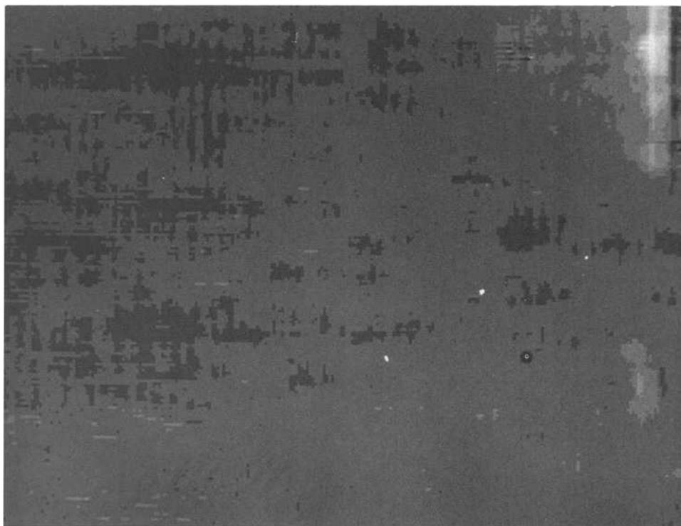
FIG. 2—Attenuation image of Gr(P55)/Al(6061) plate. The darkest level corresponds to 0 db/cm and the lightest level to 10.4 dB/cm. The sound propagation direction is perpendicular to the graphite fibers.
