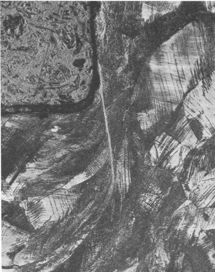
FIG. 13—*Light microscope picture of a typical adiabatic band formation in a Hadfield steel under dynamic blanking.*
