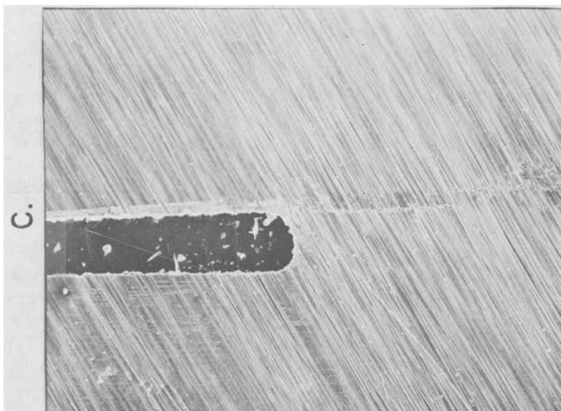
FIG. 2—(C) SEM photograph of broken fibers in 30^\circ ply at X30 ( 30^\circ ply of a [\pm 30/90]_s laminate).
