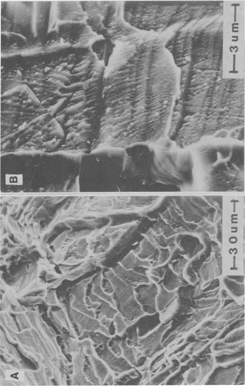
FIG. 5—SEM fractographs of SLC interface cracking. (A) Representative area. Note irregular arrest marks of “terraces.” (B) Fine serrations or shark’s skin texture on IFC facets.
