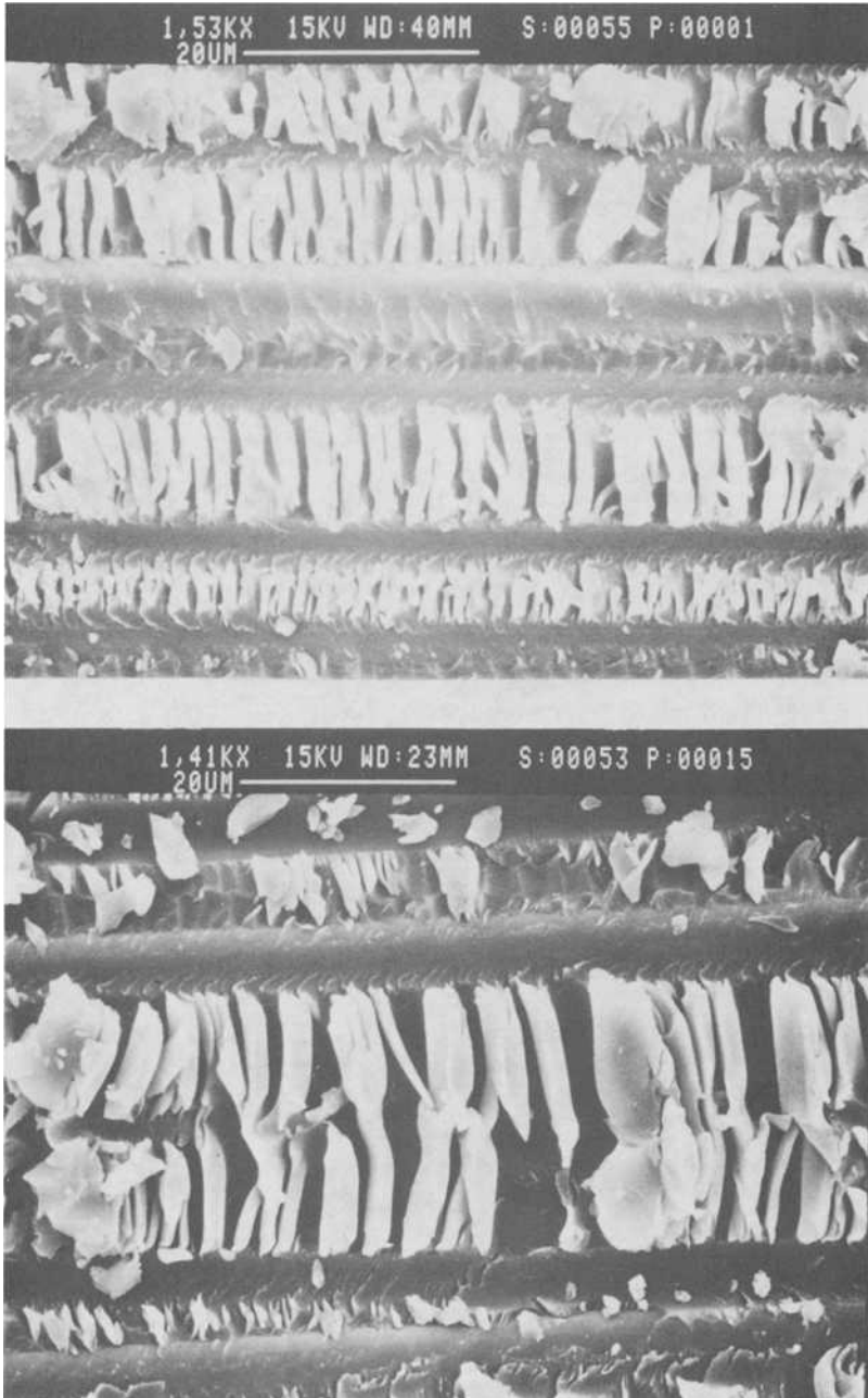
FIG. 12—Mode II fracture in unidirectional AS4/3501-6 graphite/epoxy (crack propagation direction from right to left; shear direction from left to right).
