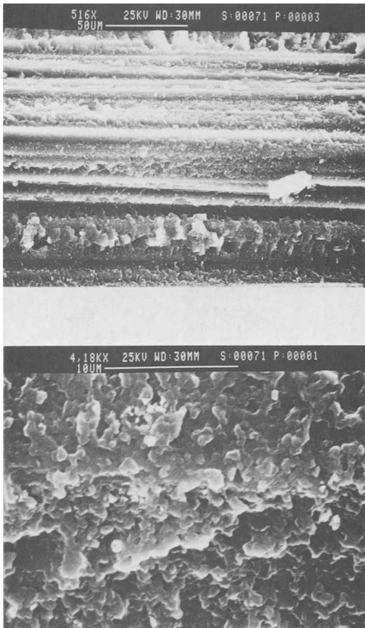
FIG. 19—Mixed Mode I and II fracture in unidirectional T300/F-185 graphite/epoxy ( K_I/K_{II} = 0.36 ) (crack and shear direction from right to left).
