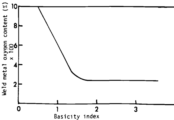
FIG. 2—General trend of the weld metal oxygen content as a function of flux basicity.
