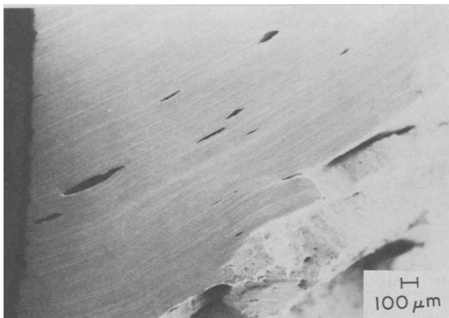
FIG. 11—Side of a Tenelon Charpy specimen, showing crack arrester orientation splitting ahead of the main crack front. Hydrogen charged and tested at 255 K.
