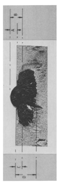
FIG. 1—Alternative crack depth interpretations.
