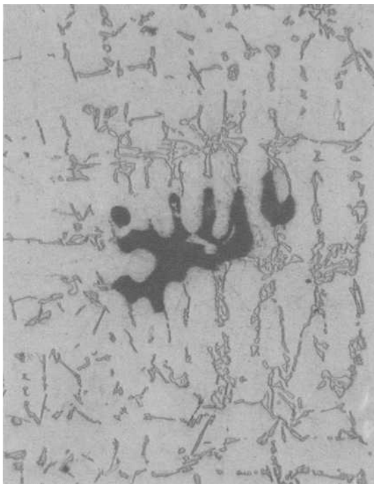
FIG. 10—Typical microstructure showing shrinkage porosity (X100).
