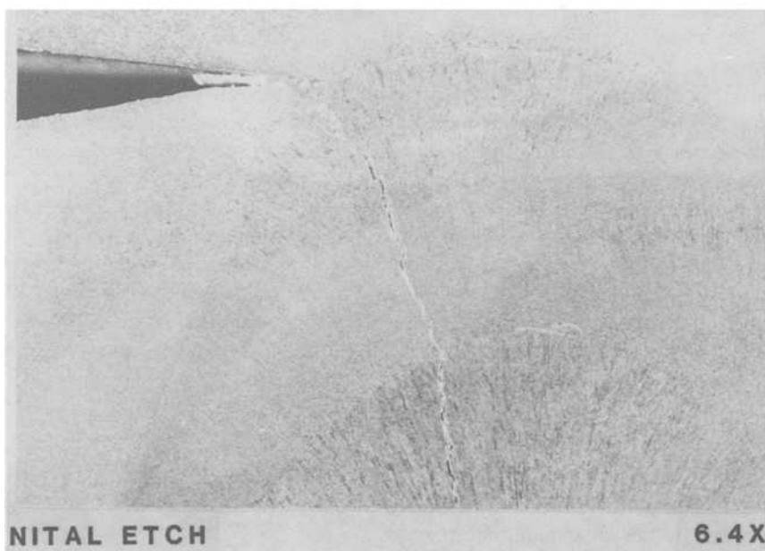
FIG. 4— Typical cracks found in weld joint.
