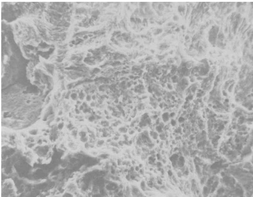
FIG. 7—Scanning electron fractograph taken at about 4 mm (0.16 in.) from the origin corner, showing intergranular cracking, ductile tearing, and some residual oxide ( \times 2000 ).
