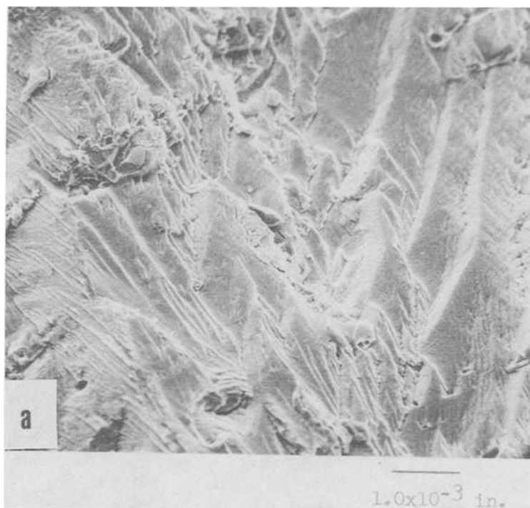
FIG. 12—(a) Typical fracture appearance near the point of crack initiation in a laboratory specimen tested under a low alternating stress and a near zero minimum tensile stress ( R = 0.05 ). In (b) fine fatigue markings are visible.
