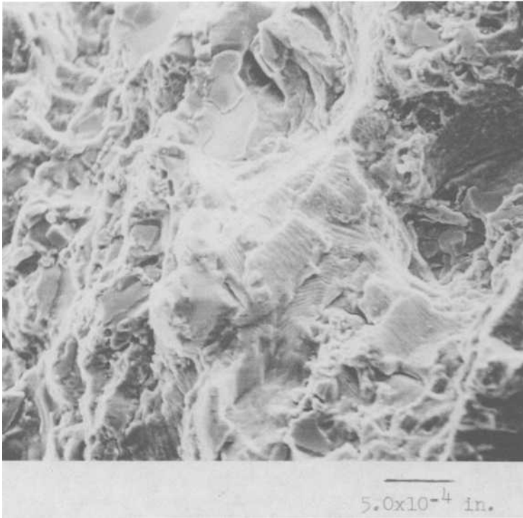
FIG. 16—SEM fractograph of a laboratory specimen tested at a high alternating stress intensity [ >22 \text{ MPa} \cdot \text{m}^{1/2} ( 20 \text{ ksi} \cdot \text{in.}^{1/2} )]. The fracture is similar to overload failure except it contains many areas which exhibit distinct fatigue striations.
