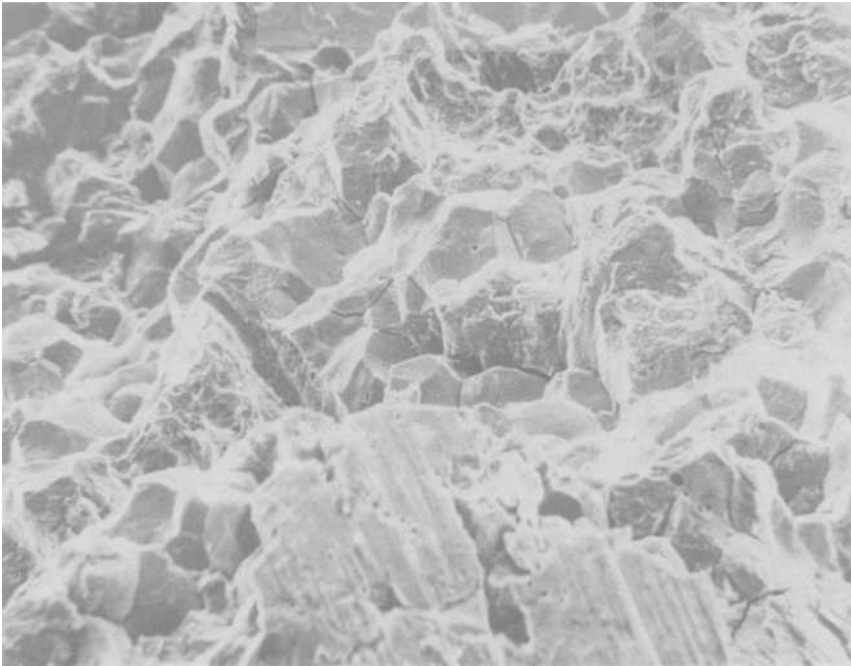
FIG. 6—Scanning electron fractograph at 3 mm (0.12 in.) from the rabbet corner. Intergranular and secondary cracking are evident, along with some residual oxide and ductile tearing ( \times 500 ).
