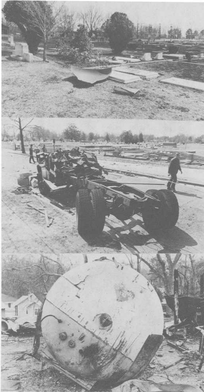
FIG. 1—Close view of the separated dome portion of tank (upper); View showing truck remains (middle); and view showing remaining tank portion (lower).
