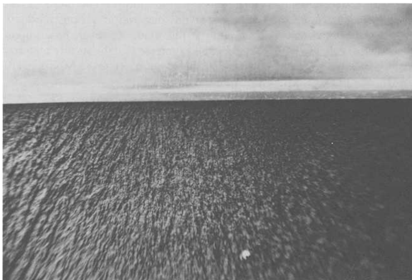
FIG. 5—Failure initiation site in lower die.
