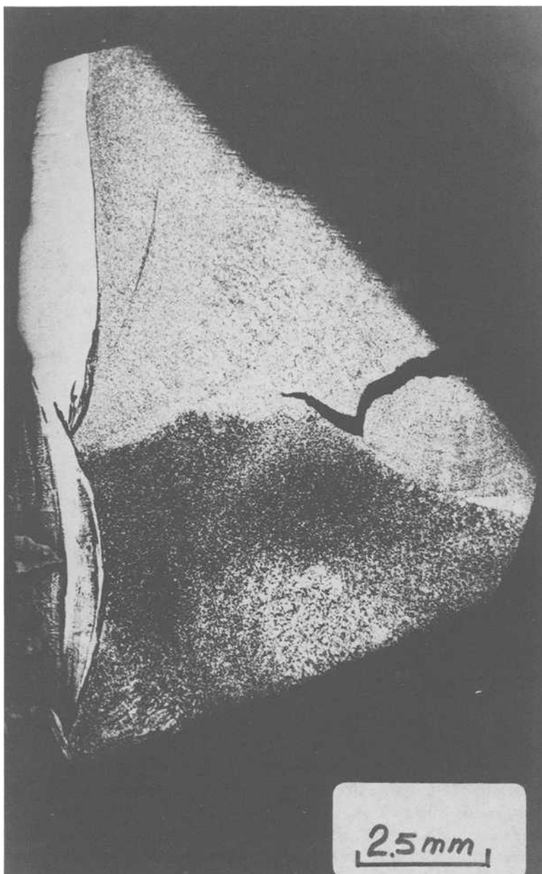
FIG. 7a—Macrosection of specimen removed from the inside surface adjacent to indication A4. Cracking is confined to weld metal. Cladding is displayed.
