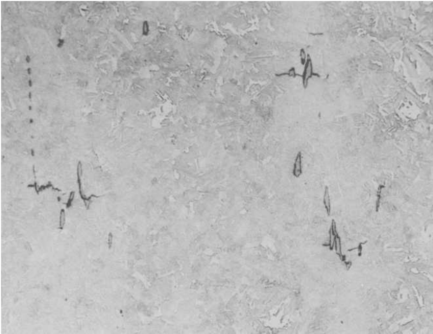
FIG. 3—Metallographic section near main fracture, showing segregation, MnS inclusions, and some microcracks at inclusions ( \times 150 ).
