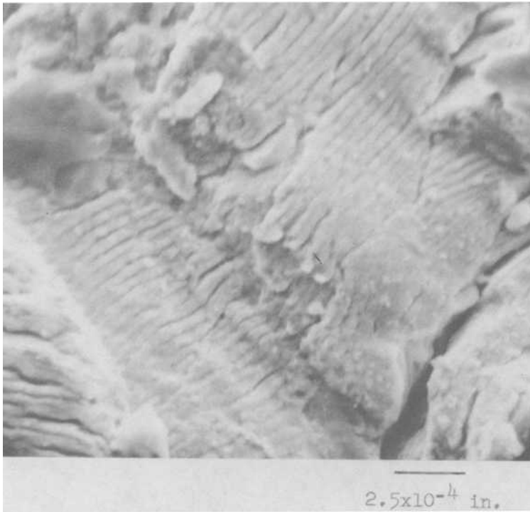
FIG. 15—Typical fatigue striations observed in a laboratory specimen tested at an alternating stress intensity between 11 and 22 \text{ MPa} \cdot \text{m}^{1/2} ( 10 and 20 \text{ ksi} \cdot \text{in.}^{1/2} ).
