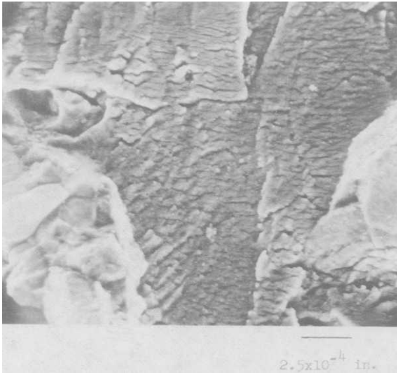
FIG. 7—SEM fractograph taken approximately 4.4 mm (0.175 in.) from the initiation site, showing a highly worked surface with cracks of different orientations, and no distinct fatigue striations.
