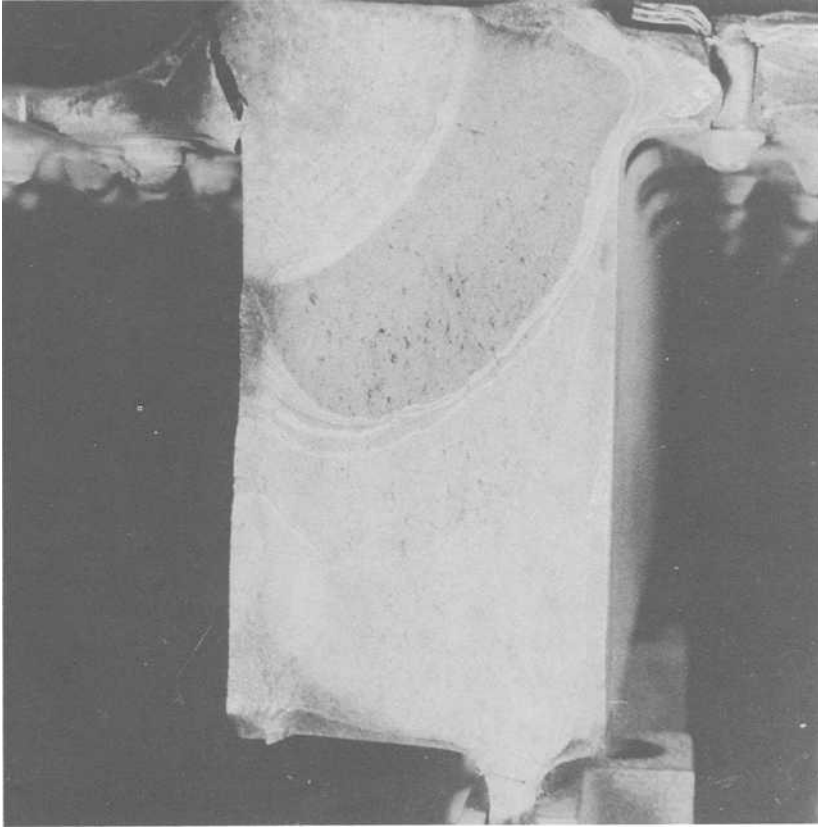
FIG. 5a—Details of the fatigue fracture of the top chord.
