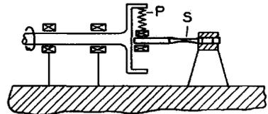
(e) Stationary Cantilever Specimen with Rotating Load.
