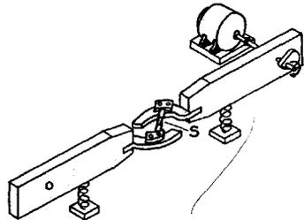
(e) Mechanical Oscillator Type of Combined Repeated-Bending and Reversed-Torsion Stress Machine.
