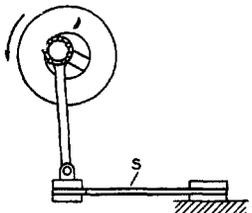
(a) Cantilever Specimen Actuated by a Crank or Cam.
