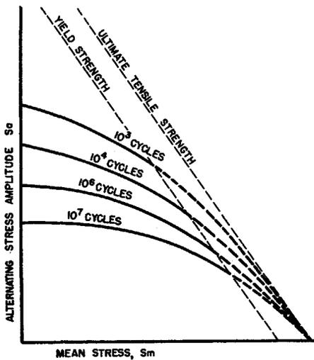
FIG. 27.—Haigh-Soderberg Method of Representing Failure Under Axial Loading at a Constant Number of Cycles.
