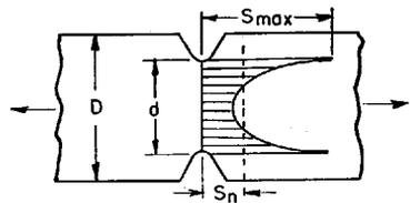
FIG. 16.—Notch Fatigue Specimens.
