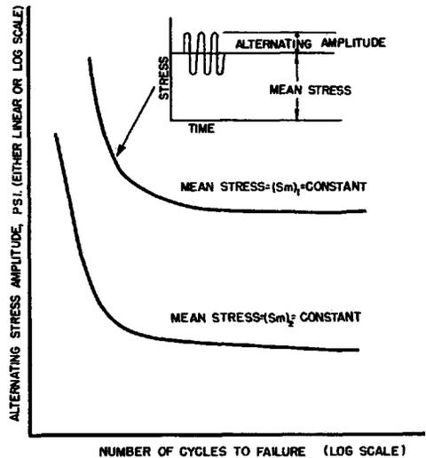
FIG. 23.—Representation of  $S-N$  Curves Taken at Constant Mean Stress.
