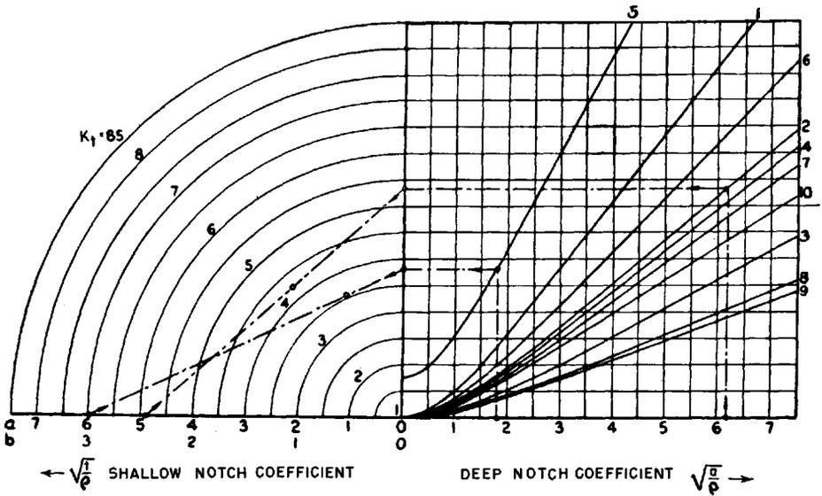
Fig. 20.—Nomograph for the Determination of the Ideal Stress-Concentration Factor.
