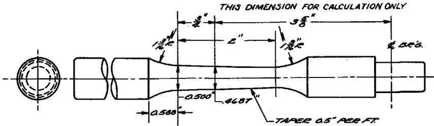
(a) Rotating-Beam Fatigue Specimen (McAdam Type).
