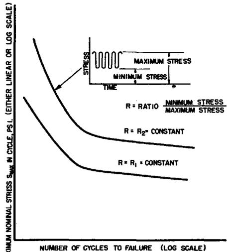
FIG. 24.—Representation of  $S$ - $N$  Curves Taken at Constant Stress Ratio.
