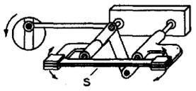
(b) Crank Type Machine Subjecting Specimen to Uniform Bending Moment.
