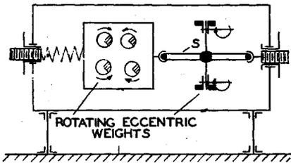
(a) Mechanical-Oscillator Type Machine for Applying Alternating Torsion and Pulsating Axial Loading—Schenck.
