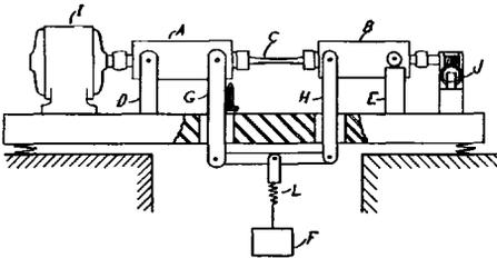
FIG. 18.—Pure-Bending Type Rotating-Beam Fatigue Machine.
