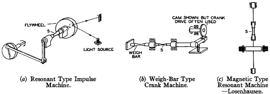
FIG. 7.—Torsion Fatigue Testing Machines.
