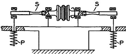
(b) Double-End Rotating Cantilever Machine.
