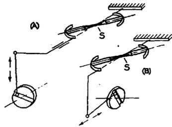
(d) Attachments to Conventional (A) Repeated-Bending and (B) Reversed-Torsion Machines to Obtain Combined Bending and Torsion Stress.
