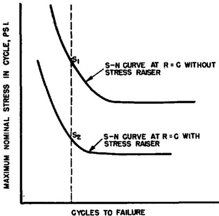
FIG. 30.—Use of Constant  $R$  Curves to Estimate Strength Reduction Factor.
