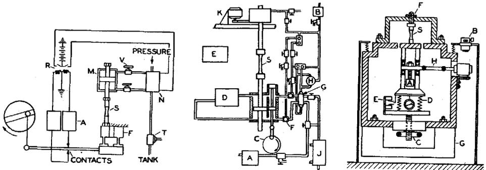
(a) Crank and Lever Operated Machine—Krouse.
