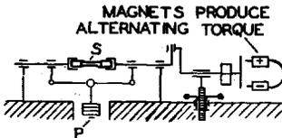
(b) Combined Rotating-Bending and Reversed-Torsion Stress Machine.
