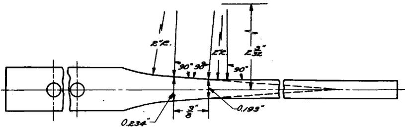
(c) Sheet Fatigue Specimen (Bell Telephone Co. Type).
