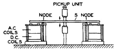
(g) Magnetic Type Resonant Machine—Rayflex.
