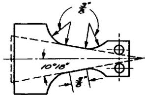
(b) Sheet Fatigue Specimen (Bureau of Standards Type). Sheets from 0.008 to 0.031 in. gage length increased for thicker sheets.
