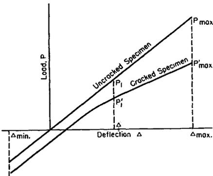
FIG. 19.—Load-Deflection Diagram for an Uncracked and a Cracked Specimen in Bending or Torsion.
