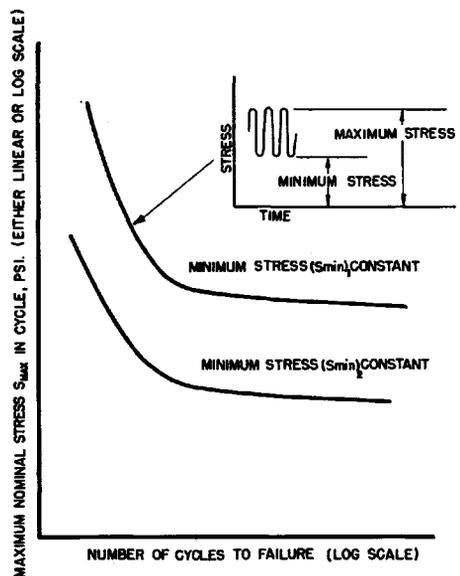
FIG. 25.—Representation of  $S$ - $N$  Curves Taken at Constant Minimum Stress.
