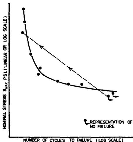
FIG. 22.—Representation of *S-N* Curve for Completely Reversed Stress.
