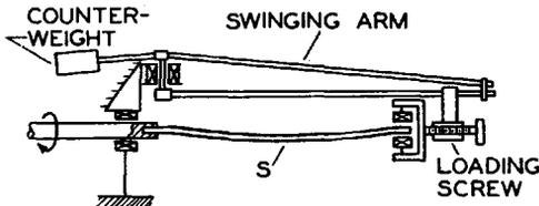
(d) Wire Tested as Euler Column. (Specimen deflection is in horizontal plane instead of vertical shown.)
