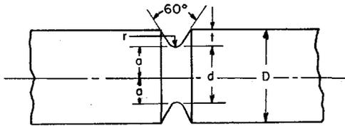
$$\begin{aligned} D &= 0.480 \text{ in.} \\ d &= 0.300 \text{ in.} \\ d/D &= 0.625 \end{aligned}$$
