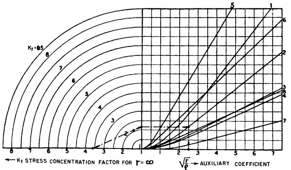
Fig. 21.—Supplementary Nomograph for Circumferential Notches, Provided with an Axial Hole
