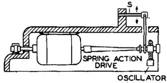
(h) Single-Weight Mechanical Oscillator Type Machine—Sonntag.
