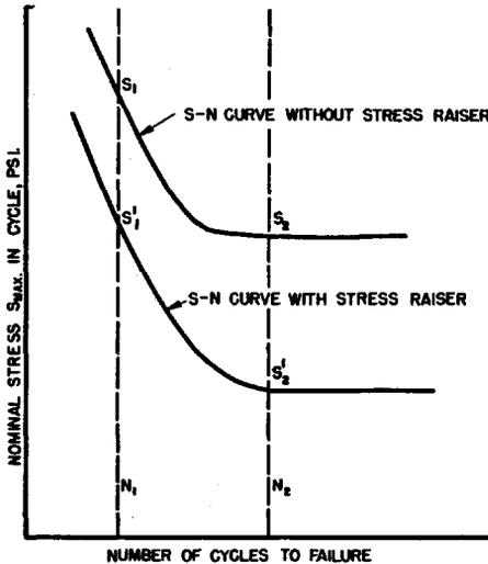
FIG. 28.—*S-N* Curves for Completely Reversed Stress Used to Estimate Strength Reduction Factor.
