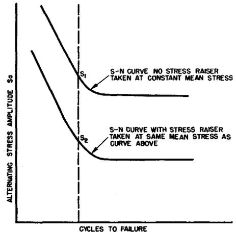
FIG. 29.—Constant Mean Curves Used to Estimate Strength Reduction Factor.
