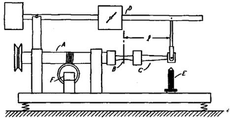
FIG. 17.—Cantilever Type Rotating-Beam Fatigue Machine.
