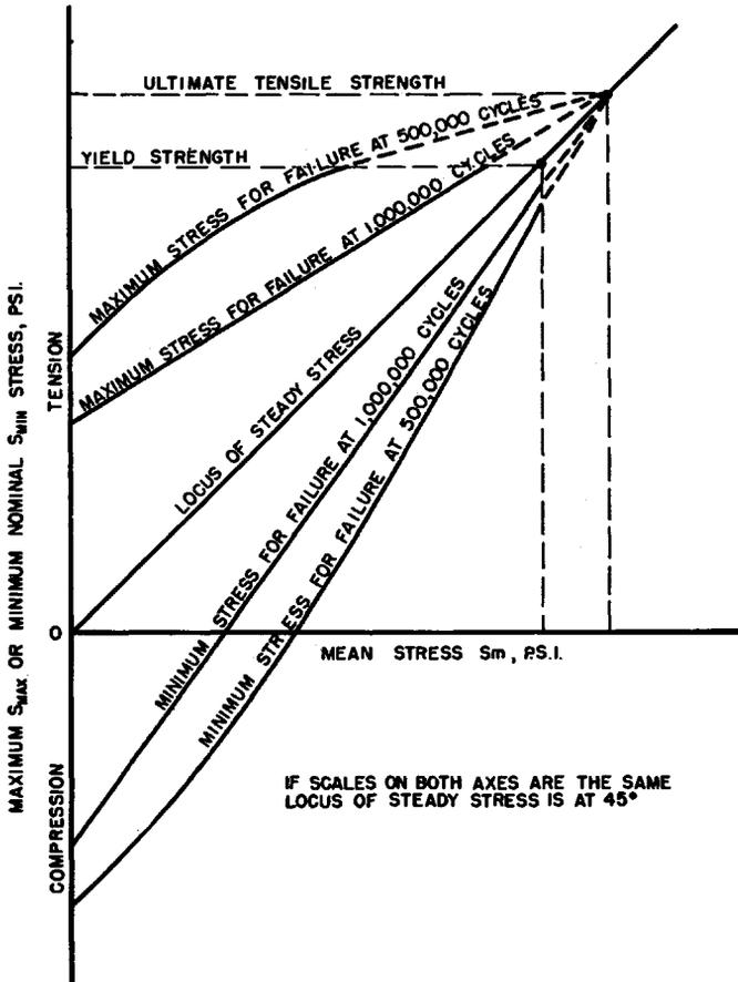
FIG. 26.—Diagram for Representation of Failure, Under Axial Loading, at Constant Number of Cycles.
