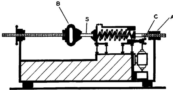
(a) Mechanical-Oscillator Type Resonant Machine—Schenck.
