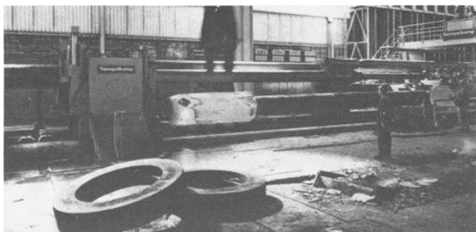
FIG. 16—A 15-MN (1500 metric ton) horizontal push bench for forged tubes. (Courtesy of Schirmer-Plate-Siempelkamp Hydraulic Presses.)
