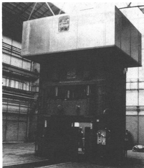
FIG. 6—A 50-MN (5000 metric ton) isothermal/hot die forging press. (Courtesy of Schirmer-Plate-Siempelkamp Hydraulic Presses.)
