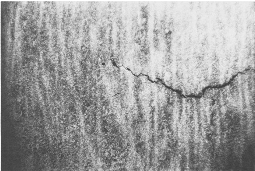
FIG. 19— Polished and etched transverse section of flake shown in Fig. 18, X12 (reduced one third for reproduction).
