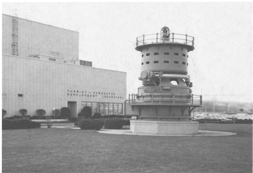
FIG. 1—5000-kW vertical Curtis steam turbine-generator at the Schenectady plant of the General Electric Co. (designated as a national historic mechanical engineering landmark by the American Society of Mechanical Engineers, 28 May 1975).
