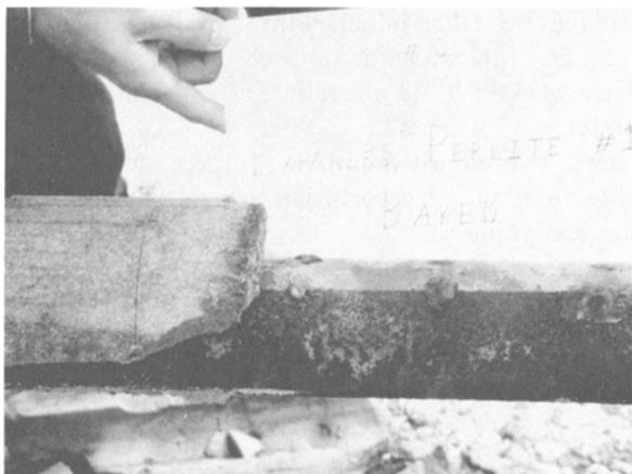
FIG. 7—The pipe and baked expanded Perlite insulation at the end of the test.
