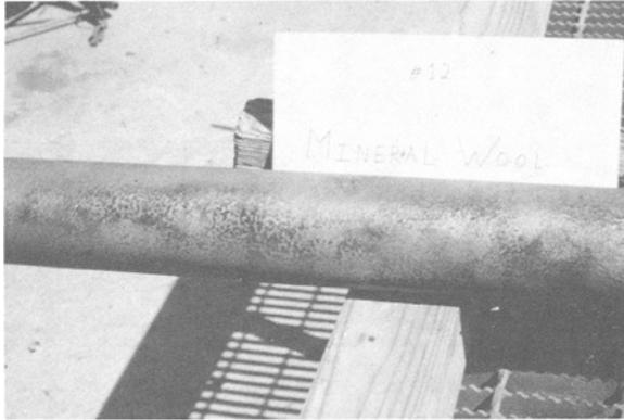
FIG. 8—Part of the pipe after the test and cleanup. Ultrasonic thickness measurements were taken at this time.
