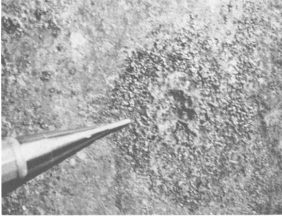
FIG. 10—*Minor pitting of carbon steel.*
