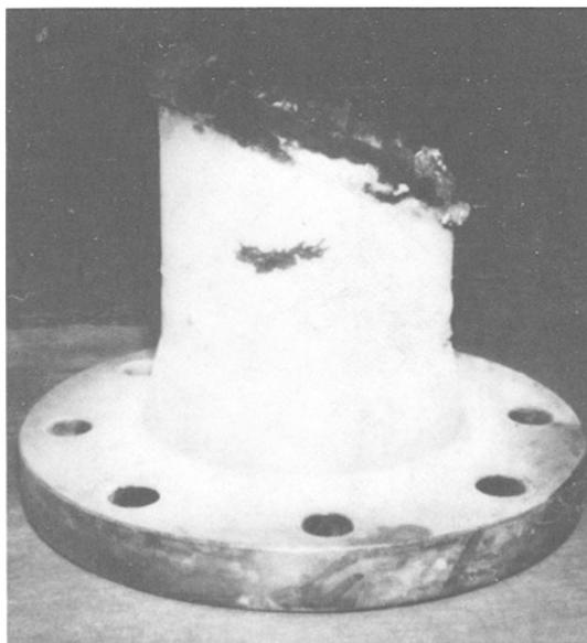
FIG. 3—*Liquid penetrant inspection, 10.2-cm (4-in.) nozzle.*
