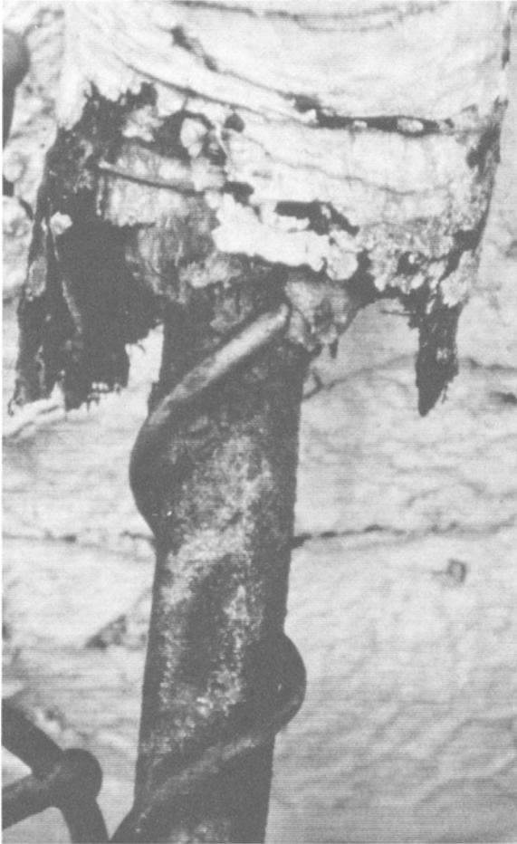
FIG. 6—A steam traced line showing severe corrosion under the tracing tubing. Galvanic corrosion may be a factor between copper tubing and steel pipe, when water frequently enters the system.
