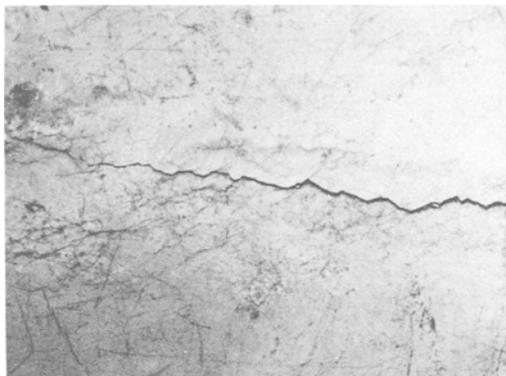
FIG. 2—Another example of ESCC. Here the sample had been bent to open up the main crack.
