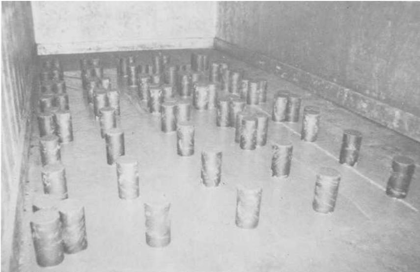
FIG. 1—Concrete specimens in the initial curing period at 4°C (39°F).
