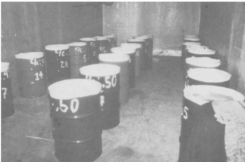
FIG. 2—Curing of the concrete specimens in reconstituted seawater kept at 0°C (32°F).
