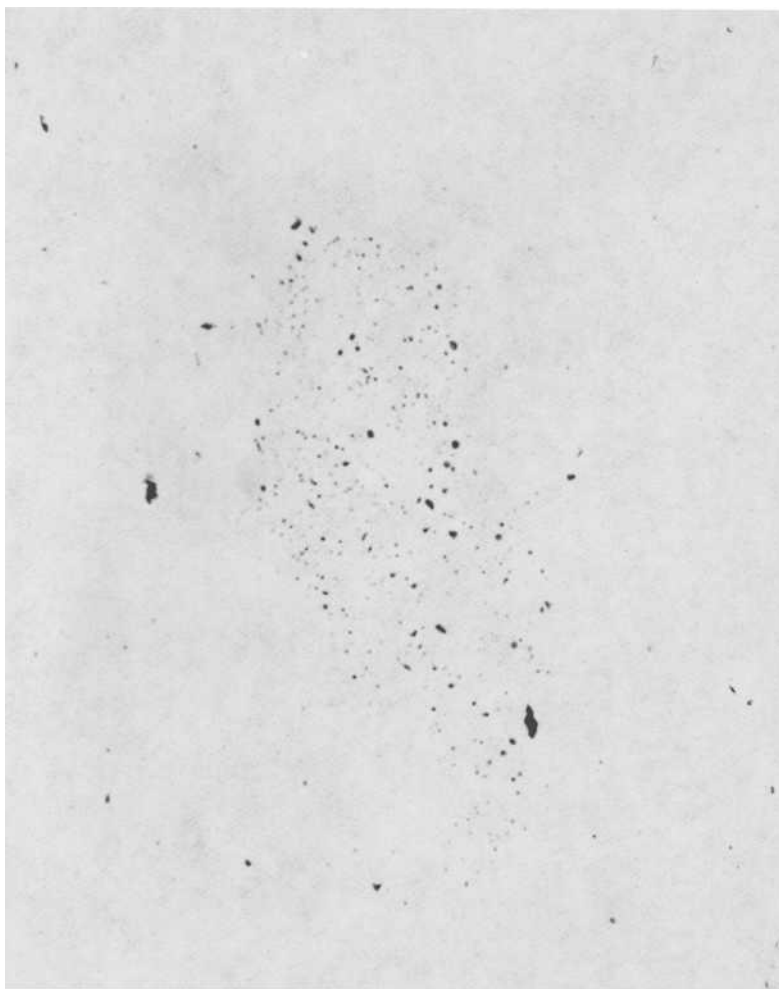
FIG. 2—“Spotty particle” oxide inclusion, magnification \times 800 .
