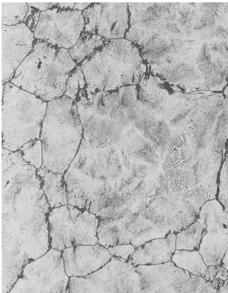
FIG. 4—Continued: (c) photomicrograph of the specimen in Fig. 4, Part a, after electrolytic etching with alkaline sodium picrate, 6 V dc, 0.15 \text{ A/cm}^2 , for 1 min.
