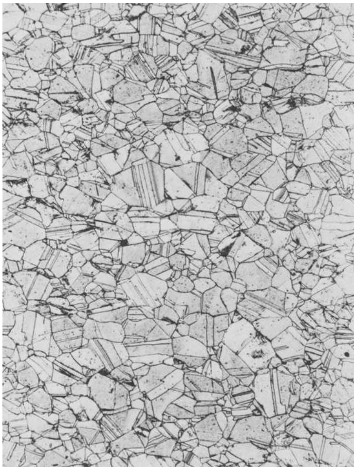
FIG. 1—Photomicrograph of an austenitic alloy, alpha brass, containing annealing twins, etched with Klemm's I reagent (saturated aqueous sodium thiosulfate plus 2% potassium metabisulfite), at \times 100 magnification.
