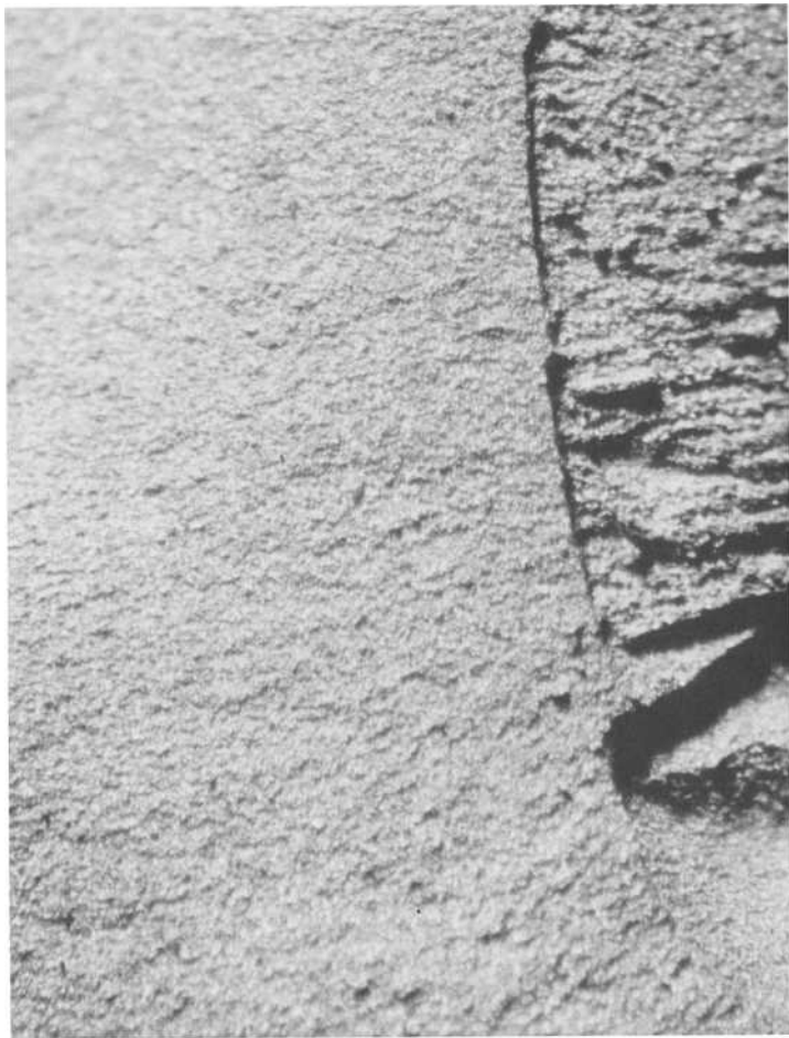
FIG. 1—Fracture surfaces of commercial grades of WC-Co at \times 40 : (top) 6% cobalt by weight, (bottom) 16% cobalt by weight.
