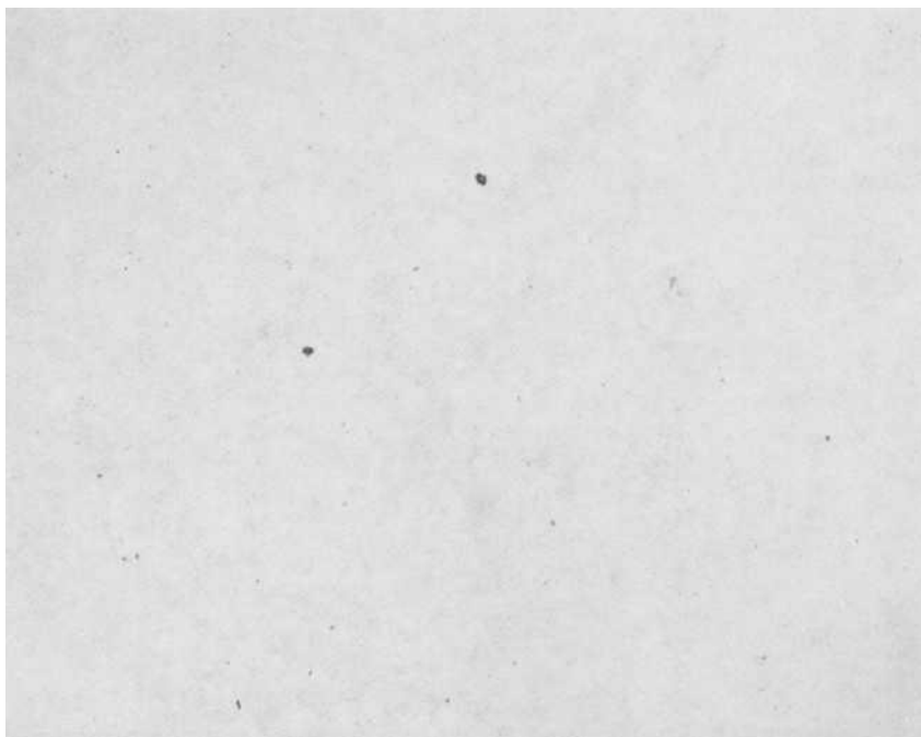
FIG. 2—Typical porosity of commercial grade WC-Co, unetched surface, \times 200 .
