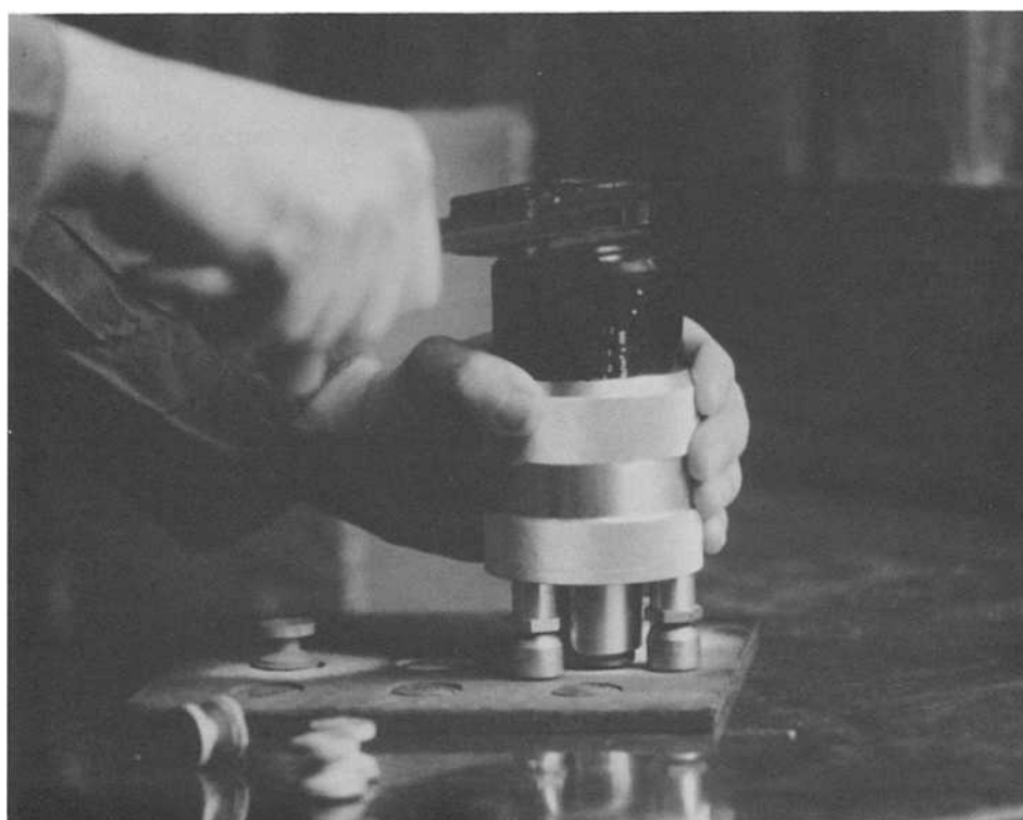
FIG. 5-6—Elcometer adhesion test. This test uses small aluminum dollies which are adhered to the lining surface and pulled off in direct tension. It is useful since portable equipment is available to perform tests under field conditions. (Photograph courtesy of Ceilcote Company, unit of General Signal.)
