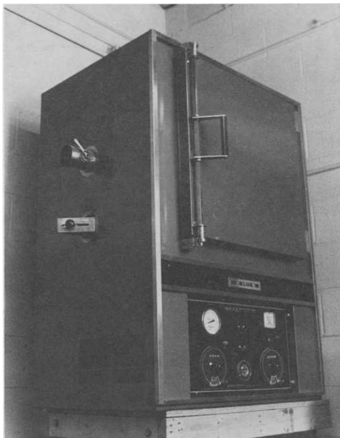
FIG. 5-1—Oven/muffle furnace for laboratory evaluation of FGD lining materials. High-temperature ovens can be used to evaluate thermal effects on lining materials. (Photograph courtesy of Ceilcote Company, unit of General Signal.)
