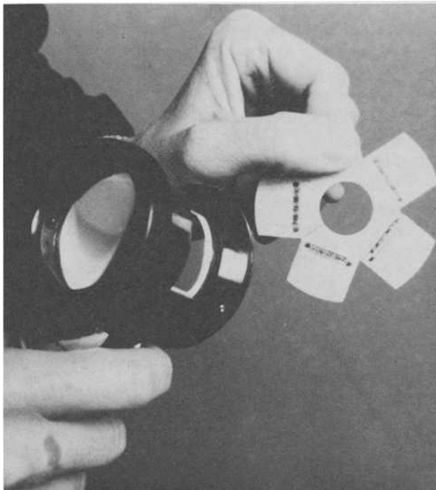
FIG. 7-12—Keane-Tator surface comparator. A field test determines the depth of profile of a sandblast pattern. (Photograph courtesy of Ceilcote Company, unit of General Signal.)
