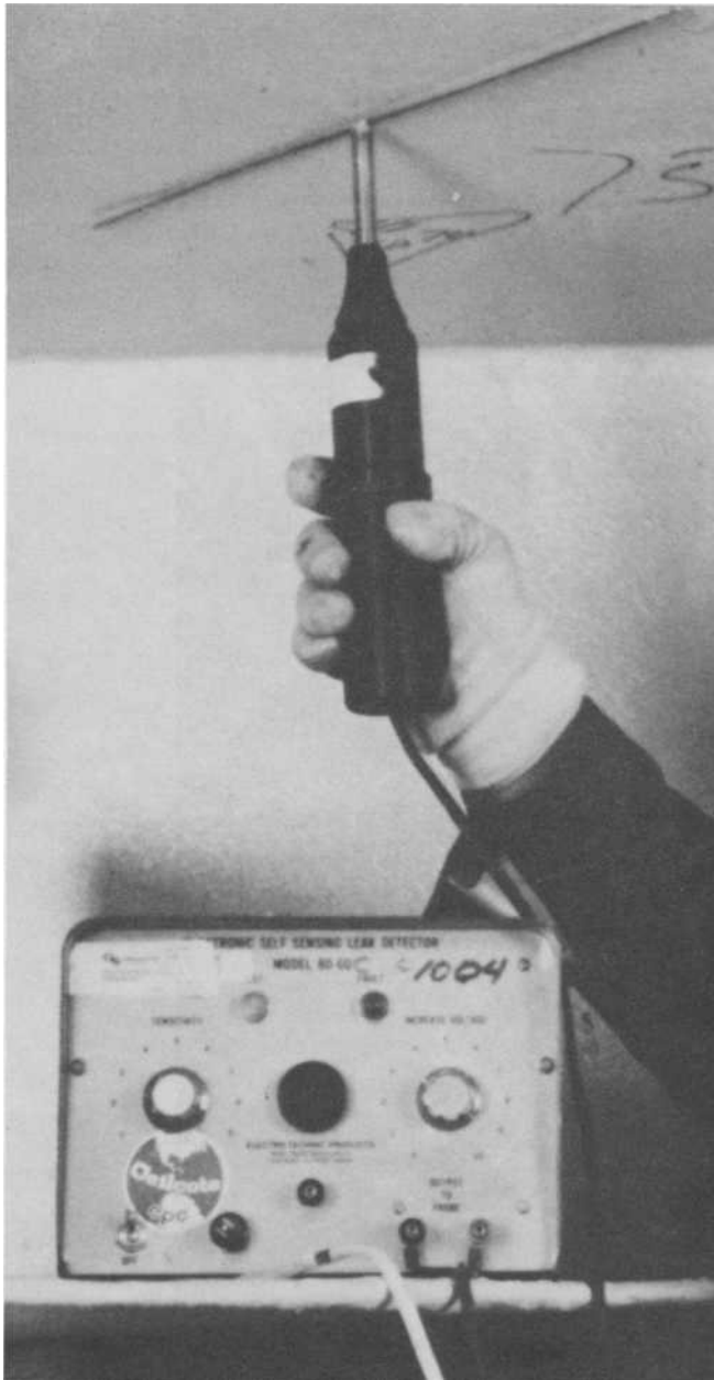
FIG. 7-9 (left) and FIG. 7-10 (right)—Spark testing of organic linings with up to 20 000 V to ensure that the lining is pinhole free. (Photographs courtesy of Ceilcote Company, unit of General Signal, and Tinker and Rasor, respectively.)
