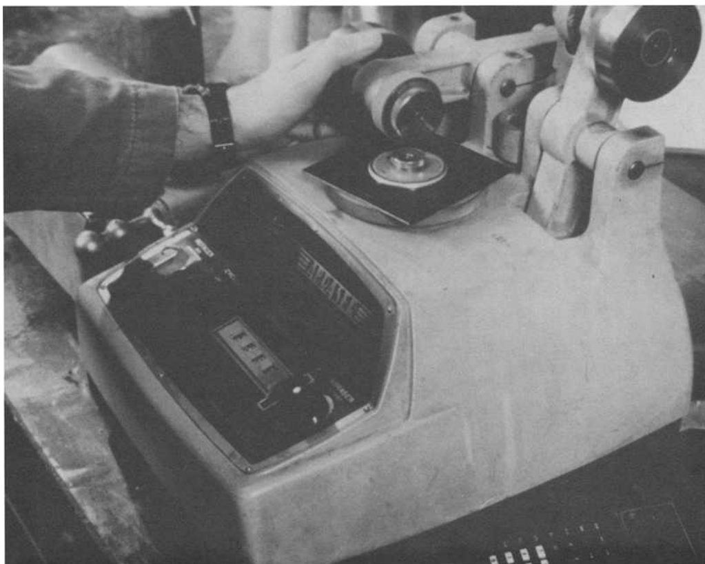
FIG. 5-5—Abrasion testing using the Taber abraser. This test measures wear of a lining or coating surface under a rolling contact with selected abrasive wheels. It does not correlate particularly well with abrasive liquid or gaseous environments. (Photograph courtesy of Ceilcote Company, unit of General Signal.)
