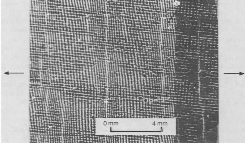
FIG. 1—Moiré fringe pattern of a  $[0,90_3]$  E-glass laminate between cracked sections in the 90-deg plies.
