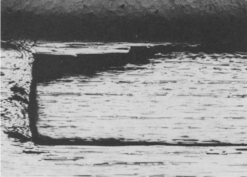
FIG. 7—Photomicrograph of 50-ply, AS-1/AF-R-E350 short-beam shear specimen.
