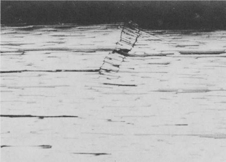
FIG. 6—Photomicrograph of 16-ply, AS-1/AF-R-E350 short-beam shear specimen.
