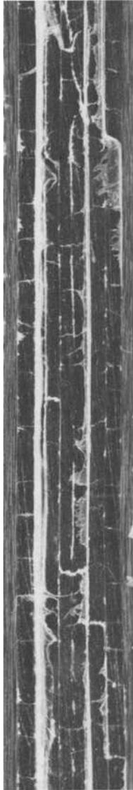
FIG. 15—Edge replica from a  $[0,90,\pm 45]$ , laminate at Stage II.
