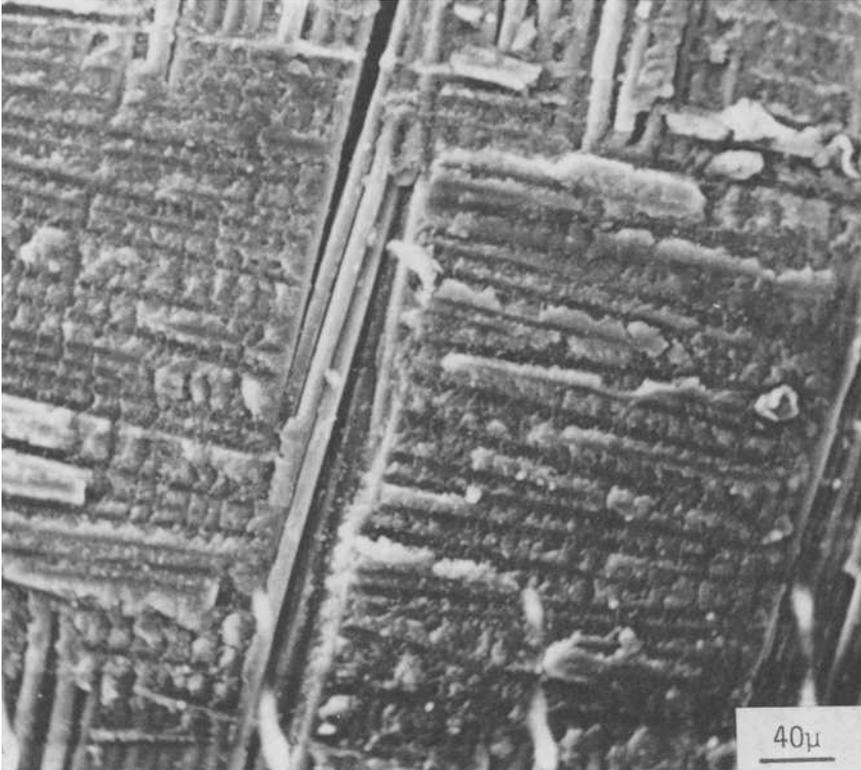
FIG. 24—Bridging of fibers by passage of a longitudinal crack.
