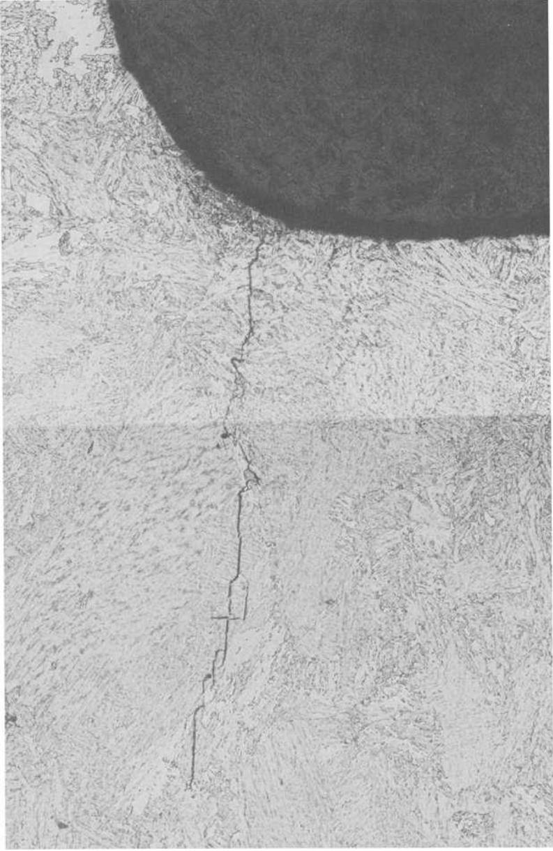
FIG. 6—Section through a subcritical crack. Etchant: Nital.
