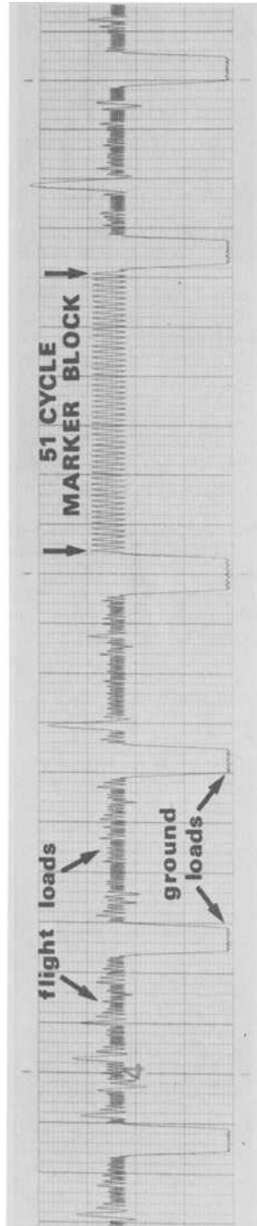
FIG. 16—Tracker load spectrum with marker block.
