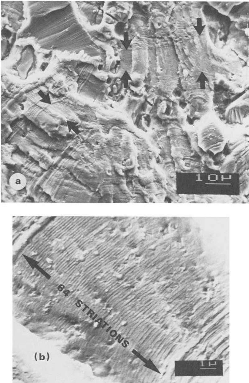
FIG. 8—(a) First observed marker band of Snowbird spectrum (2.6 mm from crack initiation site). (b) Marker band width = 10.3\text{ }\mu\text{m} ; average striation spacing = 0.16\text{ }\mu\text{m} .
