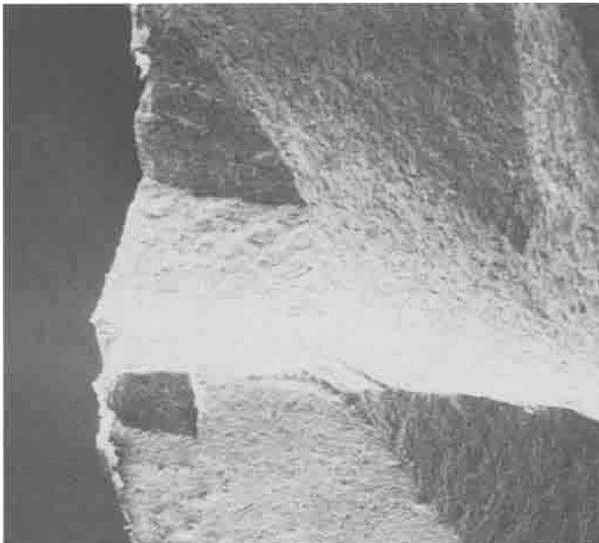
FIG. 2— SEM photomicrograph of corner chip ( \times 50 ).
