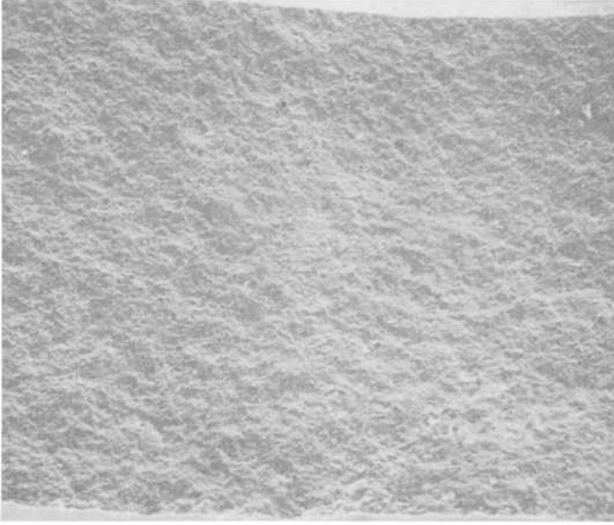
FIG. 14— SEM photomicrograph of fracture surface of tinning failure ( \times 50 ).
