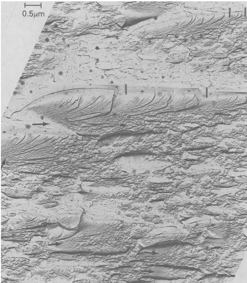
FIG. 15—Mist and hackle on glass fracture. Crack propagation left to right. Note fracture stress showing local crack fanning out in association with hackle formation (at arrows) and diminishing height of hackle (near vertical marks) associated with distinct turning of fracture steps across the hackle ridges. (Photo courtesy E. Beauchamp, Sandia National Laboratories.)
