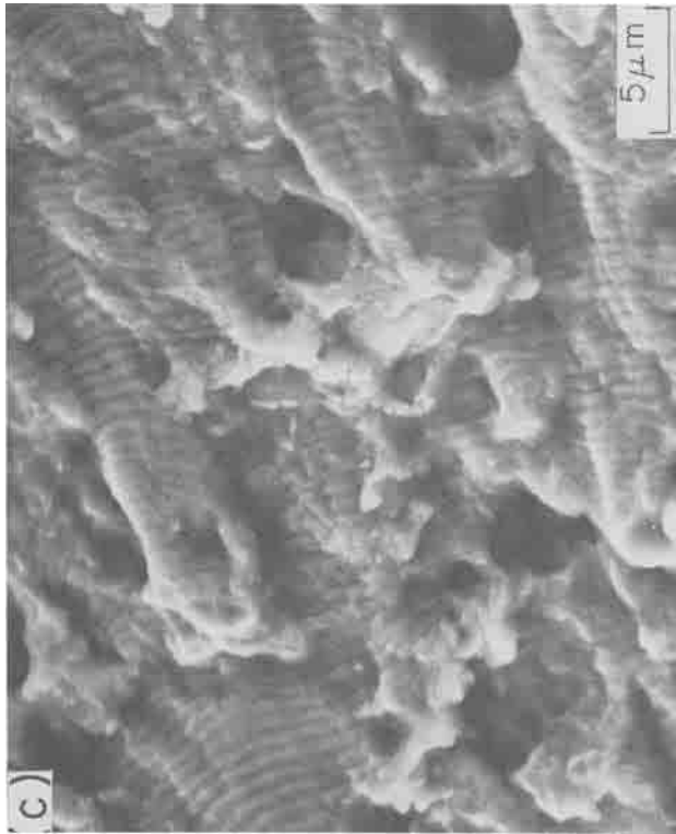
FIG. 5—Variation of fatigue striations with grain size in specimens without hydrogen. (a) 20\text{ }\mu\text{m} grain size ( \Delta K \approx 19\text{ MPa}\sqrt{\text{m}} ). (b) 100\text{ }\mu\text{m} grain size ( \Delta K \approx 29\text{ MPa}\sqrt{\text{m}} ). (c) 200\text{ }\mu\text{m} grain size ( \Delta K \approx 29\text{ MPa}\sqrt{\text{m}} ).
