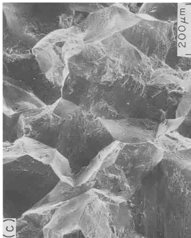
FIG. 7—Variation of intergranular fracture in cathodically charged specimens (200 \mu\text{m} grain size) with stress intensity. (a) \Delta K \approx 5.5 \text{ MPa}\sqrt{\text{m}} . (b) \Delta K \approx 14 \text{ MPa}\sqrt{\text{m}} . (c) \Delta K \approx 24 \text{ MPa}\sqrt{\text{m}} .
