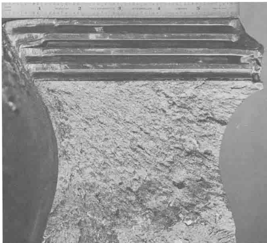
FIG. 3—Fracture surface at base of blade attachment groove. Inlet side is at left.
