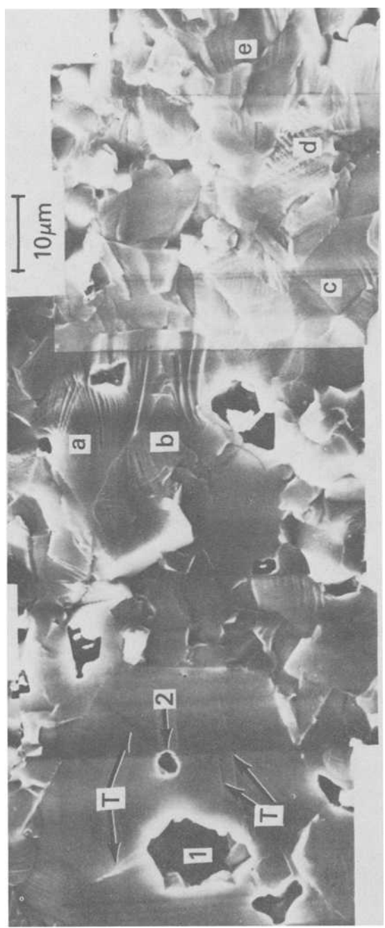
FIG. 46—Fracture surface of a high-strength \text{Al}_2\text{O}_3 specimen tested at -196^\circ\text{C} . Fracture at 651\text{ MPa} ( 94.5 \times 10^3\text{ psi} ) originated from the large pore within the large grain near the left-hand edge of the photo, about 60\text{ }\mu\text{m} in from the tensile surface. Note the relatively smooth flat fracture through and somewhat beyond the large grain, except for the fracture tails (T) associated with both the main (1) and a secondary (2) pore. Beyond this smoother area the fracture becomes rougher and begins to involve some intergranular failure as well as a number of features which appear to be similar to cathedral-type mirrors, or portions thereof, seen on single-crystal \text{Al}_2\text{O}_3 fracture (a to e). The orientation of these apparent cathedral mirrors as well as other fracture features indicate that the local direction of crack propagation was significantly different from a simple smooth semicircular flaw spreading out from the origin. (Photo courtesy Dr. H. Kirchner, Ceramic Finishing Company.)
