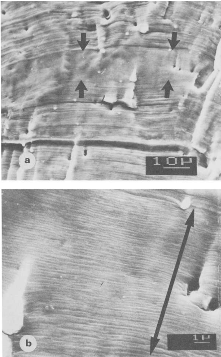
FIG. 13—(a) Marker band 2; Surface A1, Rivet 1 (0.63 mm from crack initiation site). (b) Marker band width = 9.2\text{ }\mu\text{m} ; average striation spacing = 0.14\text{ }\mu\text{m} .
