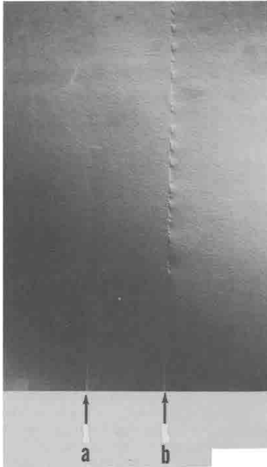
FIG. 5—Optical photomicrograph of fracture surface showing detail resulting from (a) momentary crack arrest and (b) 16-h aging period. Fracture direction from left to right; Nomarski differential contrast optics (after Michalske [4]).
