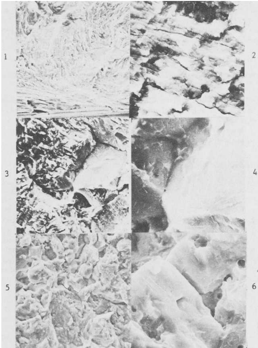
FIGS. 1 to 6—(1) Notched 35NCD16; N_f = 2850 ; 0 to 1587 MPa stress; ridges at varied angles to notched surface ( \times 1300 ). (2) Same as Fig. 1; truncated but possibly damaged striations ( \times 13\ 000 ). (3) Notched 35NCD16; N_f = 10\ 055 ; 0 to 966 MPa stress; isolated zone of intergranular fracture ( \times 1000 ). (4) Same as Fig. 3; features suggestive of quasi-cleavage on prior austenite grain boundaries ( \times 4000 ). (5) Notched 4340; 2139-MPa UTS; N_f = 1130 ; 0 to 1145 MPa stress; zone of transition from transgranular to intergranular fracture ( \times 1350 ). (6) Unnotched 4340; 2139-MPa UTS; N_f = 3950 ; 0 to 1415 MPa stress; quasi-cleavage and intergranular fracture ( \times 6300 ). The direction of crack propagation in each photomicrograph is from bottom to top.
