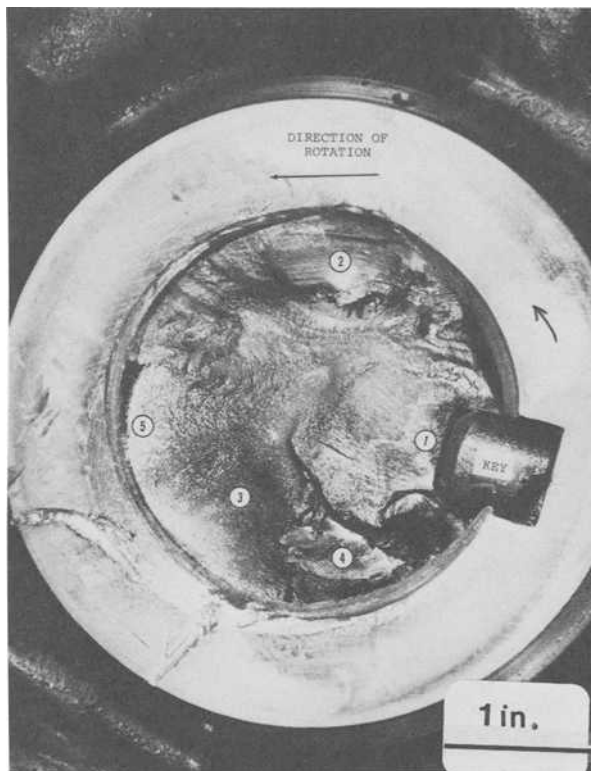
FIG. 3—Appearance of the governor side fracture surface. Areas 1 to 5 were damaged.
