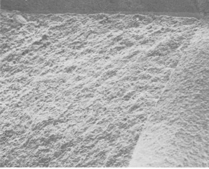
FIG. 11— SEM photomicrograph at fracture origin of pinning failure ( \times 100 ).
