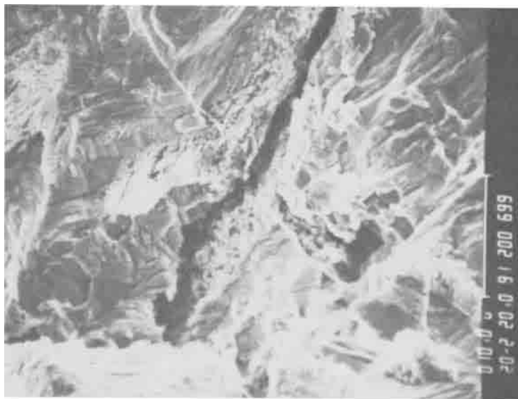
FIG. 14—Microscopic fracture surface of spiral-longitudinal cracks.
