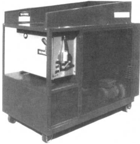
FIG. 2—Typical application machine for spray-applied mineral fiber.
