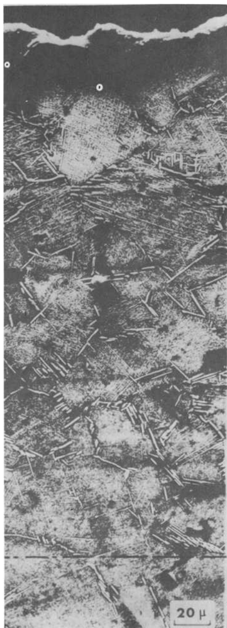
FIG. 10—Optical micrograph showing plastic zone in In 718 as delineated by \delta -phase [50].
