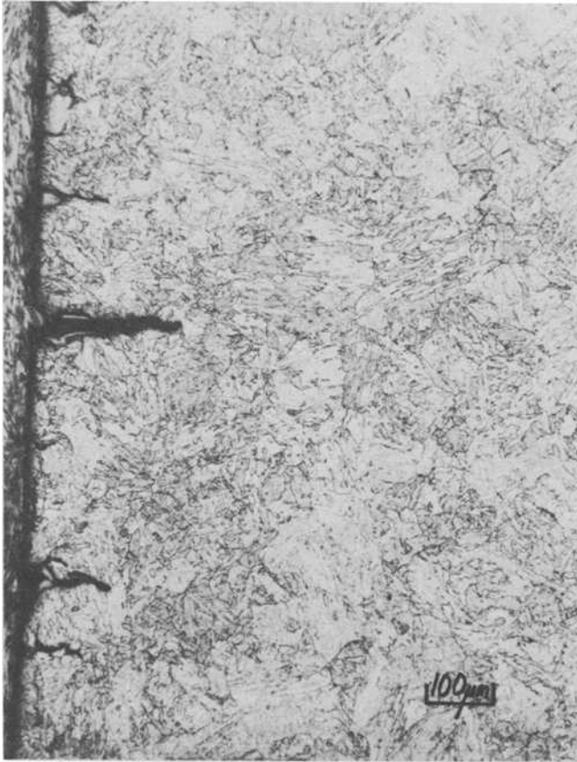
FIG. 6—Section of specimen cycled with 29-min hold in tension; \Delta\epsilon = \pm 0.7\% for 349 cycles.
