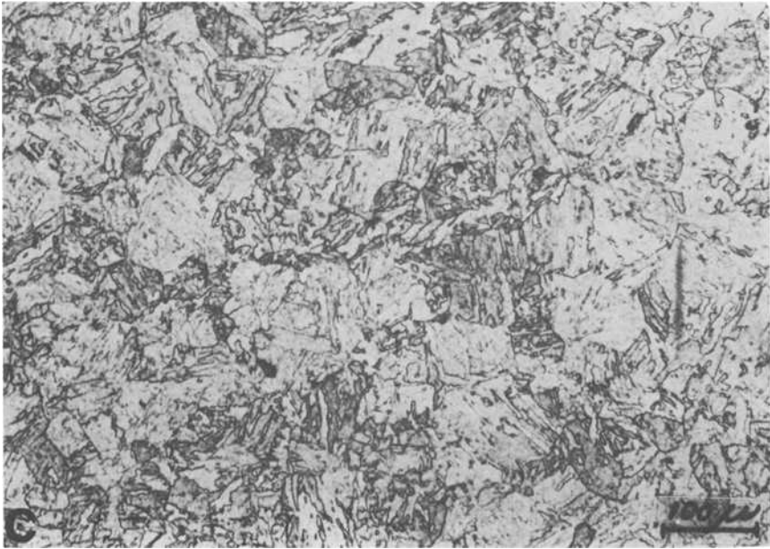
FIG. 13c—Optical micrograph of material cycled with holds for 349 cycles.
