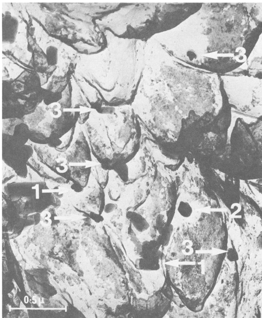
FIG. 10—Transmission electron fractograph of an A533B extraction replica showing small shear dimples containing submicron precipitates identified as (1) Mo 2 C; (2) AlN; and (3) AlN/Mo 2 C aggregate.
