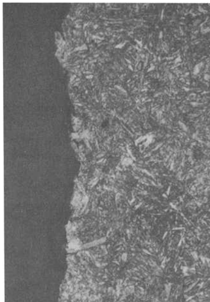
After One Shot Peening/Plating Cycle
