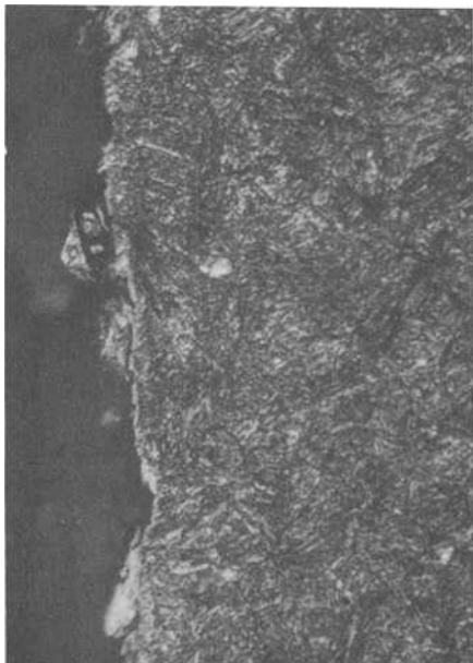
After Five Shot Peening/Plating Cycles
