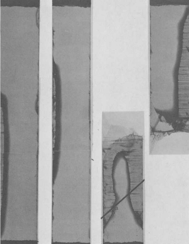
FIG. 7—DIB X-radiograph of  $(25/-25/\overline{90})_n$ . Specimens 11-2, 11-3, and 11-4 (left to right) after  $\epsilon_x = 0.63$  percent. Oblique cut made for microscopic examination of delamination Regions a and b is shown.
