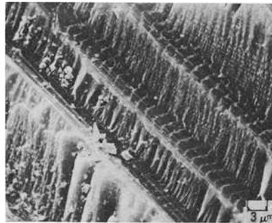
b) Epoxy Striations Propagating From the Top of One Fiber to the Base of the Adjacent Fiber
