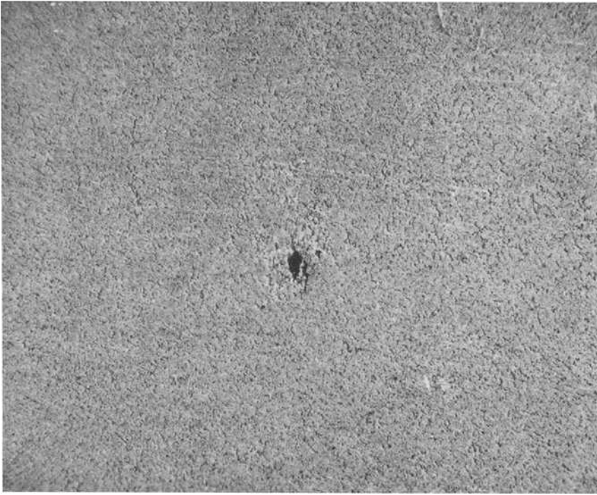
FIG. 8—Failure origin associated with segregation ( \times 20 ).
