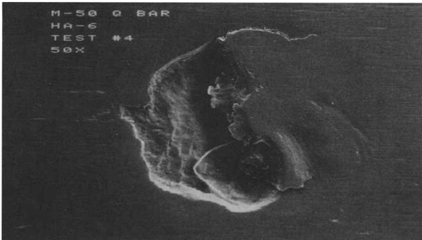
FIG. 8—Typical fatigue spall in M-50.
