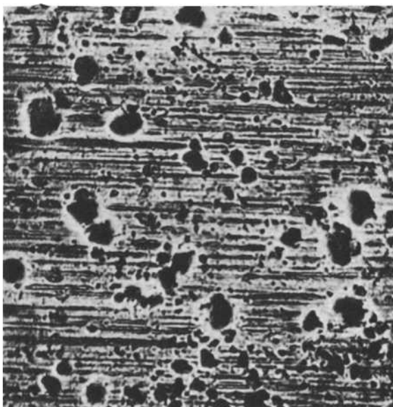
FIG. 9—Debris indentation damage created under 40- \mu m filtration conditions ( \times 100 ).
