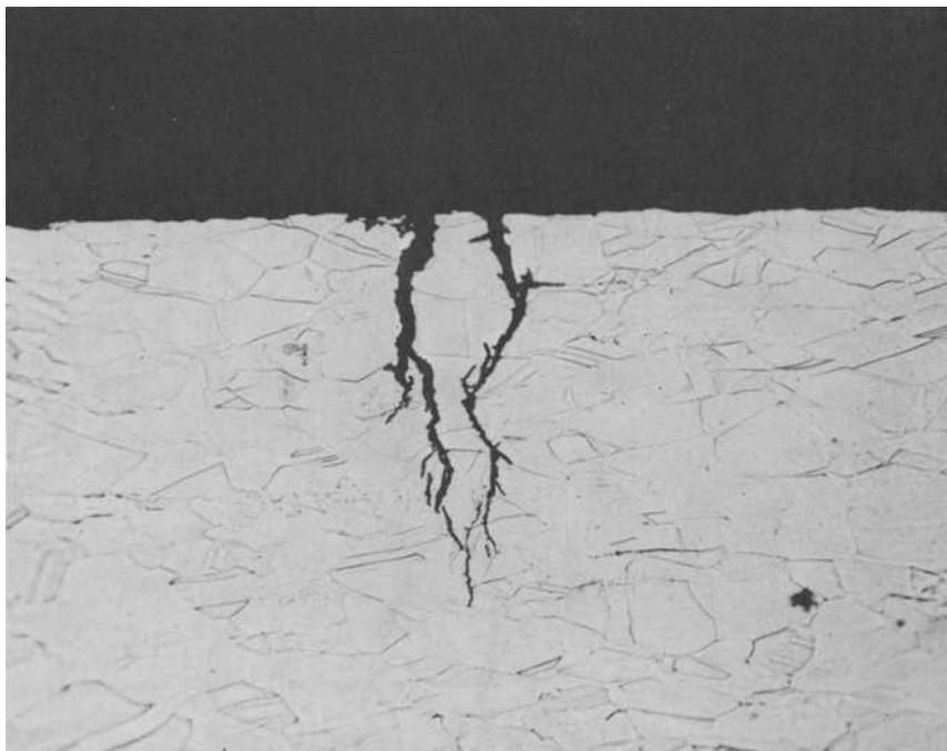
FIG. 4—Alloy B122 (C77000); New Haven, 4 years; exposed surface-initiated SCC showing a transgranular morphology ( \times 375 ).
