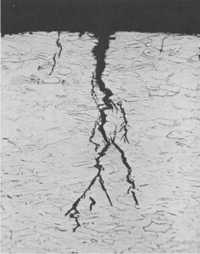
FIG. 3—Alloy B122 (C76200); East Alton, 4 years; surface-initiated SCC with a transgranular morphology ( \times 375 ).
