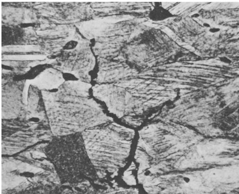
FIG. 6—Alloy B121(C35300); Brooklyn crack morphology is primarily transgranular ( \times 1675 ).
