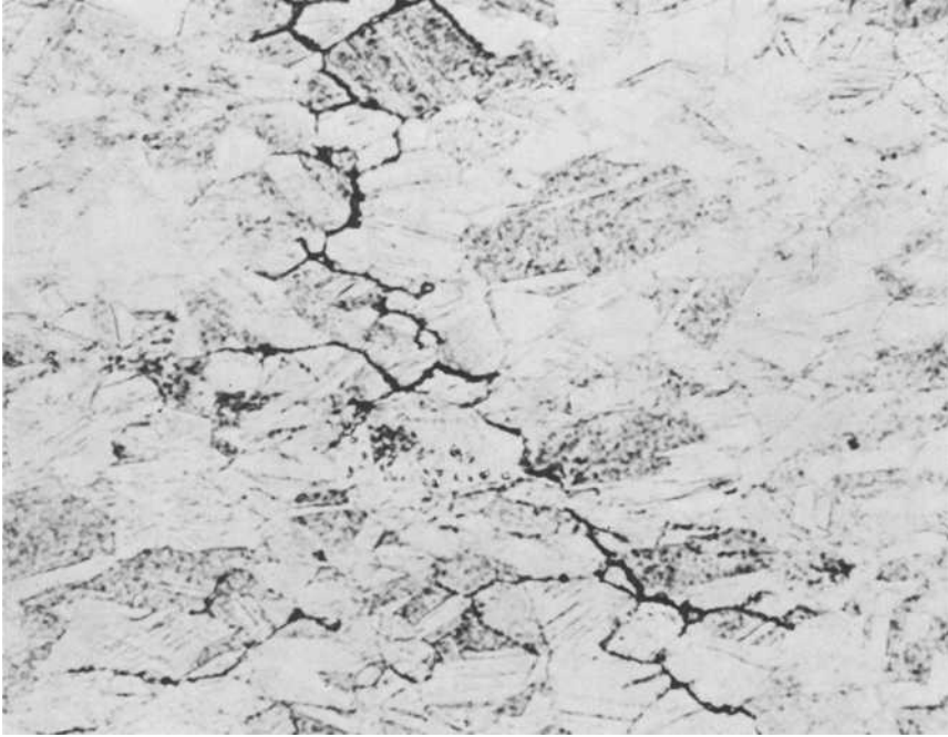
FIG. 5—Alloy B36(C26000); New Haven crack morphology is exclusively intergranular ( \times 400 ).
