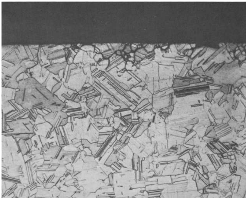
FIG. 1—Intergranular attack. The intergranular penetration is only two or three grains deep, but it did occur on exposure rather than from a mill processing treatment ( \times 300 ).
