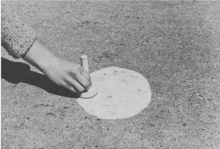
FIG. 1—Operator spreading fine sand with a circular motion of the spreading tool in the sand-patch test.
