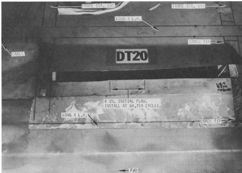
FIG. 26—68 206 cycles: DT 20 final failure (Panel 12, outboard surface) (1 in. = 2.54 cm).
