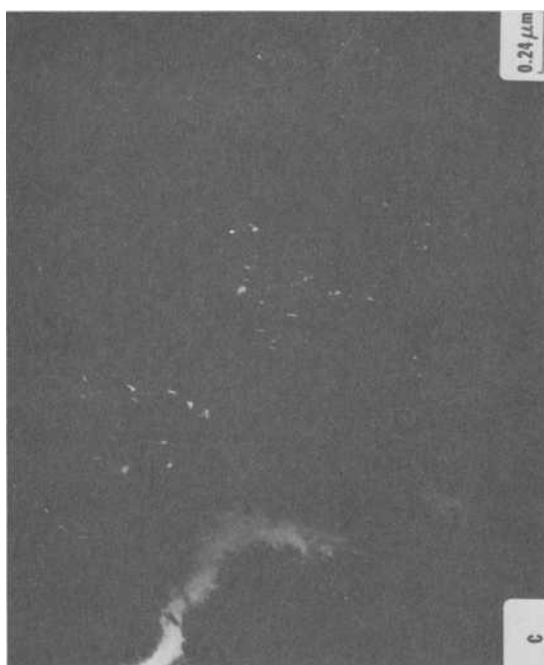
FIG. 9.—Electron micrographs of base + 1Mn alloy cooled at 18°C/min and tempered at 650°C for 4 h. (a) Bright field showing dislocated laths with coarse Fe 3 C and fine alloy carbides (Mo 2 C); (b) Dark field of Fe 3 C; (c) Dark field of Mo 2 C.
