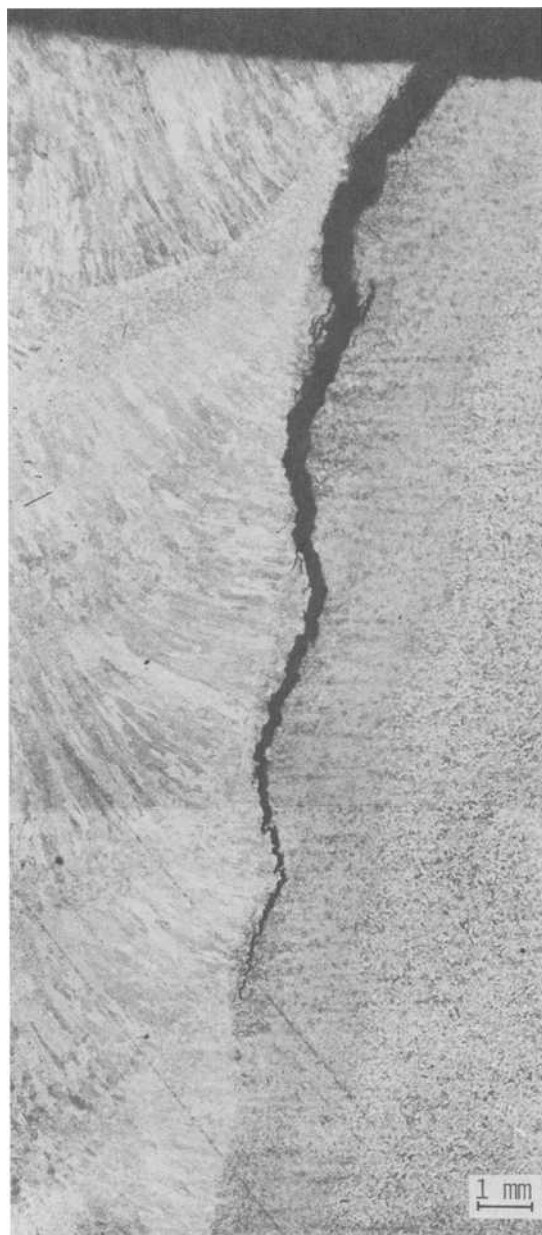
FIG. 19—A crack observed at a nozzle attachment weld of a reactor made of 1\frac{1}{4}\text{Cr}-\frac{1}{2}\text{Mo} steel after approximately eight years of operation at about 530^\circ\text{C} .
