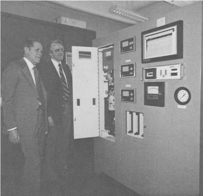
FIG. 7—Westinghouse continuous on-line steam analyzer.
