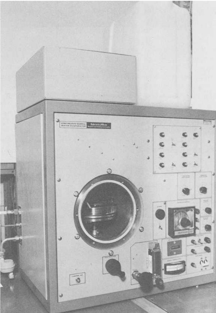
FIG. 1—Continuous sample water evaporator.
