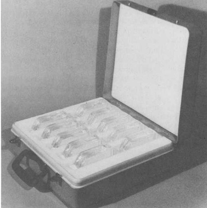
FIG. 2—*Photograph of a grab sample bottle shipping case.*
