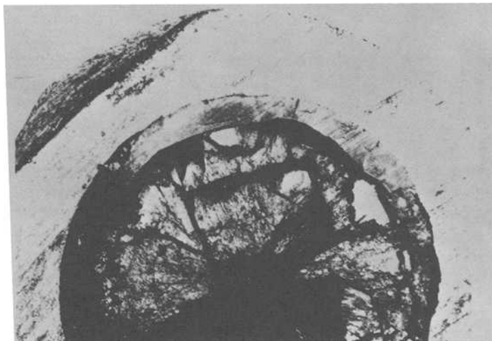
FIG. 1—Cross section of a ferromanganese cylinder (2.54 cm diameter) following immersion for 30 s in a steel bath having an initial superheat of 30°C. (Note the steel shell, the melting zone, and the unmelted core.) [38]
