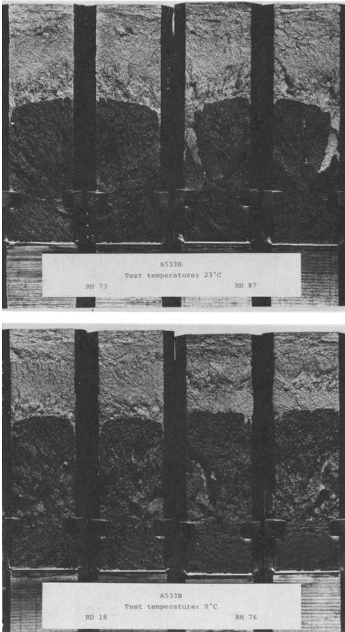
FIG. 6—Photographs of a set of fractured and heat-tinted crack arrest specimens supplied by Laboratory 19.
