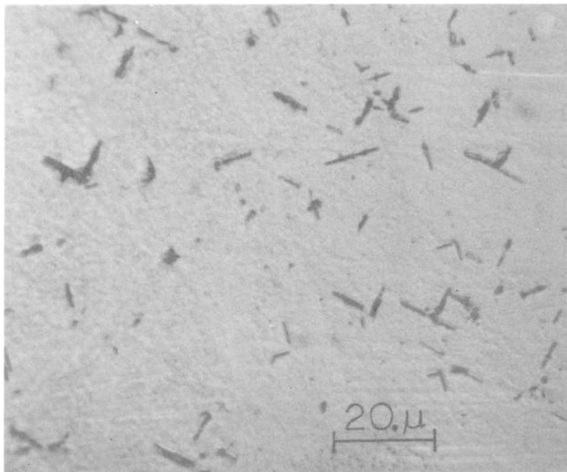
FIG. 6—Light micrograph showing plate-like nitride precipitate in an Fe-26Cr alloy furnace-cooled from 1290°C. Total (C + N) level is 67 ppm [9].
