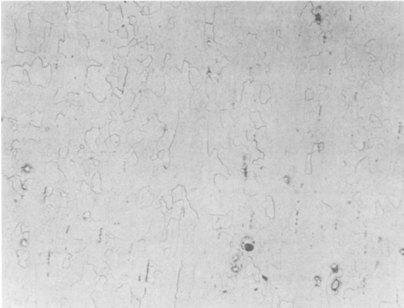
FIG. 2—Representative microstructure of Type 410 stainless steel distillation column tray [heat treated 3 h at 593°C (1100°F)]. ( \times 200 ; etchant, Vilella's).
