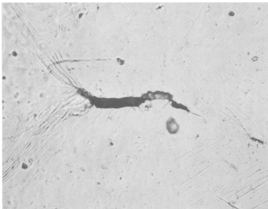
FIG. 4—Optical micrograph of grain boundary fracture on the electropolished surface of a Heat 1 Condition B specimen tension tested at -75^{\circ}\text{C} ( \times 500 ).
