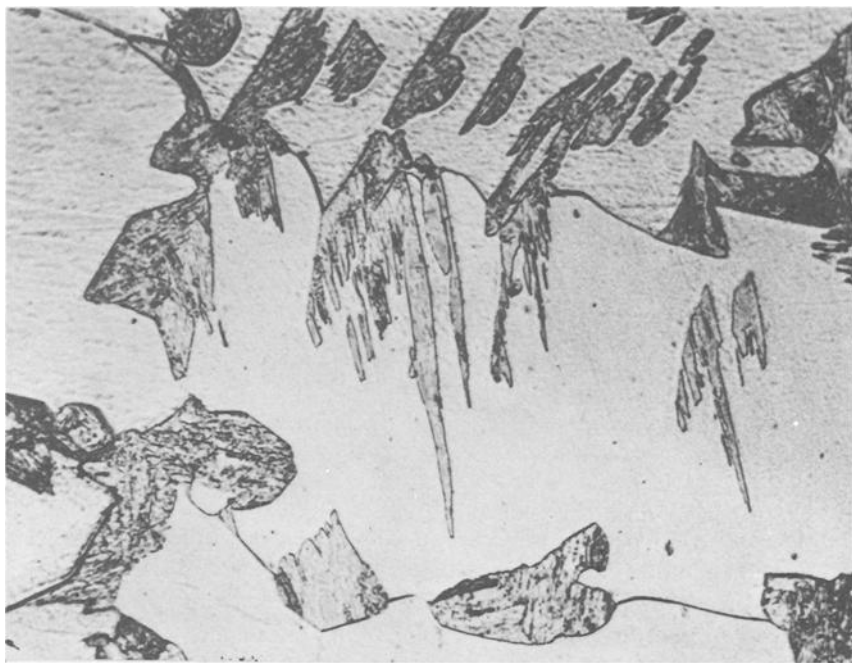
FIG. 5a—HAZ microstructure in SMA B-2. Granular, blocky martensite and angular Widmanstätten intragranular martensite ( \times 300 ).
