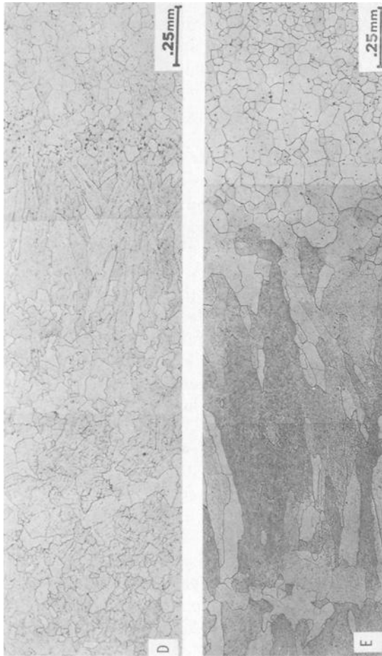
FIG. 4—Typical weld microstructures of 18Cr heats with various levels of residuals. (a) Heat A. low carbon, low titanium, low residuals; (b) Heat B: low carbon, low titanium, high residuals; (c) Heat C: high carbon, high titanium, low residuals; (d) Heat D: high carbon, high titanium, high residuals, (e) Heat E. low carbon, high titanium, low residuals. Magnification: \times 100 ; Etchant: HCl-Picric.
