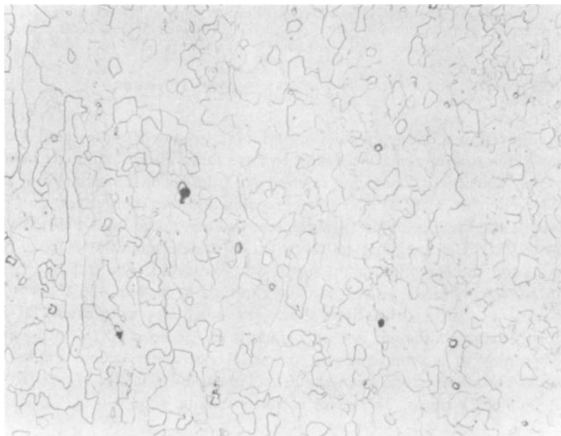
FIG. 1—Representative microstructure of Type 410 stainless steel distillation column tray (as-received condition). ( \times 200 ; etchant: Vilella's)
