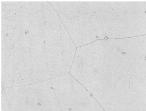
FIG. 3—Optical microstructure of Heat 2 material: \times 525 . Solution annealed at 1290^{\circ}\text{C} for 1 min and iced-brine quenched (Procedure B). note precipitate-free grain boundaries. Same magnification as in Fig. 2.
