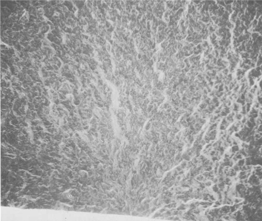
FIG. 8—Radial markings issuing from one of the five origins on sample A2-95.  $\times 300$ .
