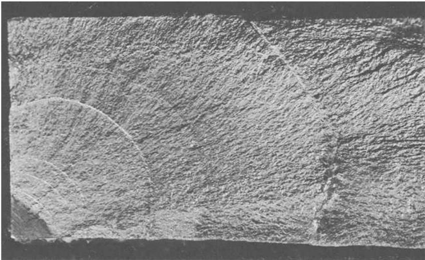
FIG. 6—Fracture surface of a corner crack in an aluminum alloy plate ( $\sigma_y \approx 130 \text{ Nmm}^{-2}$ ). Uniform fatigue markings, introduced by overloads. Notch:  $a = b = 4 \text{ mm}$ .
