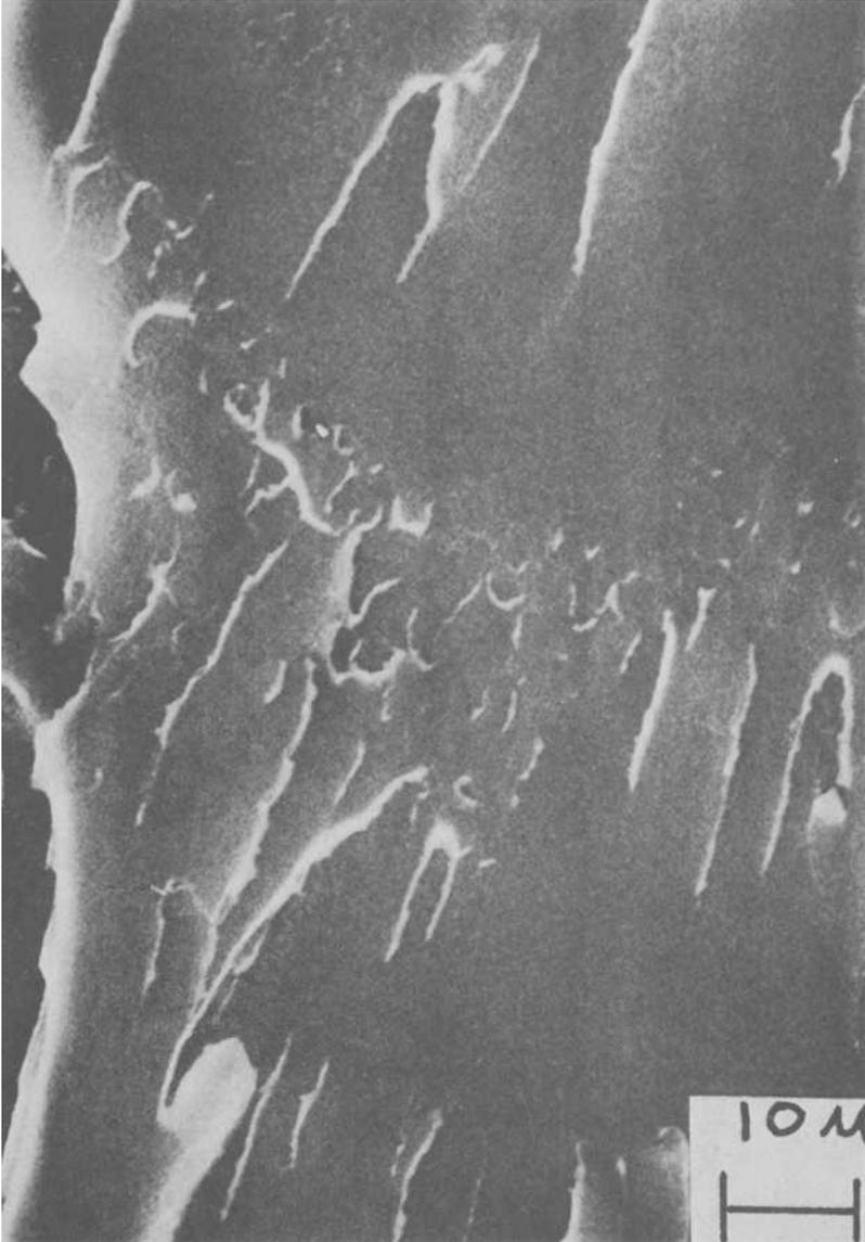
FIG. 6—Surface topology for the slightly plasticized PVC composition. The spall pattern appears random and somewhat shallow. Crack propagation was from the top to bottom of the micrograph.
