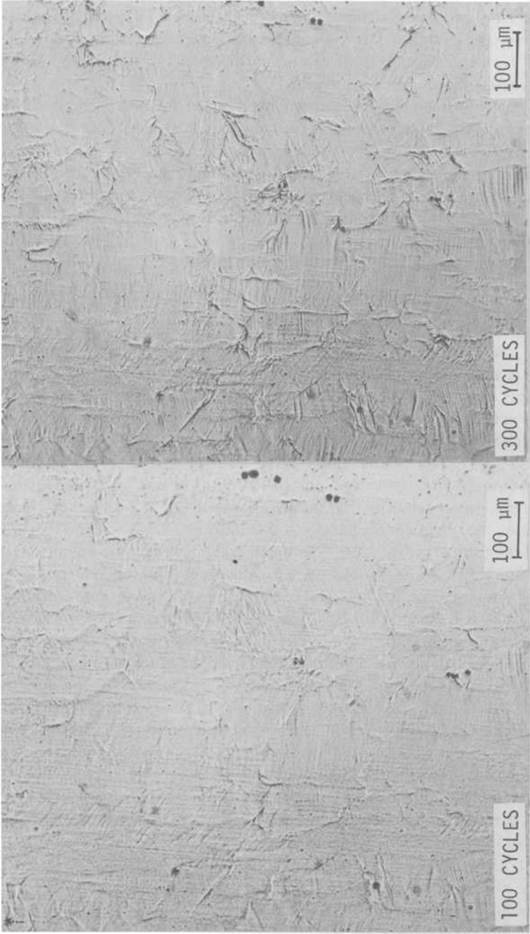
FIG. 6.—Light micrographs of a tension-compression low-cycle fatigue specimen of commercially processed 7050-T6X1. Stress axis vertical, \Delta\epsilon_T/2 = 1.2 percent. Unetched.
