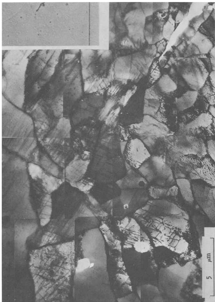
FIG. 5.—Dislocation structure around a long straight crack growing about 45 deg to the stress axis [approximately 90 \mu\text{m} in length; stress amplitude of 20 \text{kg/mm}^2 (196 \text{MN/m}^2 )].
