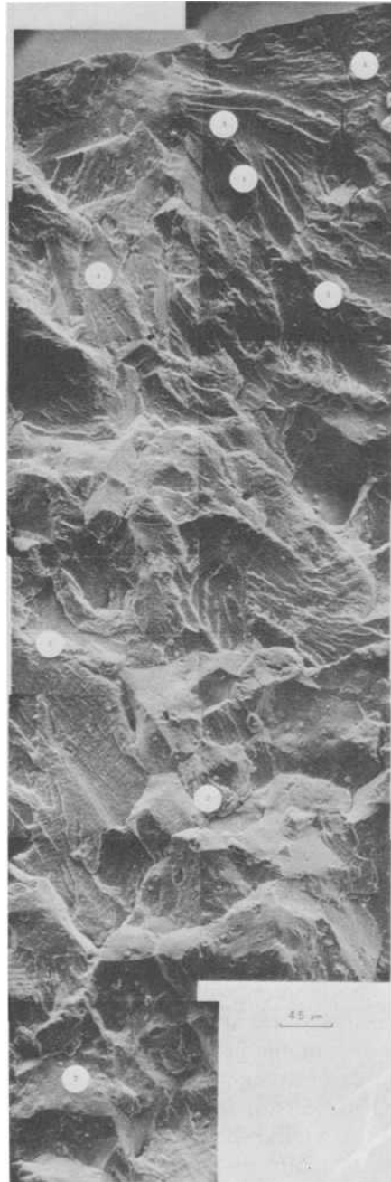
FIG. 4—Transgranular initiation of crack at surface and mixed-mode crack propagation in Hastelloy-X LCF specimen tested at 1033 K, \dot{\epsilon} = 8 \times 10^{-4} \text{ s}^{-1} , and \Delta\epsilon = 0.00615 (1 = striations; 2 = intergranular fracture; 3 = river markings; 4 = secondary crack.)
