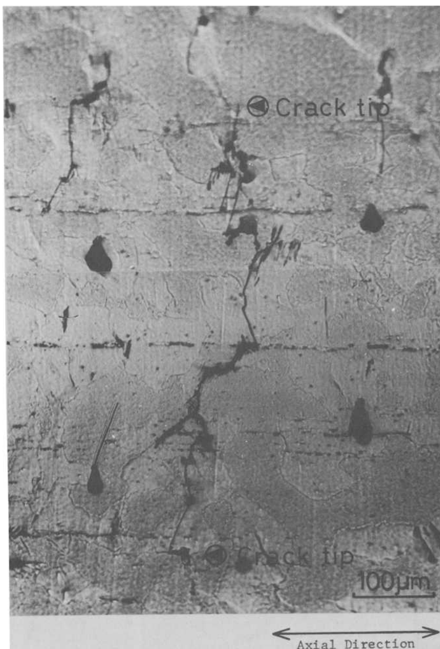
FIG. 6—A typical example of a nonpropagating crack impeded in its propagation by the second-phase martensite after 10^7 cycles. Dark shadowed patches in the photograph are second-phase martensite, ( \sigma = 255 \text{ MPa} , l = 580 \text{ } \mu\text{m} , K = 7.70 \text{ MPa}\sqrt{\text{m}} ).
