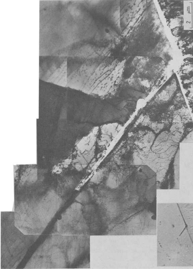
FIG. 6—Dislocation structures around a crack growing along a grain boundary which lies about 45 deg to the stress axis [ 13\text{ }\mu\text{m} in length; stress amplitude of 20\text{ kg/mm}^2 ( 196\text{ MN/m}^2 )].
