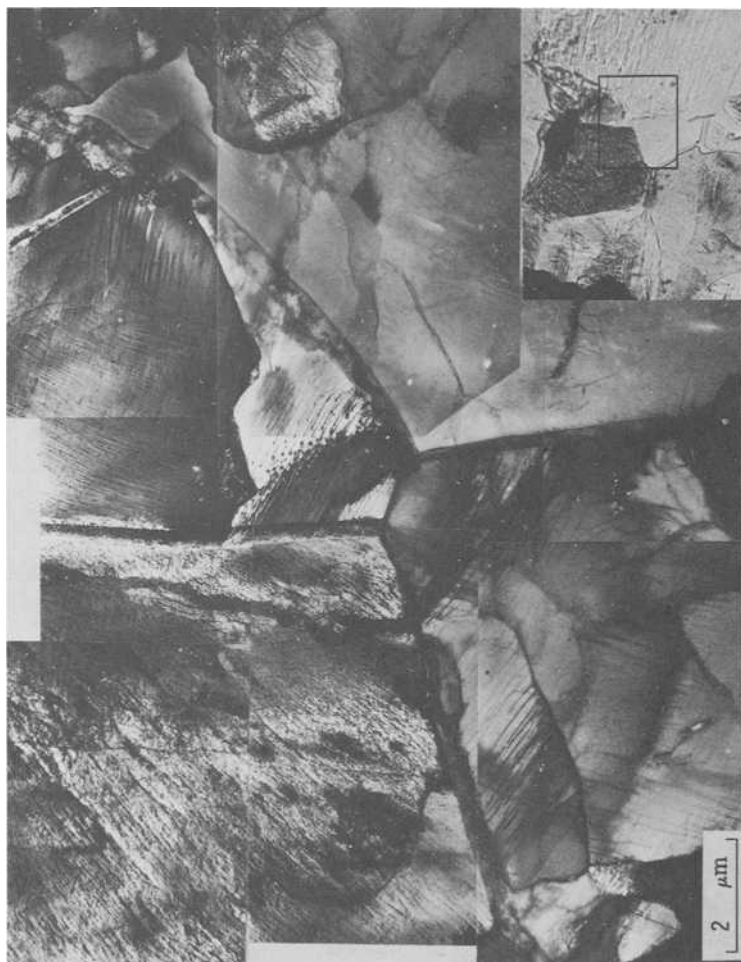
FIG. 2—Well-developed cell structure beneath the surface of the specimen covered with many slip bands; fatigue stress amplitude of 20 \text{ kg/mm}^2 ( 196 \text{ MN/m}^2 ).
