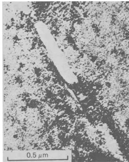
FIG. 4—Transmission electron micrograph showing precipitate-free slipband and subgrains produced in age-hardened aluminum-zinc-magnesium during high-strain torsional fatigue.
