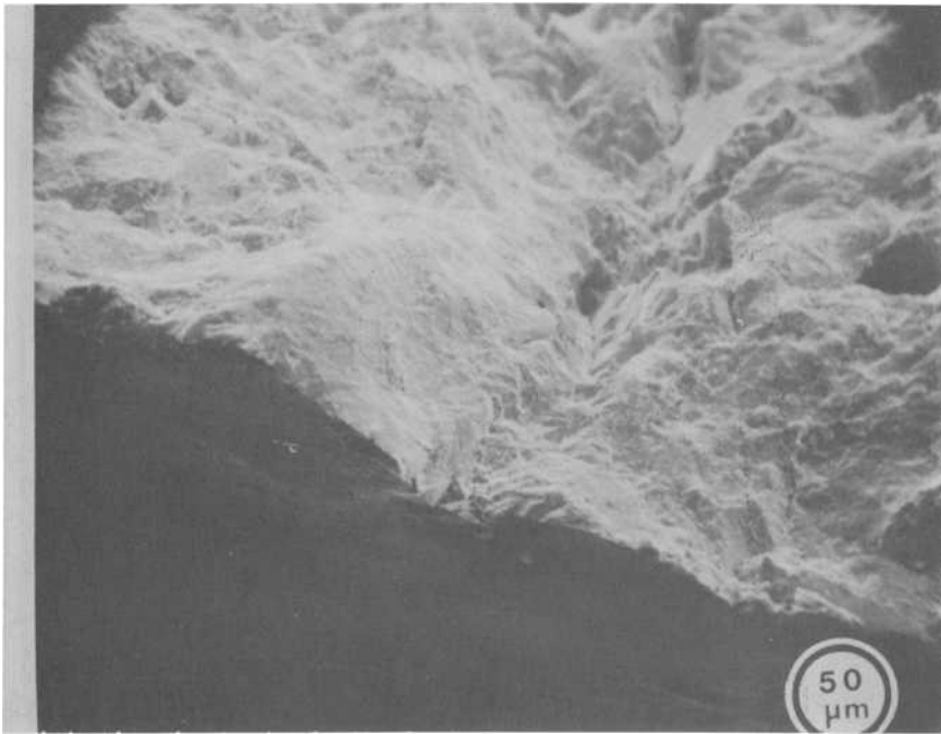
FIG. 12—SEM photomicrograph showing Stage I fatigue crack initiation followed by Stage II crack propagation at 700 K and 9.95 Hz in low-carbon Astroloy with Microstructure IV ( \Delta\epsilon = 2.2 percent).
