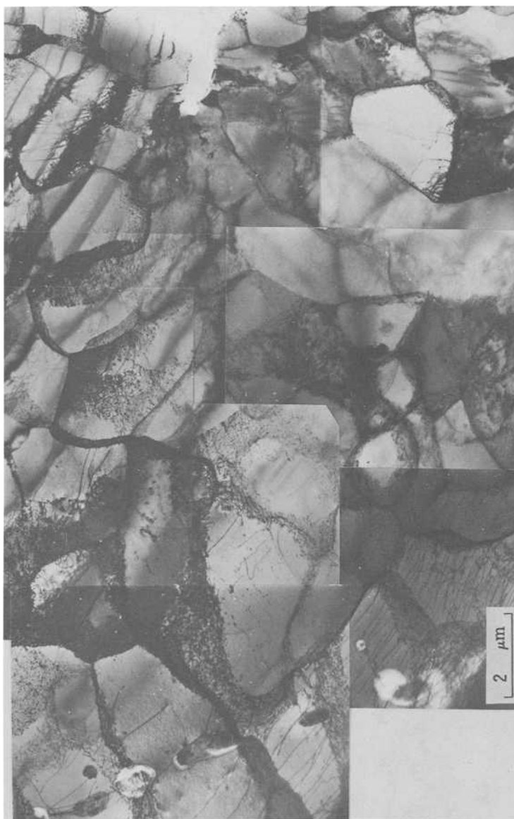
FIG. 8—Dislocation structures around a crack growing in the direction perpendicular to the stress axis [170 \mu\text{m} in length; stress amplitude of 20 \text{kg/mm}^2 (196 \text{MN/m}^2 )].
