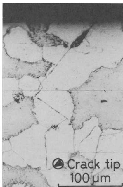
FIG. 9e—Cross-section at Point E (Fig. 8) showing the crack path.
