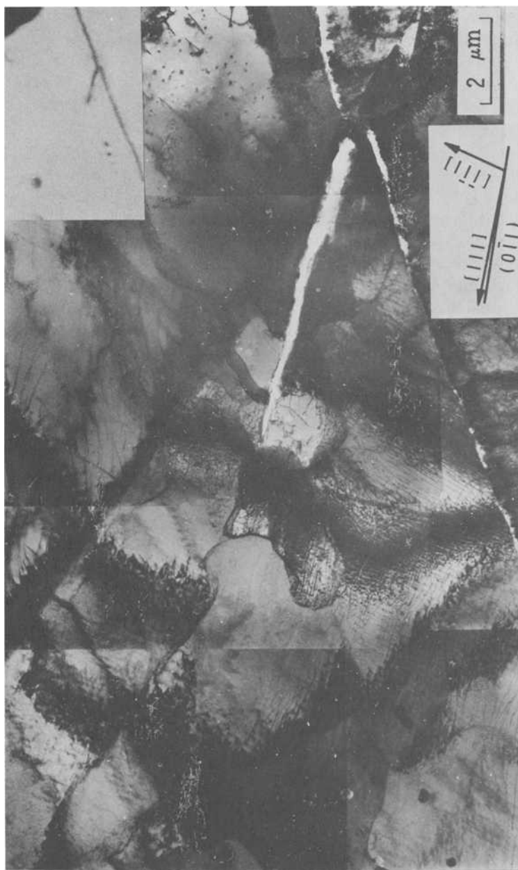
FIG. 3—Dislocation structures around a short straight crack growing about 45 deg to the stress axis [ 7\text{ }\mu\text{m} in length, stress amplitude of 20\text{ kg/mm}^2 ( 196\text{ MN/m}^2 )]. The insert shows the optical micrograph of the foil taken perpendicular to the specimen surface, indicating the crack and the interface between specimen and electrodeposits.
