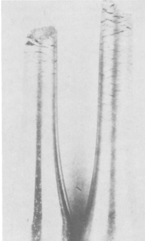
FIG. 1—Severe SCC of carbon steel in slow strain-rate test in  $CO_2$ - $CO$ - $H_2O$  at ambient temperature (original diameter, 2.5 mm).
