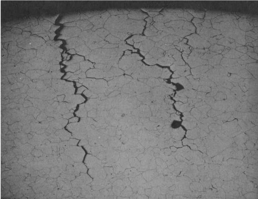
FIG. 37—Stress-corrosion cracking in sensitized Alloy C-276 [36] ( \times 50 ). Specimen: 0.008 percent carbon, heated 1 h at 871^{\circ}\text{C} ( 1600^{\circ}\text{F} ), water quenched, and formed into U-bend. Solution: boiling 45 percent \text{MgCl}_2 ( 155^{\circ}\text{C} ). Specimen exposed 2252 h.
