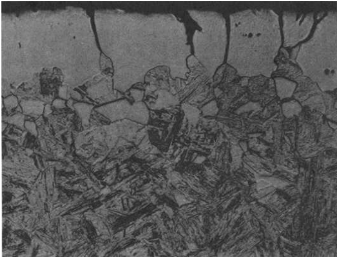
FIG. 6—Intergranular corrosion in decarburized ferritic layer of Type 410 heat treated at 1204^{\circ}\text{C} ( 2200^{\circ}\text{F} ). The cracks do not propagate through the martensite, nitric acid test ( \times 250 ).
