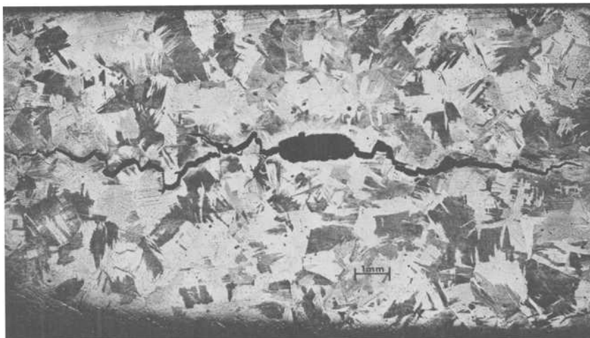
FIG. 1—Fatigue flaw extension from EDM notch.
