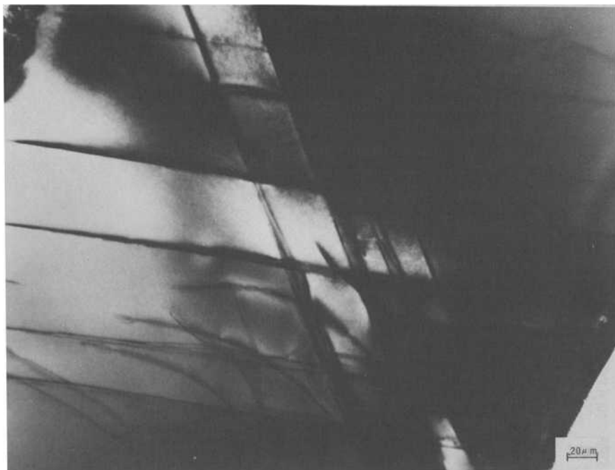
FIG. 8—Transmission electron micrograph of duplex-annealed Ti-6Al-6V-2Sn showing planar arrays of dislocations which result from this heat treatment.
