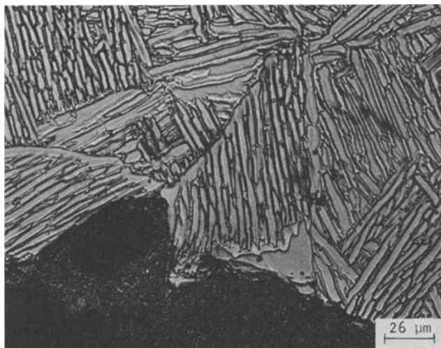
FIG. 18—Optical micrograph of plane normal to fracture plane of duplex-annealed Ti-6Al-6V-2Sn tension specimen showing crack growth occurs by local crack deflection at boundaries of Widmanstätten \alpha - \beta colonies.
