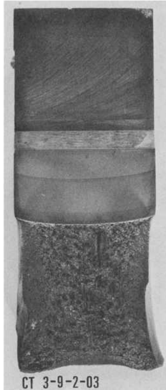
FIG. 4—Fracture surface of base metal specimen.
