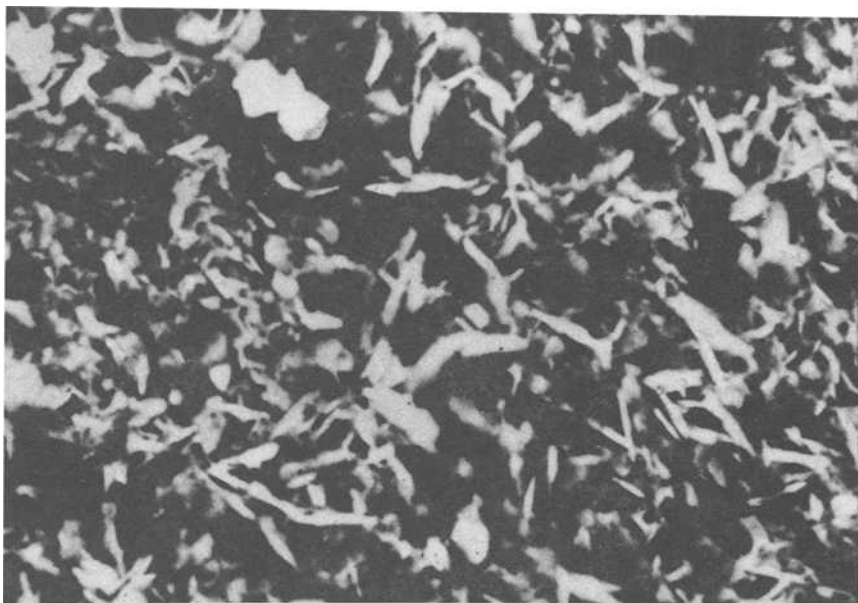
FIG. 4— Scanning electron photomicrograph of an exposed galvanized steel panel showing uniformly dispersed crystalline material over the zinc surface.
