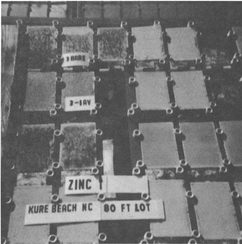
FIG. 5—Test panels at Kure Beach, N.C., 24-m (80-ft) lot, normal mean tide, facing the surf, exposed for 19 years. Three panels at top left are coated with 0.08 mm (0.003 in.) zinc, no sealer. Two panels at center left are coated with 0.08 mm (0.003 in.) zinc.
