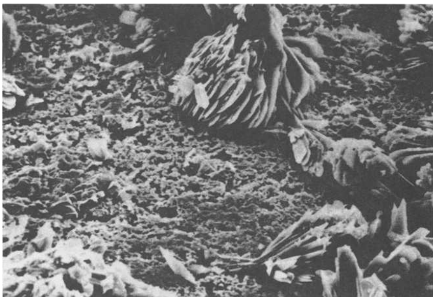
FIG. 3—Scanning electron microscopy ( \times 1000 ) shows brochantite forming at the expense of cuprous-oxide in latter stages of patination.
