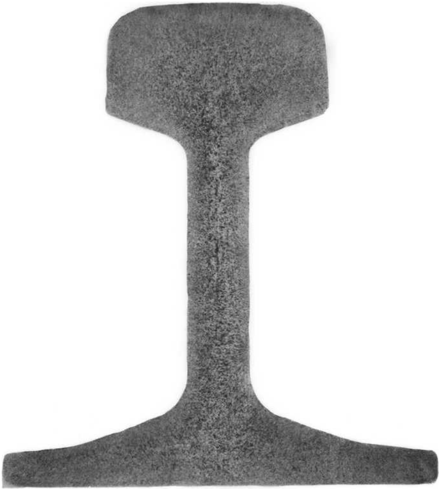
FIG. 1— Typical sulfur print of a rail rolled from a continuously cast bloom.
