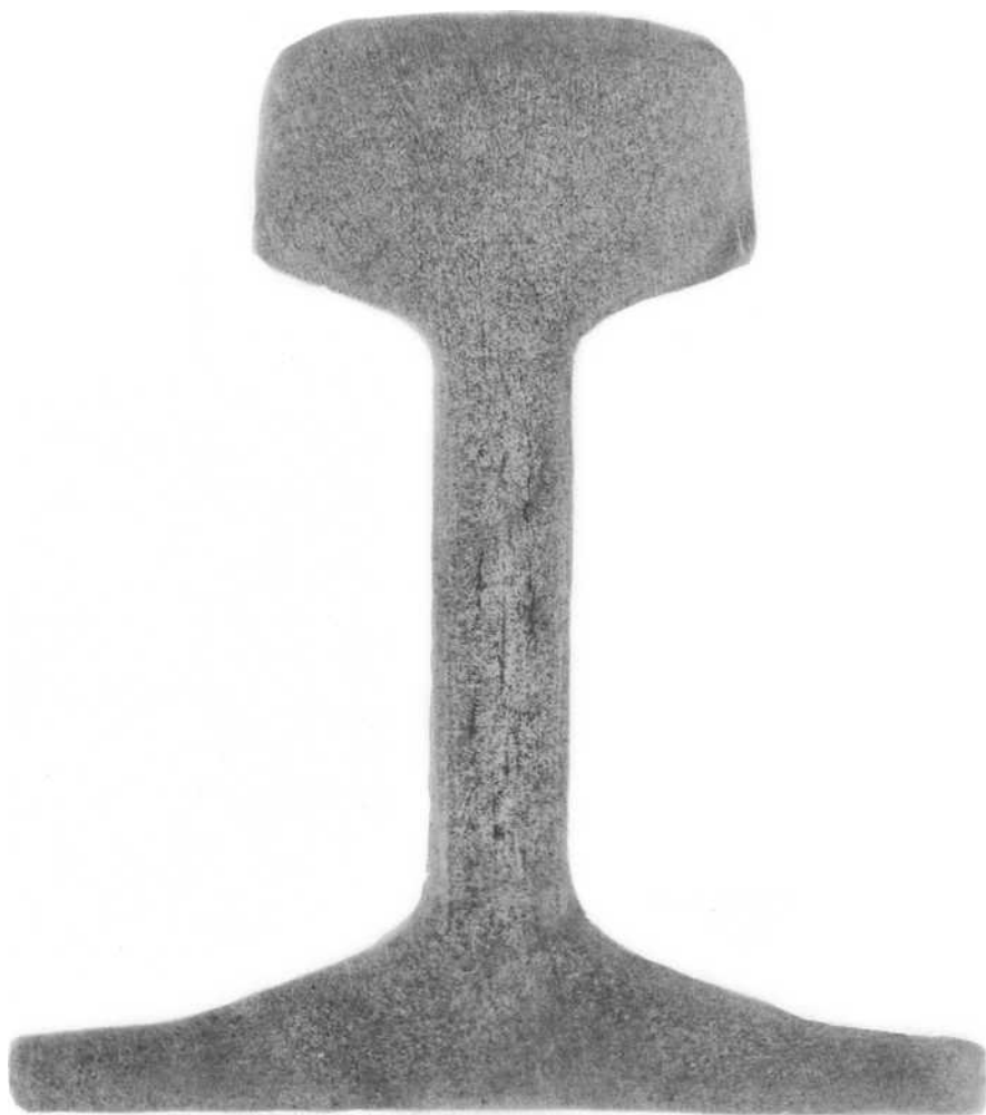
FIG. 2—Sulfur print showing abnormal feature in web of a rail rolled from a continuously cast bloom.
