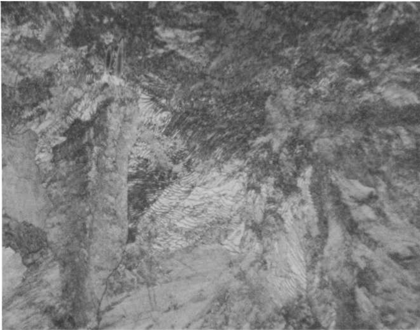
FIG. 1—Photomicrograph of the pearlitic structure typical of the railhead, web, and flange microstructure (from the head); picral etchant, \times 500 .
