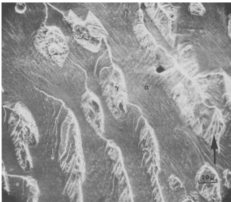
FIG. 13—VK-A271 fracture surface, R = 0.6 . Cleavage-like failure in ferrite phase, white water, \Delta K \approx 20 \text{ ksi}\sqrt{\text{in.}} (22 \text{ MPa}\sqrt{\text{m}}) , \times 425 . Arrow indicates crack growth direction.
