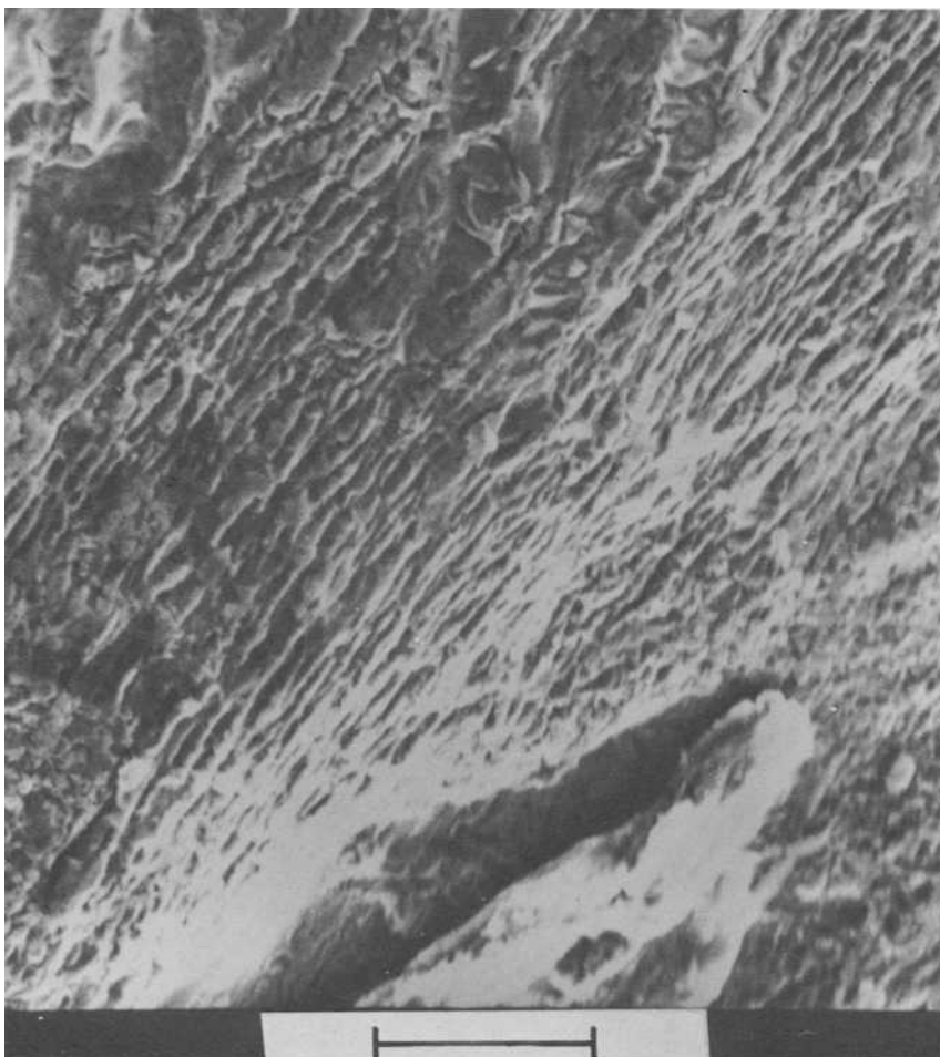
FIG. 3—Fatigue striations along a cleavage facet on crack surface of the second impeller. The specimen was examined using the scanning electron microscope. Scale maker indicates 10 \mu\text{m} .
