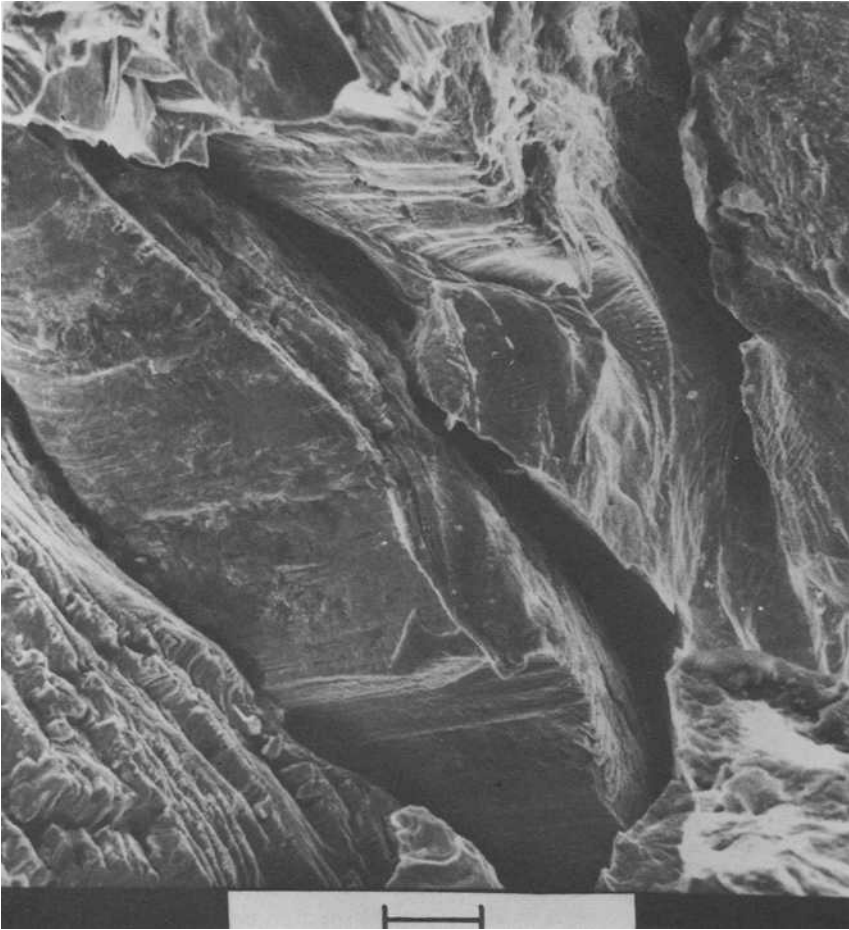
FIG. 4—Area of cleavage fracture on unalloyed tantalum specimen following high frequency fatigue test in sulfuric acid. The specimen was examined using the scanning electron microscope. Scale marker indicates 10 \mu\text{m} .
