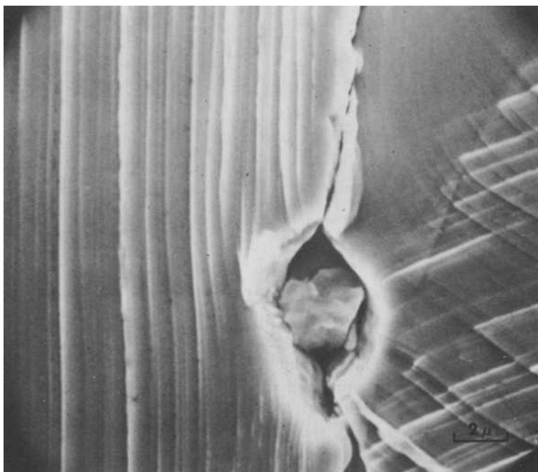
FIG. 7—Crack initiation at inclusion, Alloy 63, air, \sigma_{alt} = 44 ksi (303 MPa), \times 4800 .
