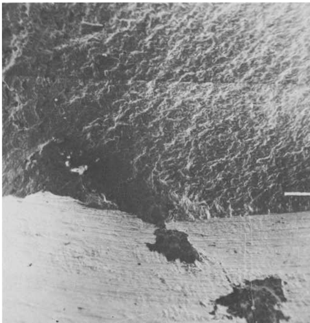
FIG. 6—AFNOR Z3 CNDU 21.7 steel, fracture surface of a rotating-bending specimen tested under a potential of 200 mV at \sigma = 150 \text{ N/mm}^2 . Initiation of the crack at a corrosion-pit. \times 80 .
