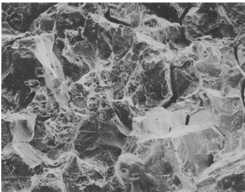
FIG. 5—Fractograph of wrought Inconel 718 compact specimen da/dN tested in 5000-psi ( 34.5\text{-MN/m}^2 ) hydrogen at ambient temperature. \Delta K = 115 \text{ ksi } \sqrt{\text{in.}} ( 126.5 \text{ MN/m}^2 \sqrt{\text{m}} ) ( \times 200 ).
