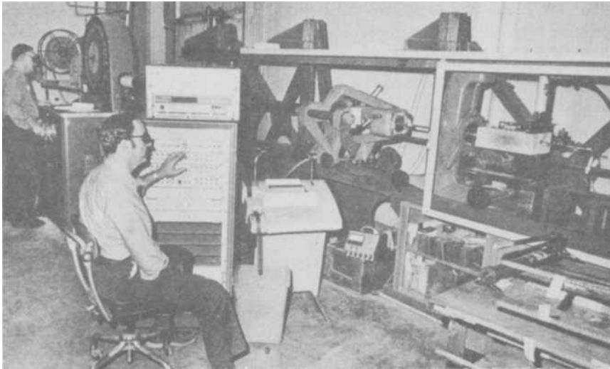
FIG. 4—Overall view of equipment used for conducting load-strength tests on stub-cantilever-beam specimens.
