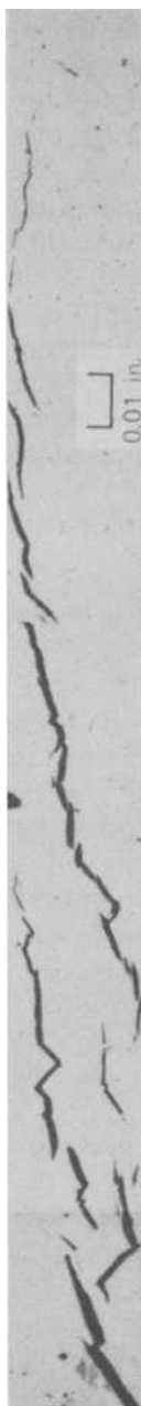
FIG. 1—Microfractures near the crack tip of a DCB specimen of Fe-3Si Steel [4].
