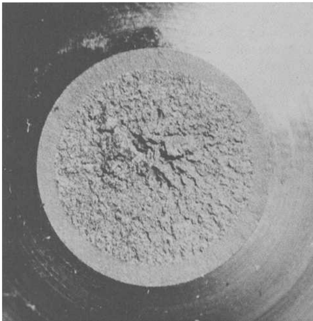
FIG. 2—Fracture surface of prenotched steel bar showing annular fatigue crack.
