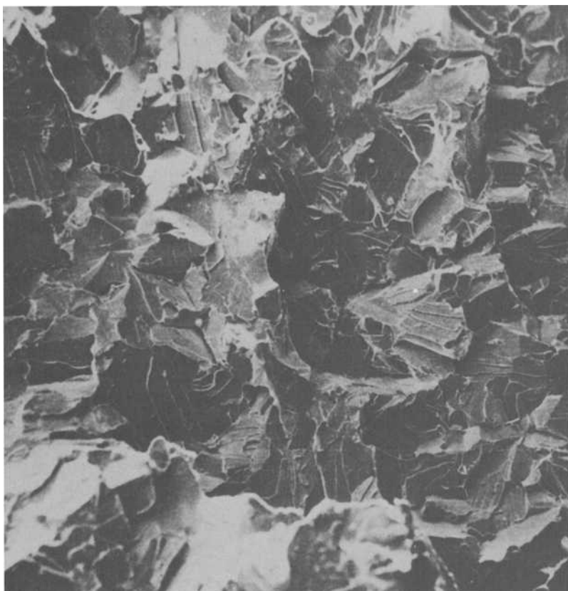
FIG. 10— Fractograph showing very little evidence of ductile fracture in L-specimen tested at 331 K ( \times 125 ).
