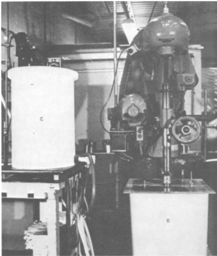
FIG. 4—Impeller tester (A) chuck that holds the impeller, (B) slurry tank, and (C) container for heating deionized water.
