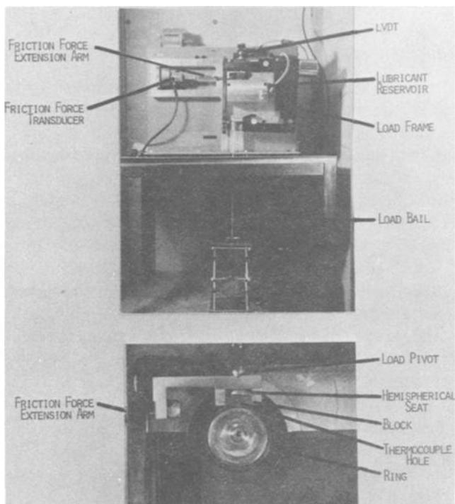
FIG. 3—Falex Model No. 1 (LFW-1) wear test machine. Ring rotates counterclockwise for unidirectional testing.
