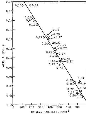
FIG. 7—Relationship between original hardness of various constructional and structural low alloy steels and the weight loss in the pin abrasion test. Numerals at data points indicate the carbon content in percent.
