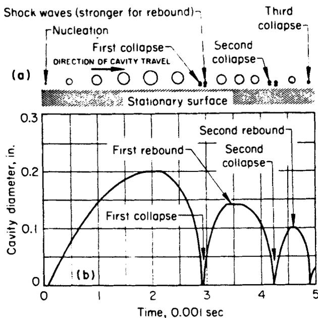
FIG. 4—(a) Schematic representation of successive stages of growth, collapse, and rebound of a single traveling cavity. (b) Graph of cavity diameter as a function of time for the cavity in (a) [5,7].
