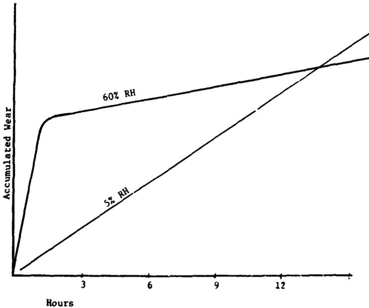
FIG. 2—Accumulated wear after various times of sliding of 1.5Mn steel using a cross-cylinder apparatus [8].
