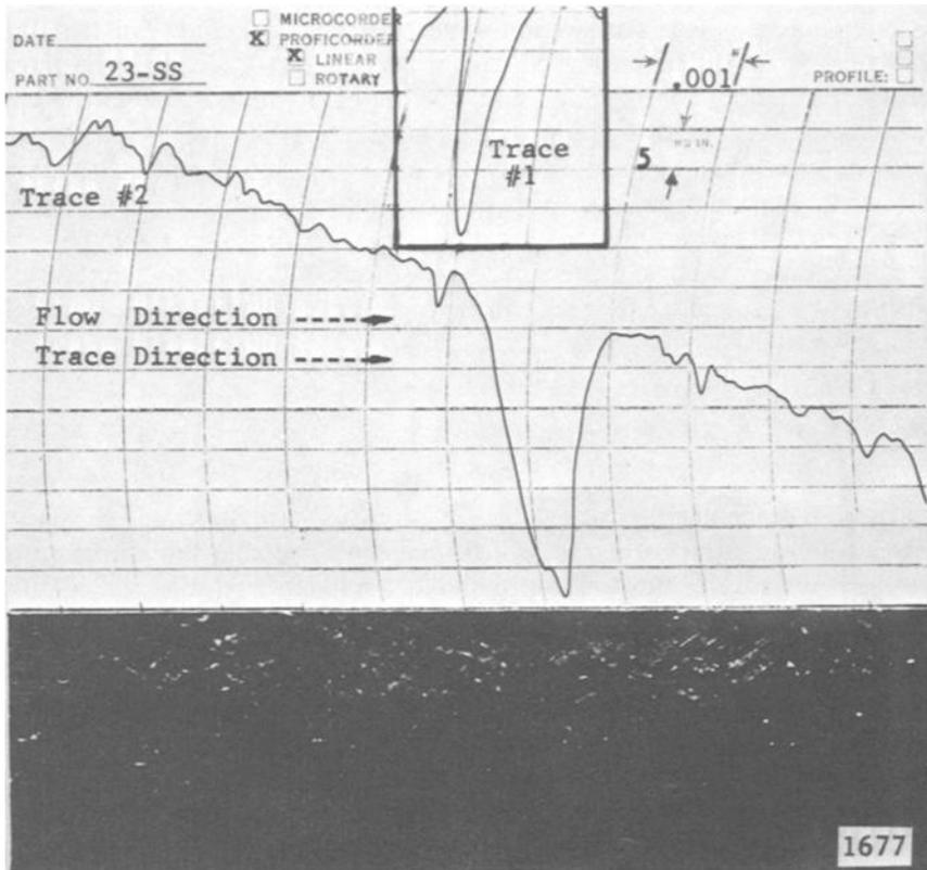
FIG. 5—Individual blow cavitation craters on stainless steel.
