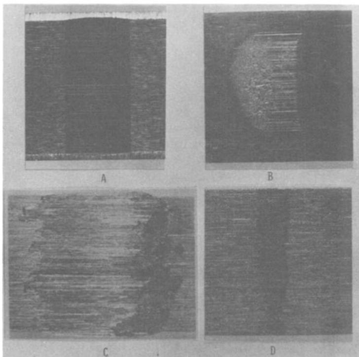
FIG. 5—Block scars after Falex Model 1 testing showing (A) a clean straight-edged scar, (B) a scar with a build-up of granular debris, (C) a scar with extensive plastic deformation, and (D) a scar with a jagged edge (approximately X6).
