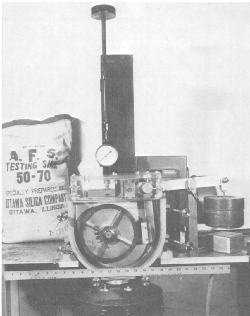
FIG. 3—Front view of the rubber wheel abrasion machine (front cover of the slurry cage has been removed).
