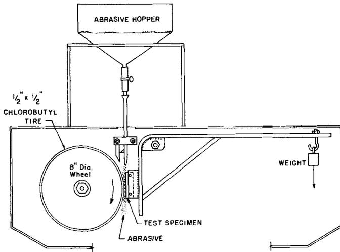
FIG. 1—Schematic diagram of dry-sand low-stress rubber wheel abrasive wear tester.
