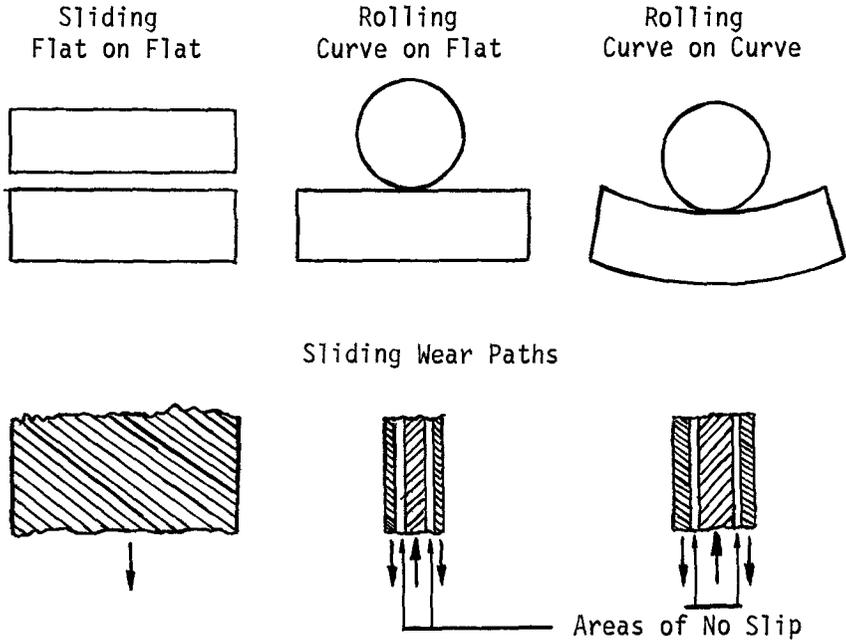
Relative Direction of Motion Due to Slip Between Surfaces
