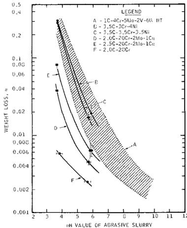
FIG. 10—Weight loss of a tool steel and several types of alloyed white irons in a low-stress impeller test under the conditions of various pH values.
