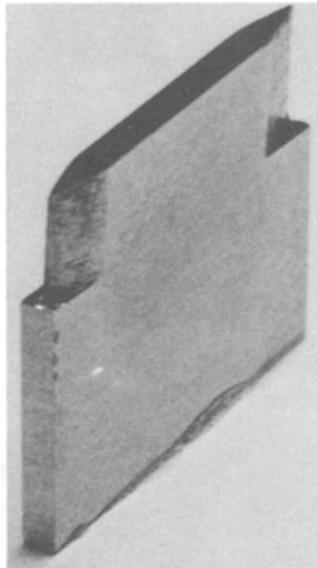
FIG. 8—Venturi device for cavitation damage tests at the University of Michigan: (top) cross section of the venturi device, and (bottom) specimen from the venturi device. (By permission, from Hammitt, F. G., *Journal of Basic Engineering*, American Society of Mechanical Engineers, Vol. 85, 1963, pp. 347-359.)
