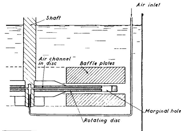
FIG. 11—Rotating disk with drill ducts for air supply.
