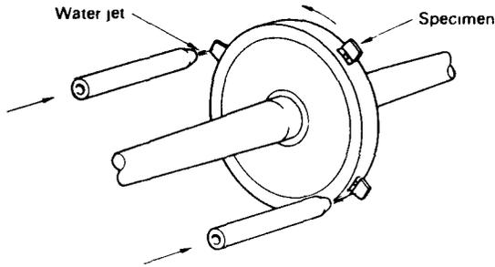
FIG. 6—*Jet impact damage device (schematic)*. (By permission, McGraw-Hill, copyright 1970, from Ref 6.)
