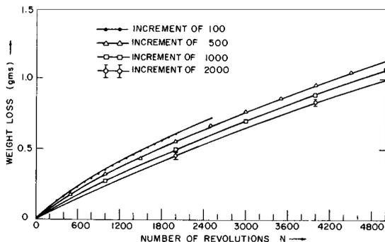
FIG. 2—Total weight lost for annealed HR 1020 steel during abrasion testing at different increments.
