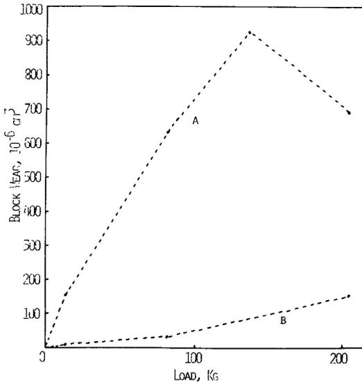
FIG. 4—Block scar volume as a function of load after testing in Falex Model 1 at 180 rpm for 5400 revolutions in Mil H5606A hydraulic fluid of (A) plasma-deposited aluminum rings and (B) modified plasma-deposited aluminum bronze blocks against SAE 4620, R<sub>c</sub>60, steel rings.
