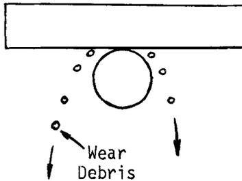
FIG. 2—Disposition of wear debris.
