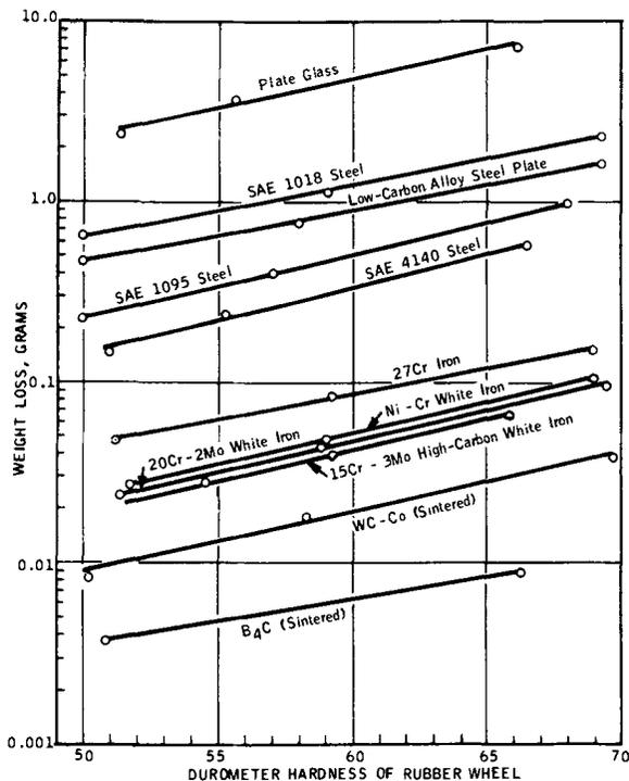
FIG. 8—Weight loss of various materials as determined from the rubber wheel abrasion test at different levels of rubber hardness.
