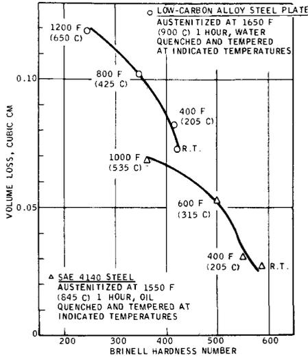
FIG. 9—Volume loss of two constructional steels plotted against hardness. (Abrasion resistance indicated in terms of volume loss normalized to 55 durometer hardness of the rubber wheel.)
