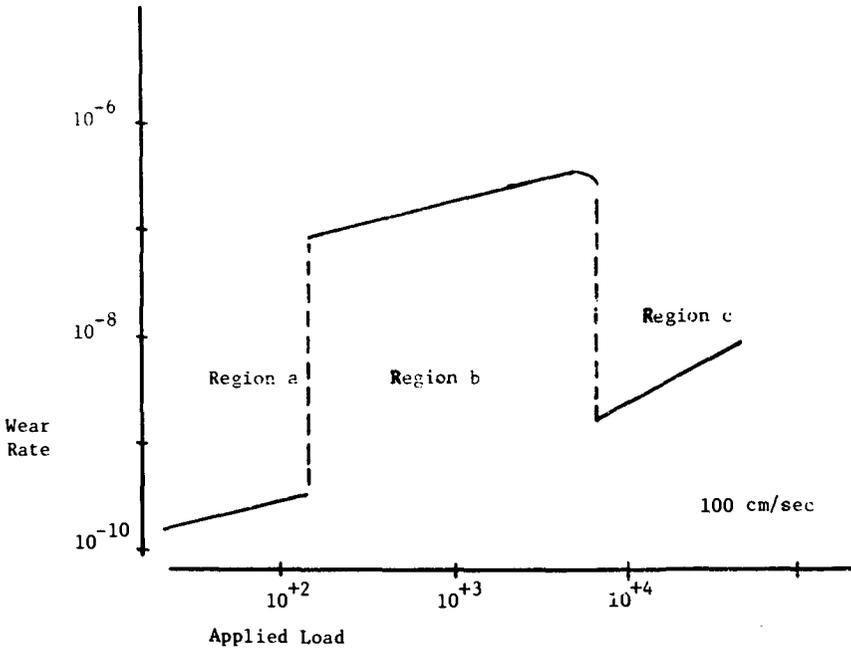
FIG. 1.—Wear rate of 1052 steel pin at various applied loads from a pin-on-ring apparatus [2].
