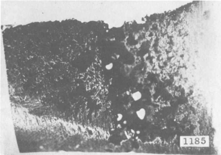
FIG. 1—Leading edge of a series 400 stainless steel impeller for a boiler feed pump, exhibiting deep local damage caused by cavitation erosion.
