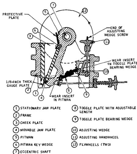
FIG. 1—Schematic sketch of the main components of the jaw crusher.
