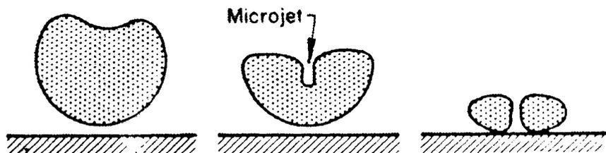
FIG. 3—Schematic representation of successive stages of nonsymmetrical cavity collapse with microjet impingement against a metallic surface. (By permission, from *Metals Handbook*, Vol. 10. Copyright American Society for Metals, 1975.)
