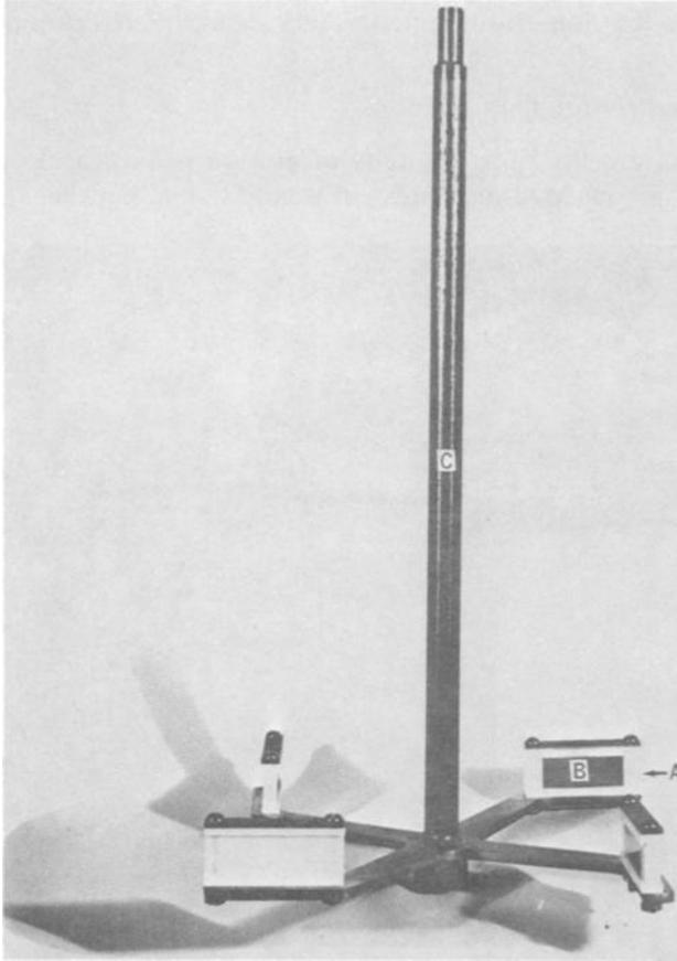
FIG. 5—Impeller (A) Teflon holder, (B) specimen, and (C) shaft.
