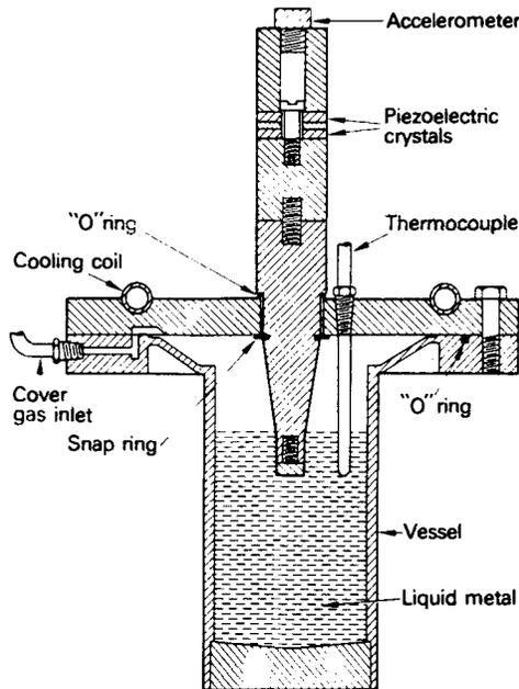
FIG. 13—Liquid metal vibratory facility at the University of Michigan. (By permission, McGraw-Hill, copyright 1970, from Ref 6.)
