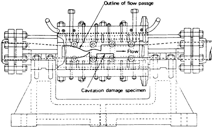
FIG. 9—Holtwood Laboratory cavitation damage test section [21].
