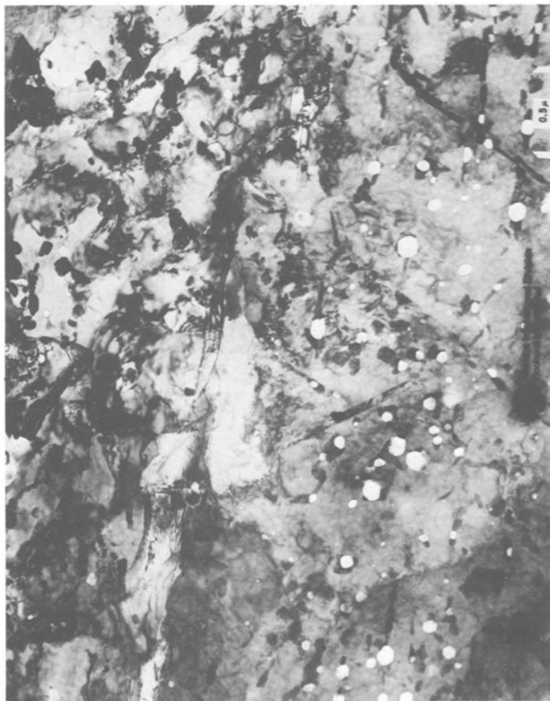
FIG. 2.—Electron micrograph of a grip end (unstrained) of a tension specimen of Type 316 stainless steel, 25 percent cold-rolled, irradiated at 600 to 535°C (1112 to 995°F) to 7.3 \times 10^{26} \text{ n/m}^2 ( E > 0.1 \text{ MeV} ) and tension at 575°C (1067°F).
