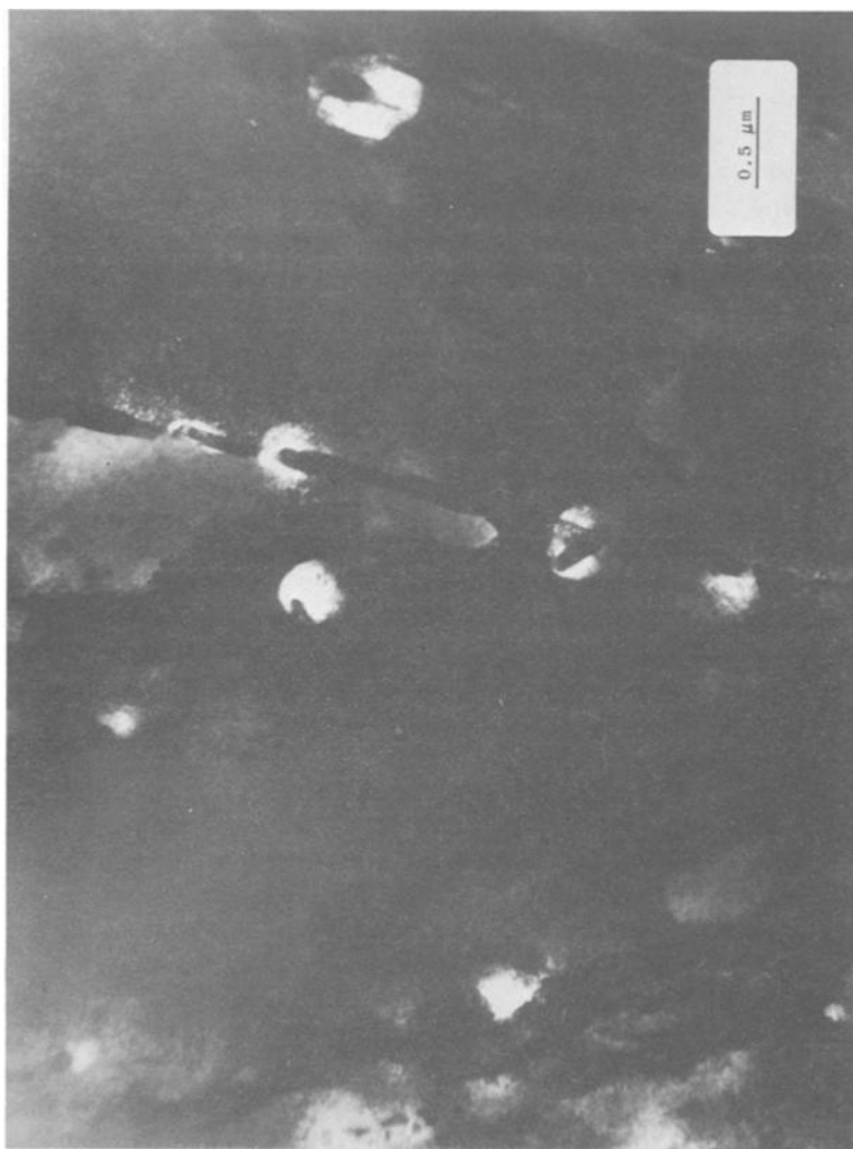
FIG. 2.—TEM of voids associated with precipitates along a grain boundary in a thick section of HT-9 specimen bombarded to a fluence of 250 dpa at 500°C (932°F).
