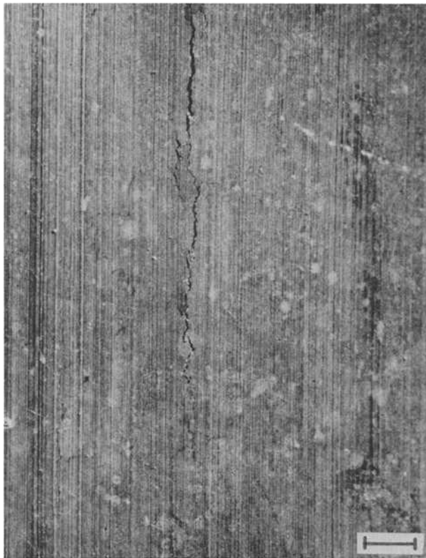
FIG. 6—Stress-corrosion crack after 2000 h exposure to clean air (mark = 1 mm).
