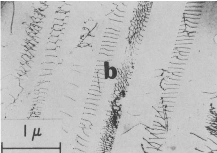
FIG. 10—Electron micrographs of thin-foil specimens of austenitic stainless steels showing dislocation arrays. (b) 12.8 percent nickel, 0.12 percent nitrogen steel showing deformed, planar array; (c) 20 percent nickel, 0.1 percent carbon steel deformed 10 percent showing cellular tangled array [59].
