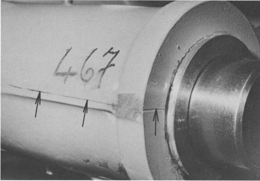
FIG. 4—Stress-corrosion crack in the parting line and through the full-wall thickness of a 7079-T6 aluminum forged landing gear ( \times 0.8 ).
