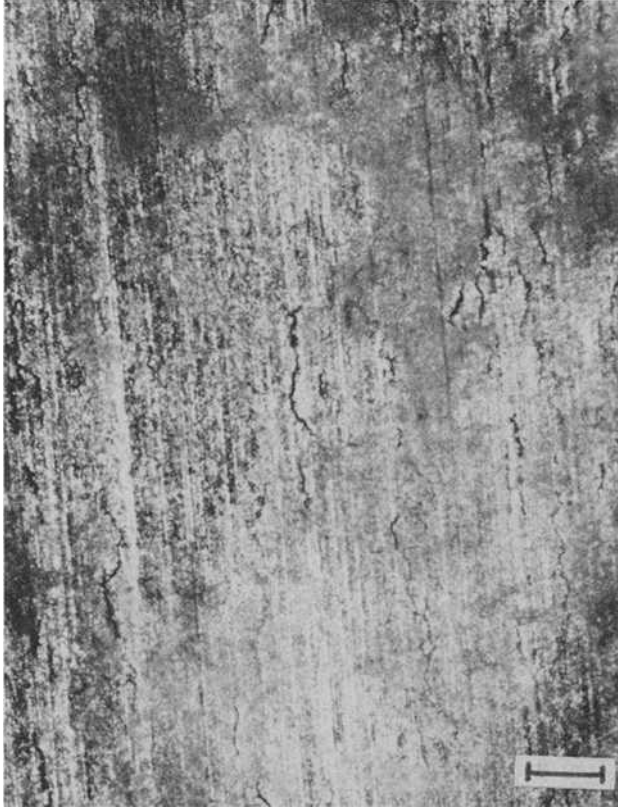
FIG. 4—Stress induced intergranular cracks in 7005-T53 after 1000 h exposure to air containing \text{SO}_2 (mark = 1 mm).
