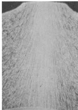
FIG. 6—Macrostructure of a transverse section through the parting line of a 7079-T6 aluminum landing gear forging showing the long thin grains in the immediate vicinity of the parting line ( \times 3 ).
