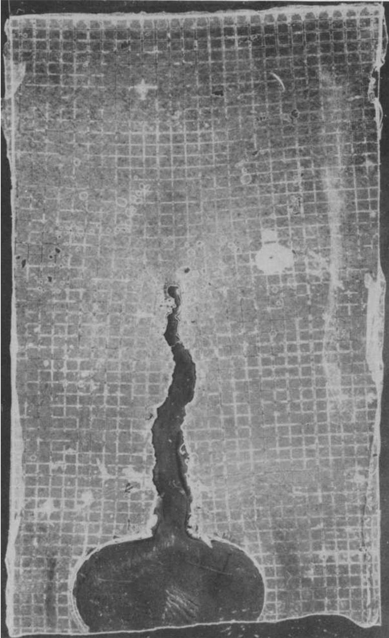
FIG. 2—Enlargement of replica at area of high-strain gradient.
