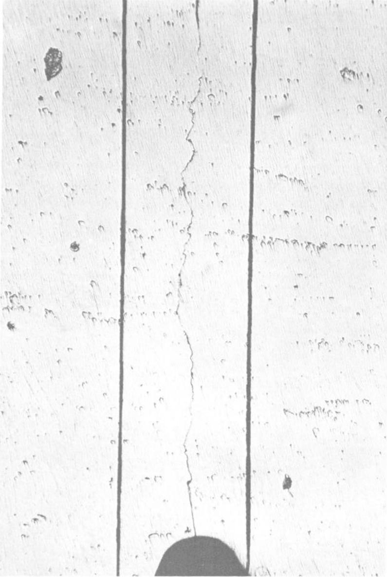
FIG. 2—Photomicrograph of a set of grooves applied parallel to a fatigue crack. The grooves are  $5\ \mu\text{m}$  wide and  $0.25\ \text{mm}$  ( $0.010\ \text{in.}$ ) apart.
