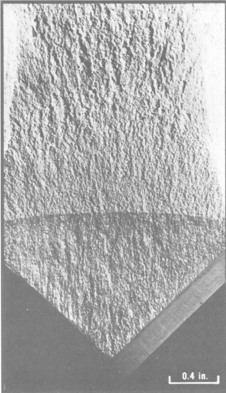
FIG. 12—Fracture surface of  $K_{Icc}$  fracture in 2219-T851 plate at 300°F.
