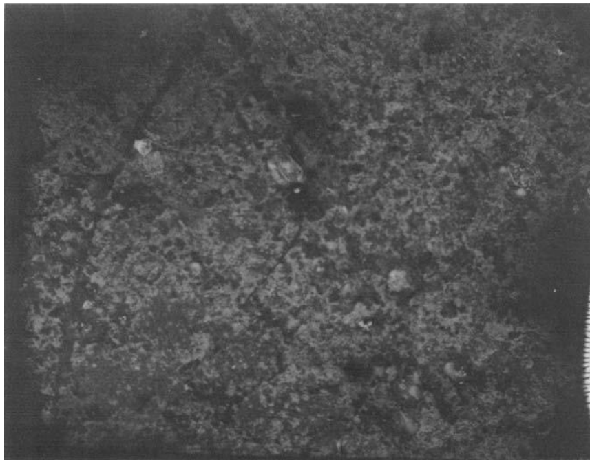
FIG. 8—Scanning electron microscopy of galvanized steel corrosion products from clean air exposure (X50).
