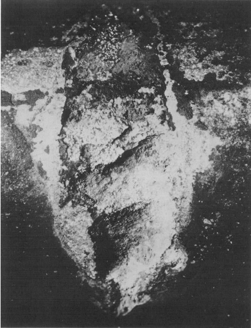
FIG. 1— Pitting attack carbon steel heat exchanger tube, area of through performance, X10.
