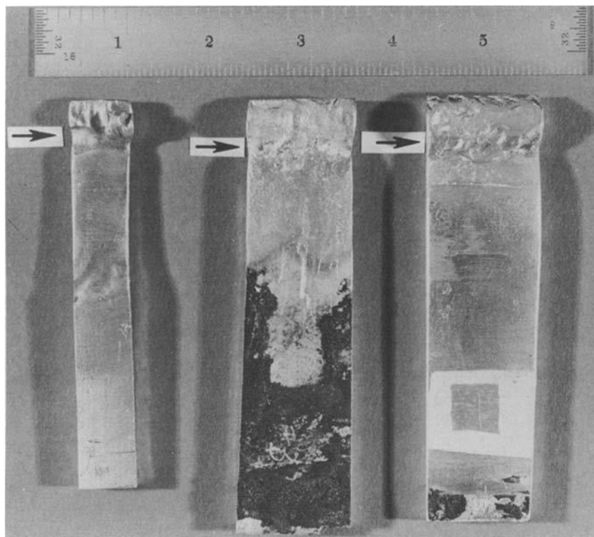
FIG. 10—Three specimens from Figs. 8 and 9 showing the corrosion in the HAZ and the lesser attack on the FM.
