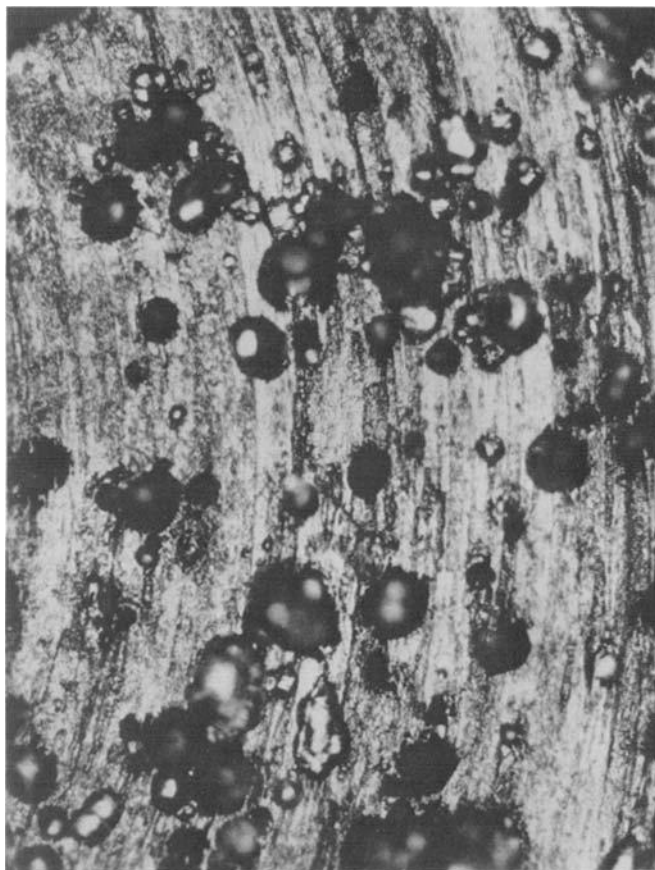
FIG. 12—Pitting on nickel after test in 2 N H_2SO_4 in CH_3OH ; magnification approximately \times 180 .
