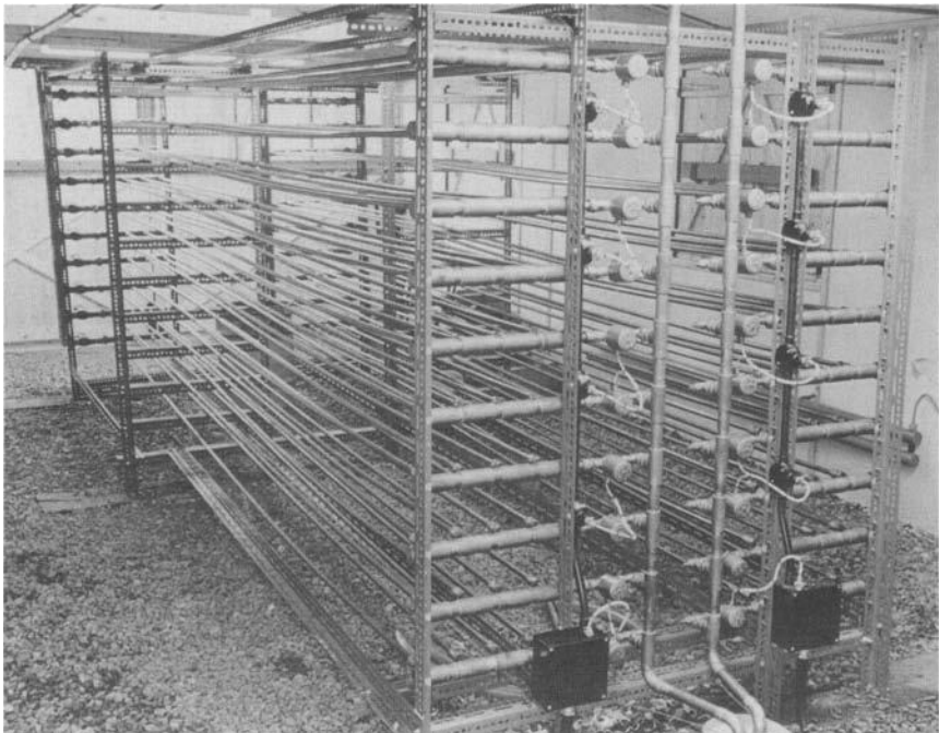
FIG. 1—Corrosion rig at the Bramham site.
