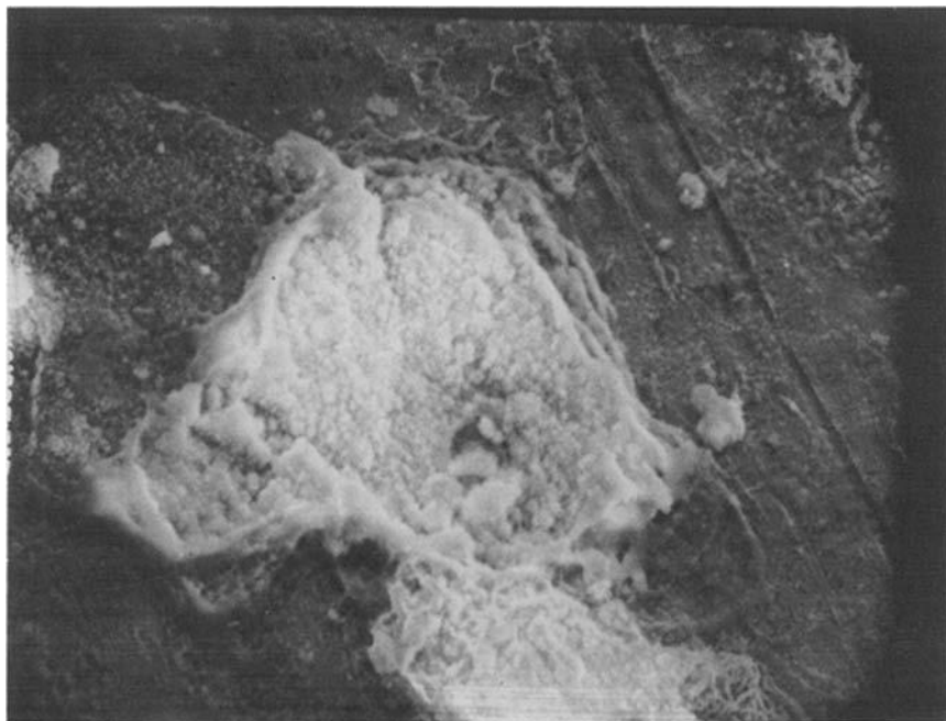
FIG. 9—Scanning electron microscopy of galvanized steel corrosion products from clean air exposure ( \times 1000 ).
