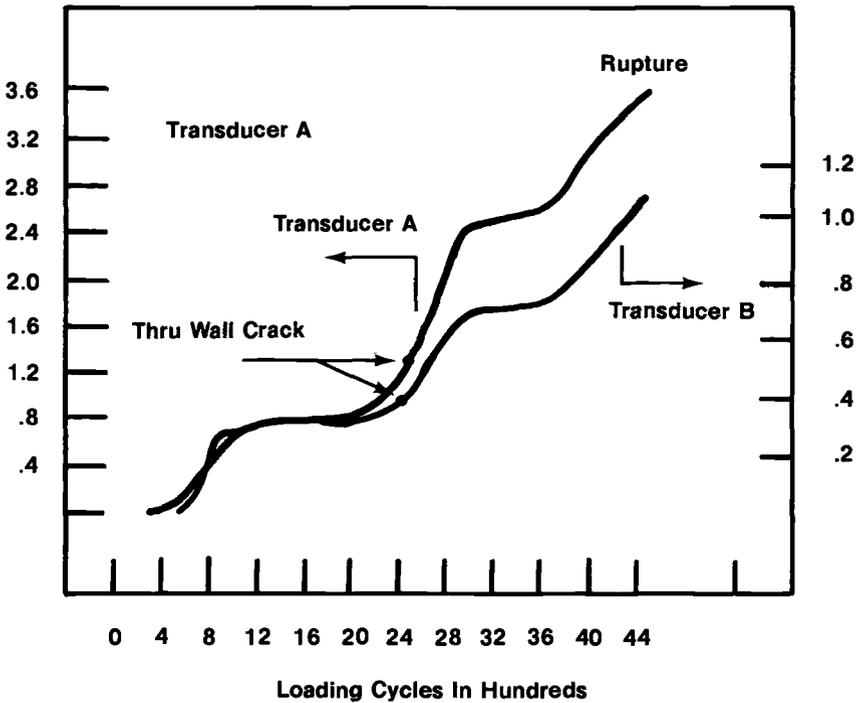
FIG. 5—Fatigue cycles versus total counts.
