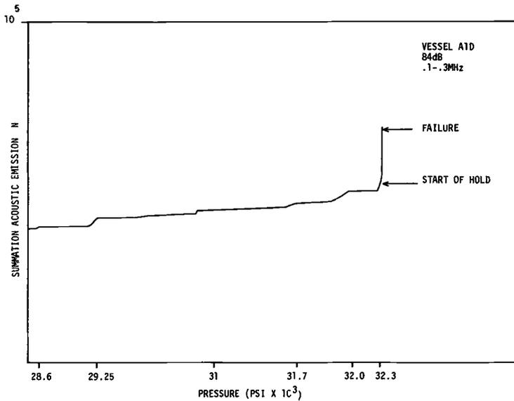
FIG. 10b—Summation of acoustic emission versus pressure 28 600 to 32 200 psi Vessel A1-D.
