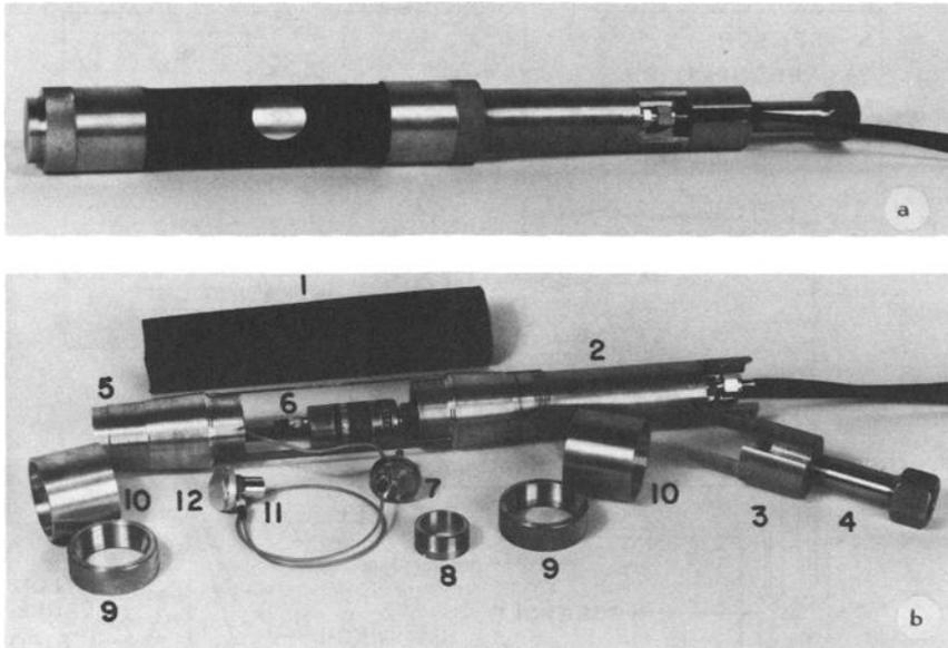
FIG. 7.—Mark II model acoustic emission borehole probe (support rod and associated adapter not shown). (a) Probe assembled ready for use. (b) Borehole probe disassembled showing component parts (1 = rubber bladder, 2 = probe body, 3 = connecting rod yoke, 4 = pipe adaptor, 5 = probe end section, 6 = preamplifier, 7 = plug, 8 = plug nut, 9 = bladder clamp nut, 10 = bladder sleeve, 11 = accelerometer, and 12 = sensor shoe).
