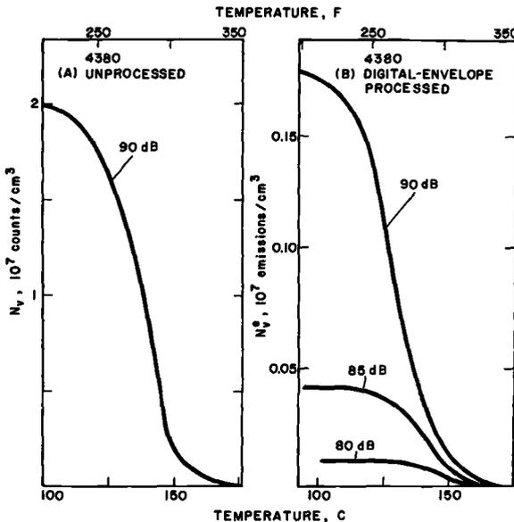
FIG. 10—Effect of digital-envelope processing and amplification on total martensite counts.
