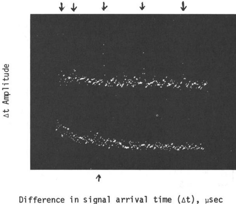
FIG. 16—Defective welds in 180 ft section of low-pressure gas line.
