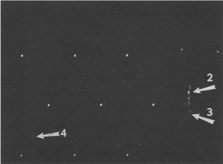
FIG. 12—CRT display of emission sources for cylindrical pressure vessel Cycle 3 (0 to 2.3  $MN/m^2$ ),
