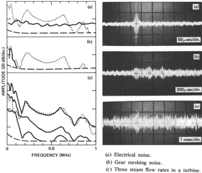
FIG. 10—Examples of background noises recorded during acoustic emission tests.
