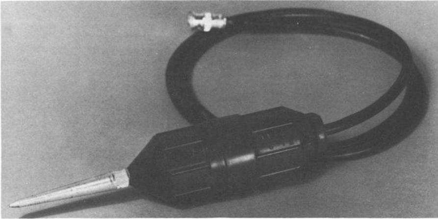
FIG. 5—Typical geophone (velocity gage) installed in marsh-type case.
