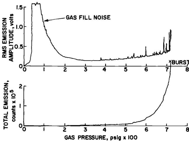
FIG. 7—Acoustic emission record of a defective pressure vessel that failed in the heat-affected zone of the waist weld at approximately 50 percent of the design burst pressure.
