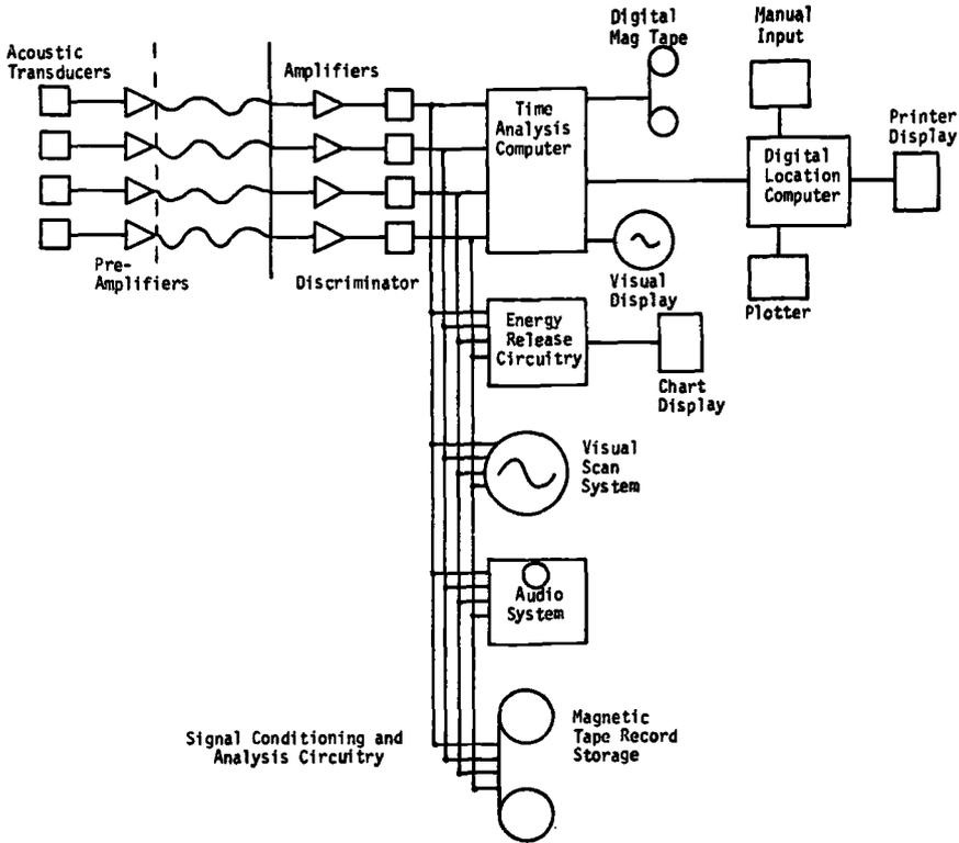
FIG. 4—Block diagram of the monitoring equipment used in the field.
