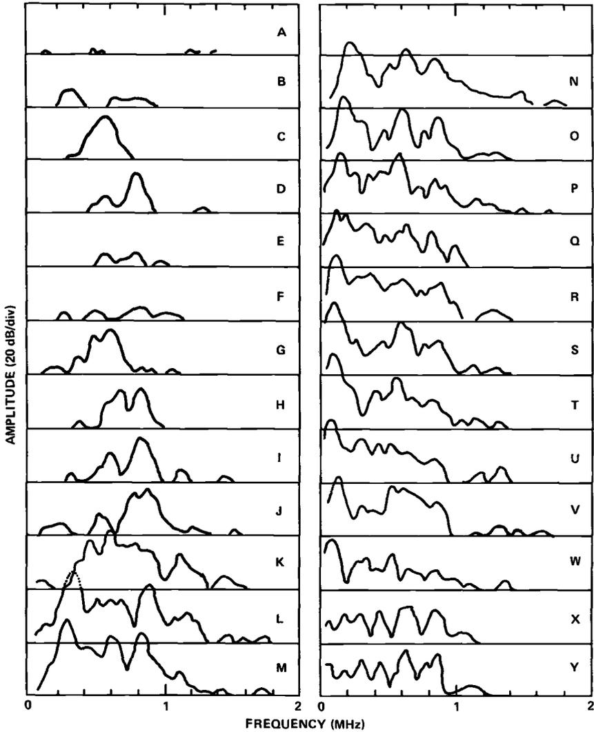
FIG. 20—Frequency analysis of successive 20  $\mu$ s increments of the acoustic burst at the bottom of Fig. 19.
