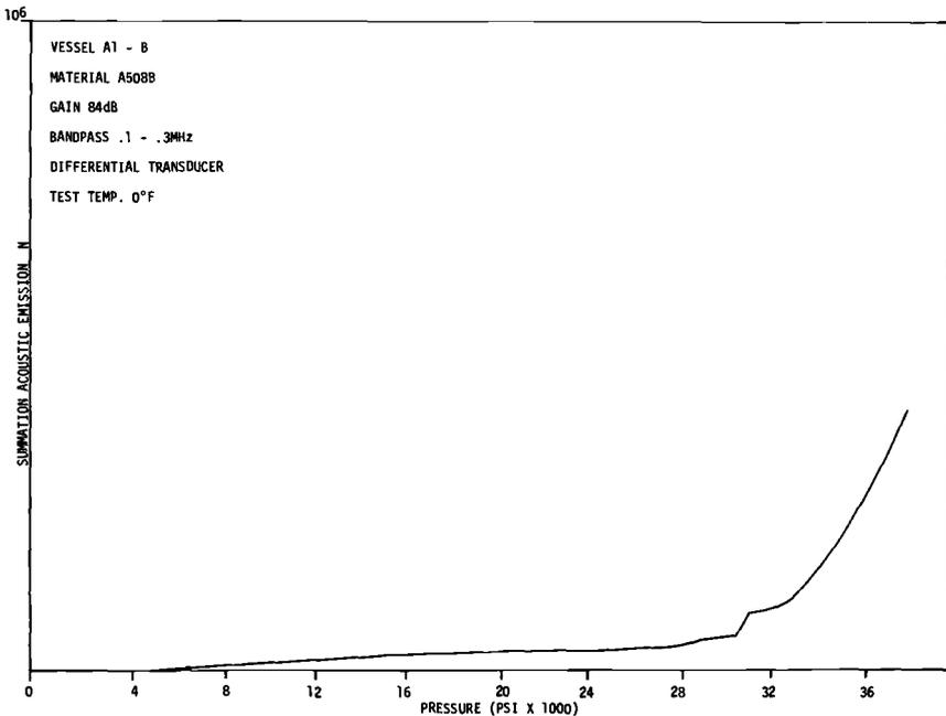
FIG. 8—Summation of acoustic emission versus pressure (composite) Vessel A1-B.
