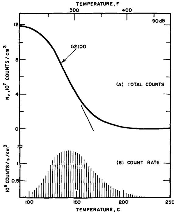
FIG. 7—Acoustic emission resulting from martensite formation in high-carbon steel.
