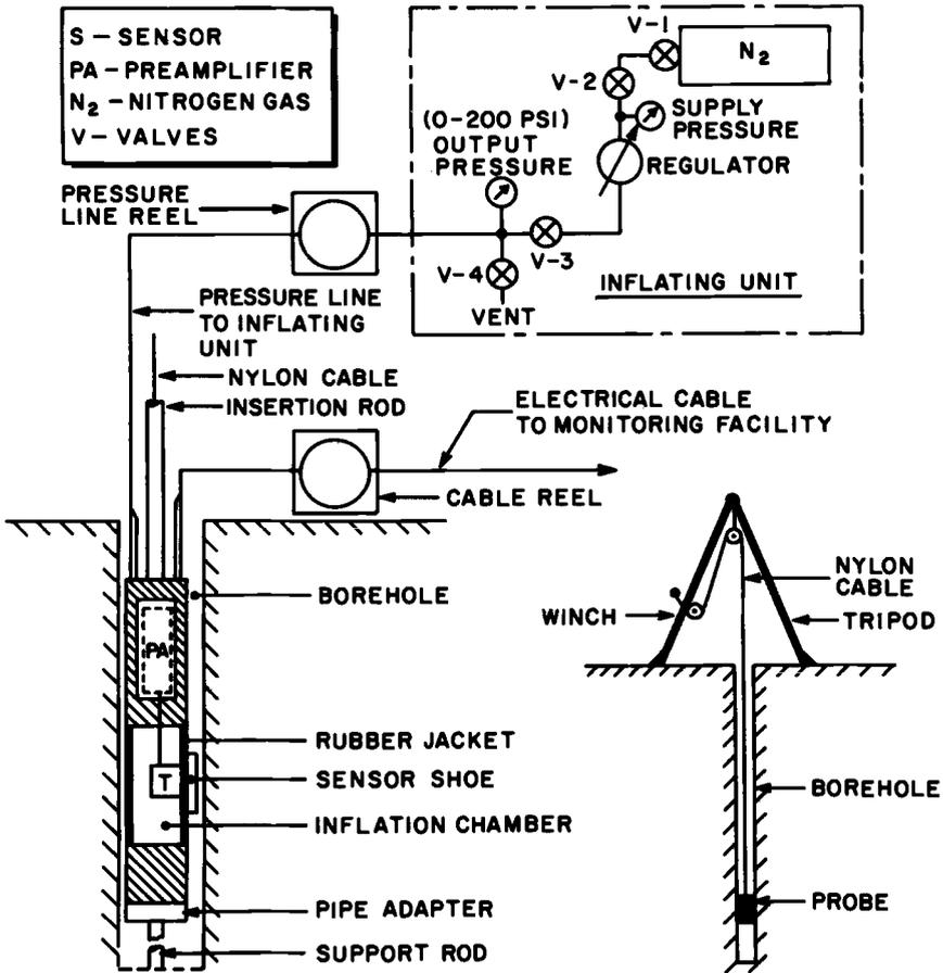
FIG. 6—Principle of operation and installation of acoustic emission probe.
