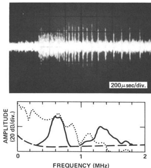
FIG. 11—Multiple acoustic bursts believed to be due to “stick-slip” friction.
