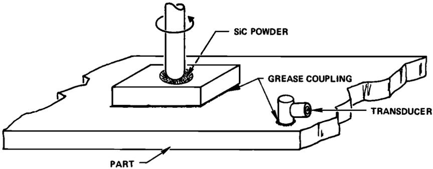
FIG. 2—Acoustic “white noise” source for determining transducer response and for acoustic attenuation measurements.
