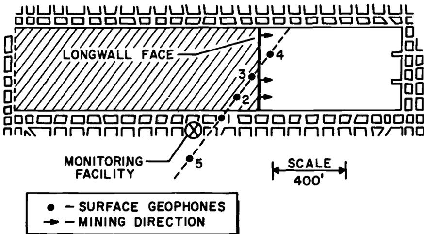
FIG. 11—Sensor array over a longwall coal mine in central Pennsylvania (distances between transducers 1 to 4 are approximately 125 ft).
