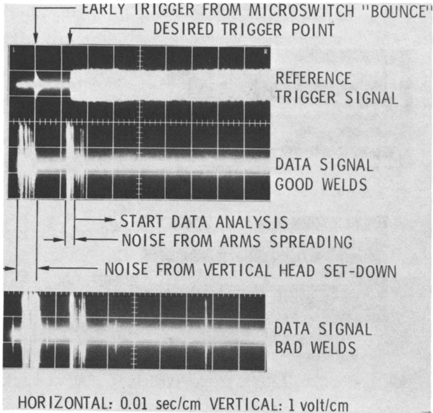
FIG. 10—Detail acoustic data from link.
