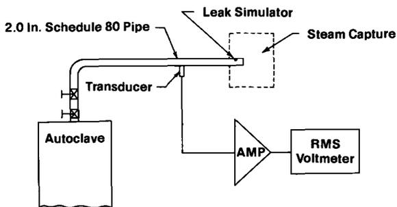
FIG. 6—Leak detection system test.
