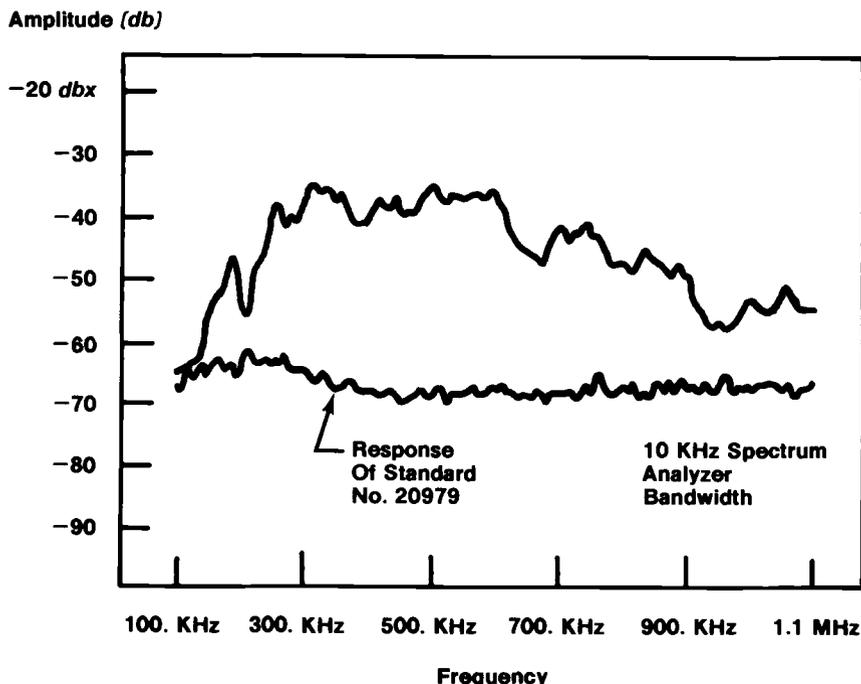
FIG. 3—Acoustic emission transducer sensitivity calibration.
