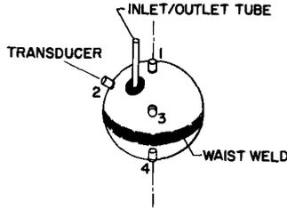
FIG. 6—Transducer array on a pressure vessel instrumented with two coincidence circuits to discriminate acoustic emissions from the tube joint area (Transducers 1, 2, and 3) and the waist weld area (Transducers 1 and 4).
