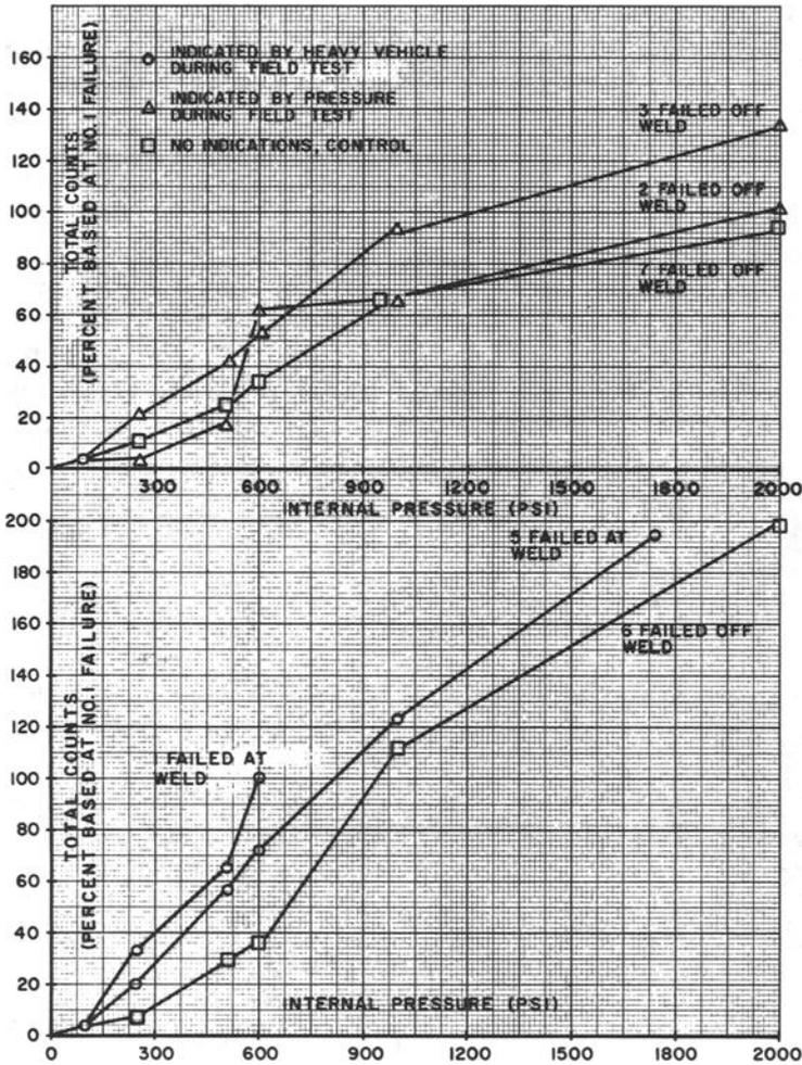
FIG. 13—Total counts as a function of pressure for specimens from Field Test 4.
