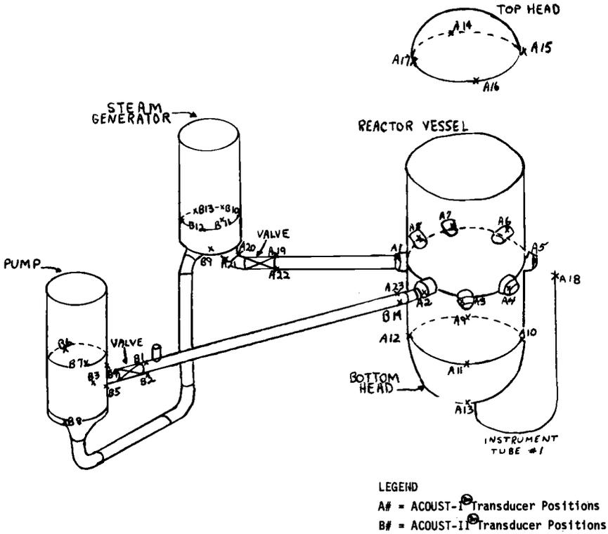
FIG. 17—Plant showing acoustic transducer locations on pumps, valves, piping, and reactor pressure vessel.
