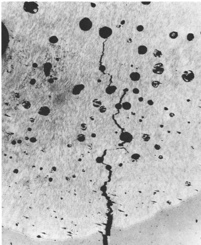
FIG. 10—Details of crack tip at the root of embrittled and porous aluminum weld in beryllium fracture Specimen 617-3 showing unfractured ligaments between pores (as polished,  $\times 100$ ).
