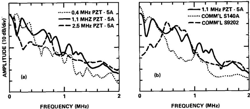
FIG. 4—Response of several piezoelectric transducers to a “white noise” source.
