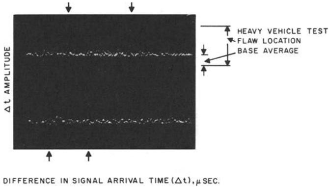
FIG. 6— $\Delta t$  amplitude data between two transducers for the heavy vehicle test during Field Test 2.
