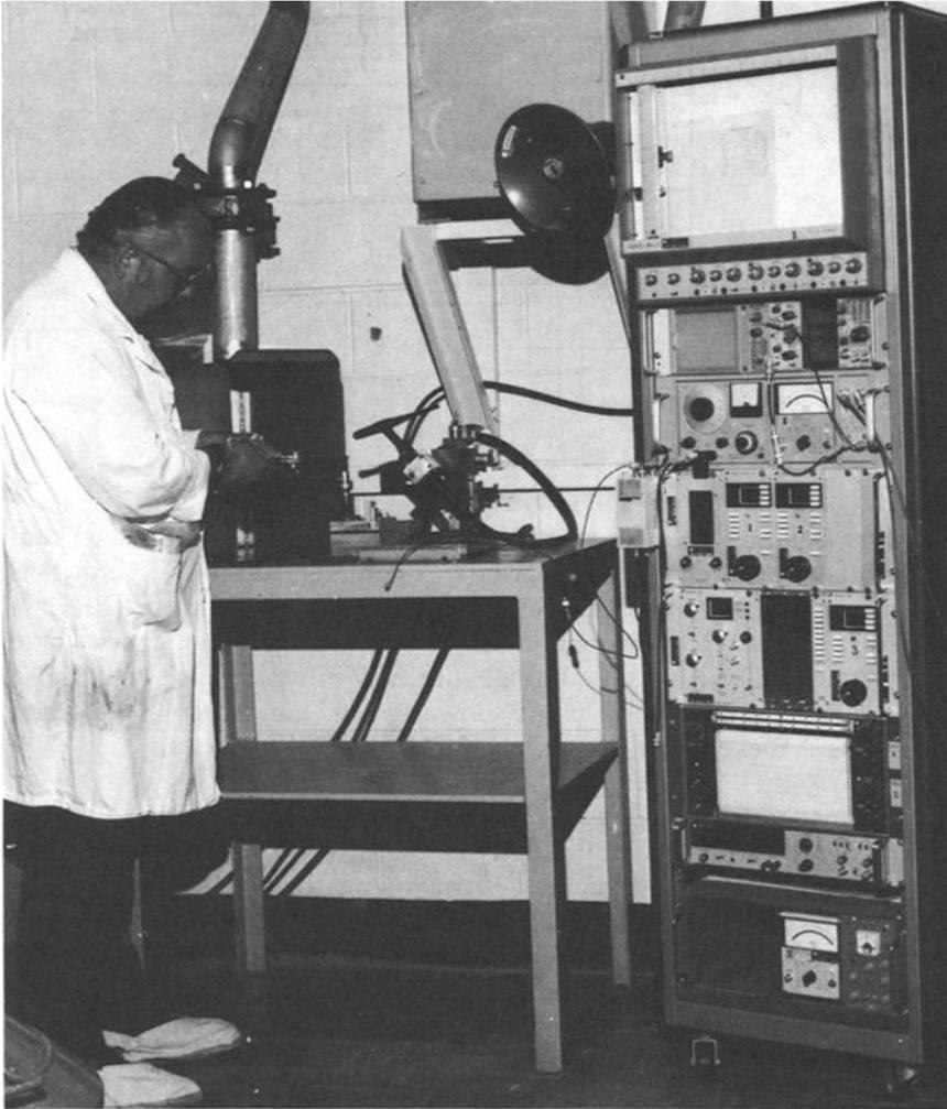
FIG. 13—Test setup and acoustic emission instrumentation used in the crack susceptibility test of beryllium coupons.
