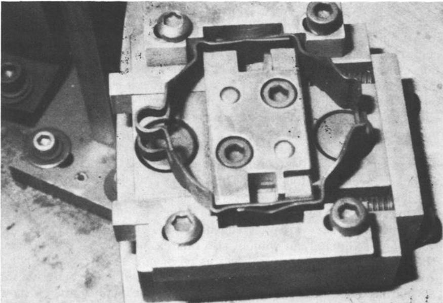
FIG. 5—Link installed for test.
