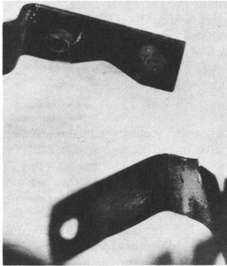
FIG. 2—Typical good and bad link welds.
