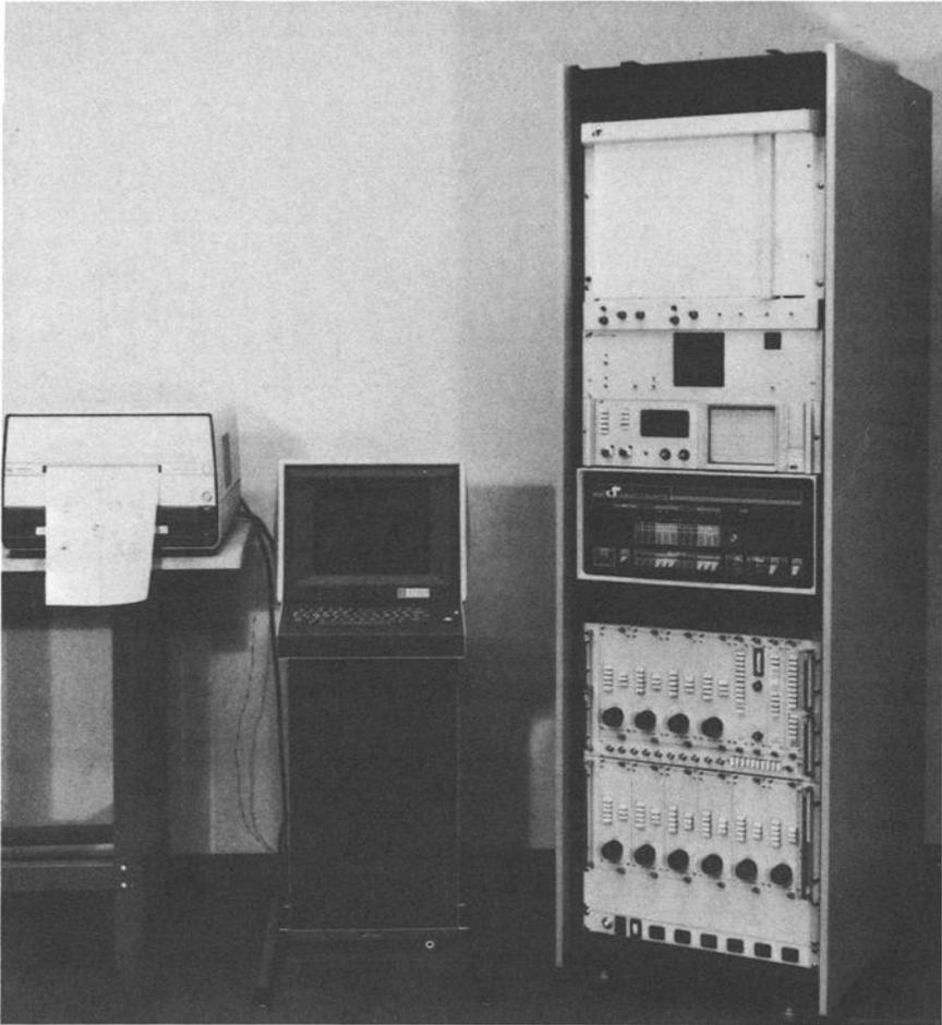
FIG. 2—Photograph of source location system.
