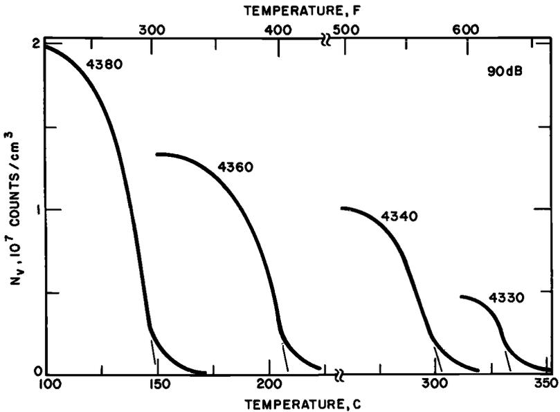
FIG. 6—Acoustic emission resulting from martensite formation in medium-carbon steels.
