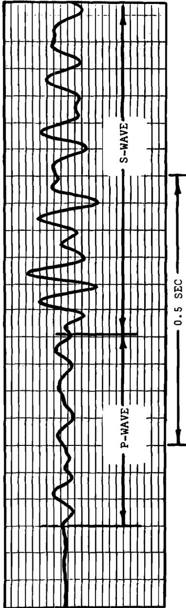
FIG. 10—Typical low frequency acoustic emission signal detected at the Michigan gas storage site (recorded using an accelerometer in a borehole probe and monitoring system bandwidth of 0 to 2.5 kHz).
