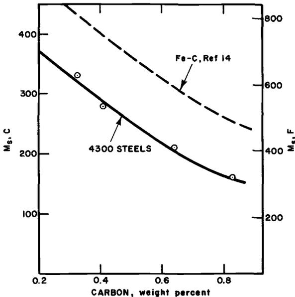
FIG. 8— $M_s$  temperatures of medium-carbon steels determined by acoustic emission.
