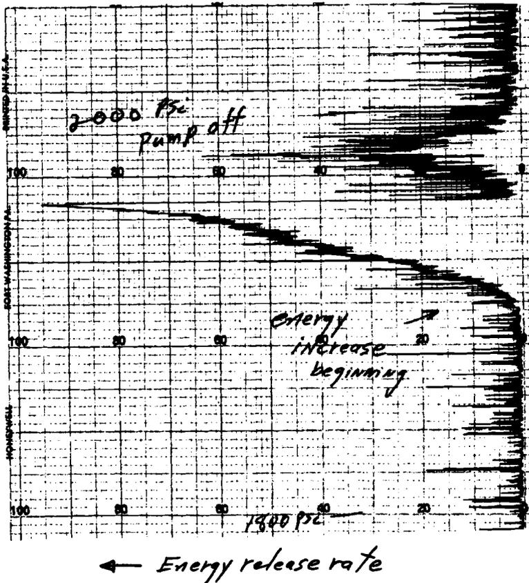
FIG. 2—Acoustic energy release pattern showing significant defect growth.
