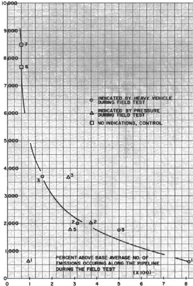
FIG. 10—Failure data for whole pipe specimens from Field Test 4.
