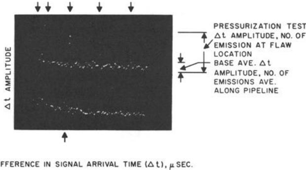
FIG. 5— $\Delta t$  amplitude data between two transducers for the pressure test during Field Test 1.
