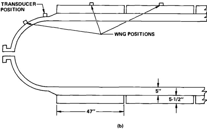
FIG. 12—Gas pressure vessels on which acoustic attenuation measurements were made.
