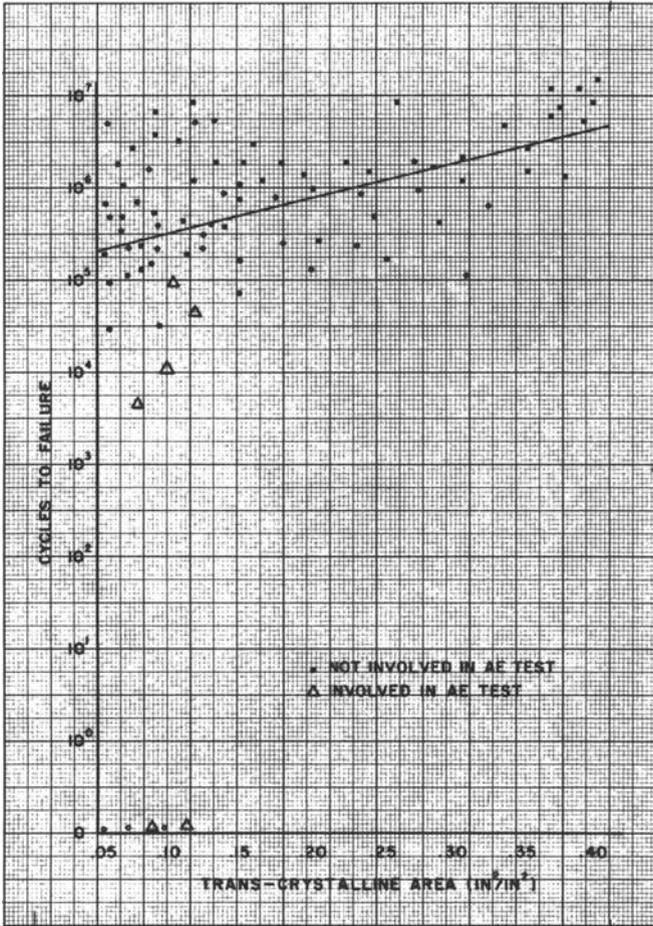
FIG. 3—Coupon fatigue test results.
