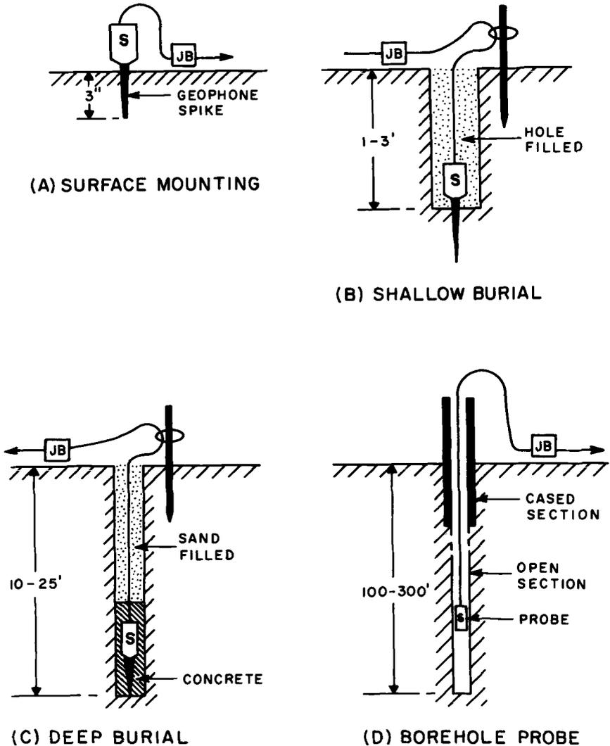
FIG. 4—Various methods of mounting acoustic emission sensors at field sites (S = sensor, PA = preamplifier, and JB = junction box).
