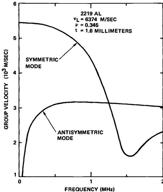
FIG. 18—Dispersion curves for Lamb waves in sheet aluminum.
