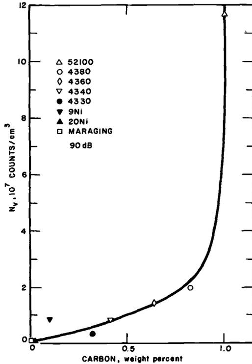
FIG. 9—Effect of carbon content on acoustic emission for formation of 100 percent martensite in steel.
