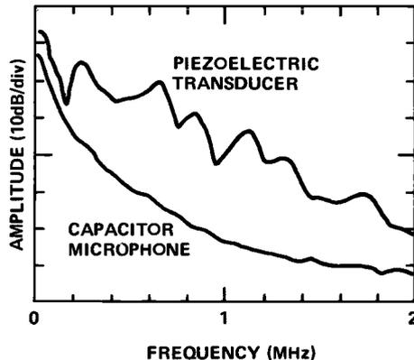
FIG. 3—Response of two types of transducers to a “white noise” source.
