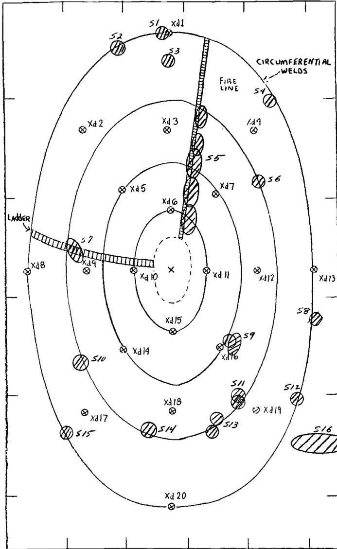
FIG. 13—Minor discontinuities in Hortonspheroid sphere storage tank.
