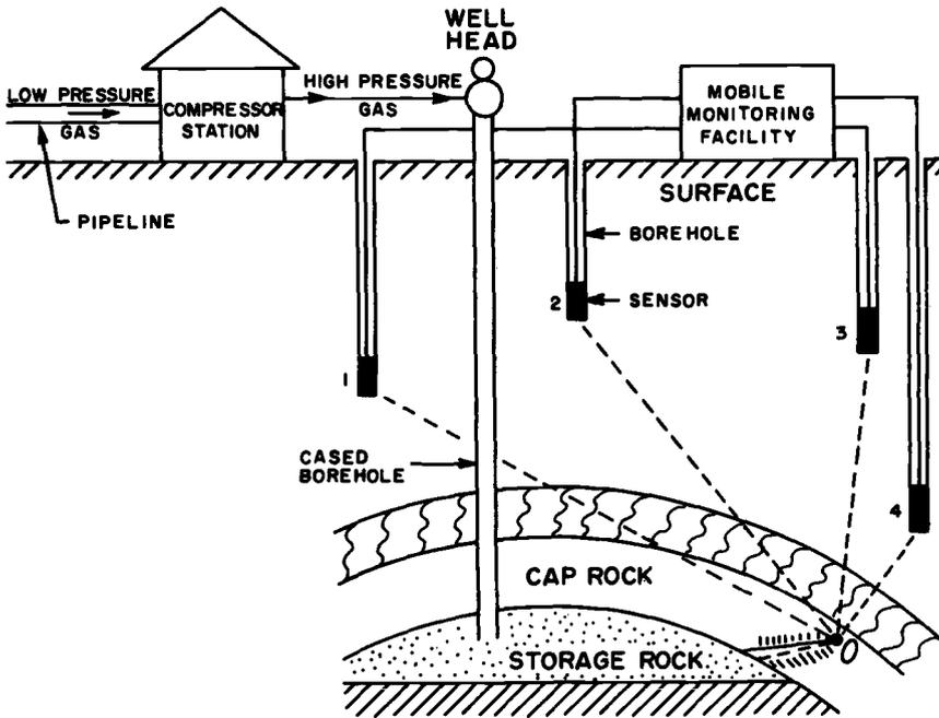
FIG. 9—Instrumented gas storage field site.
