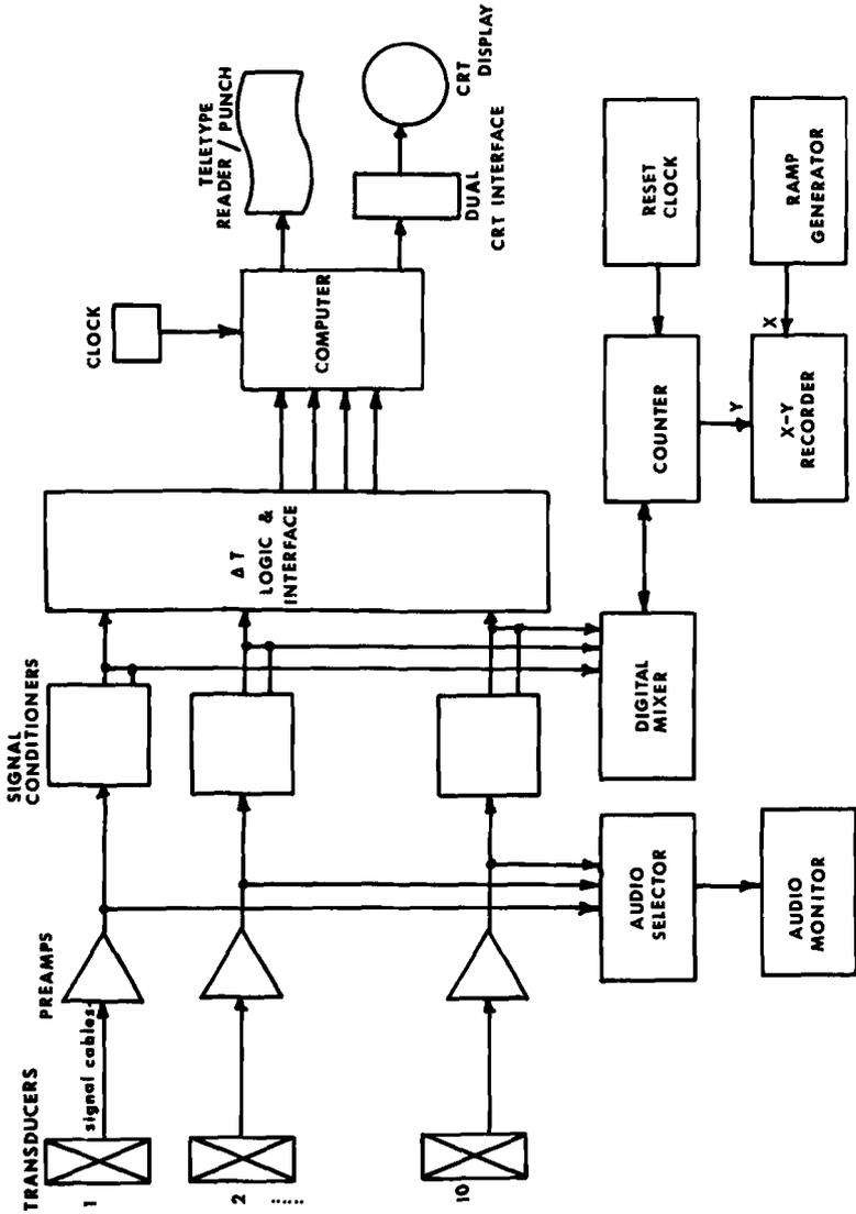
FIG. 1—Block diagram of computerized location system.
