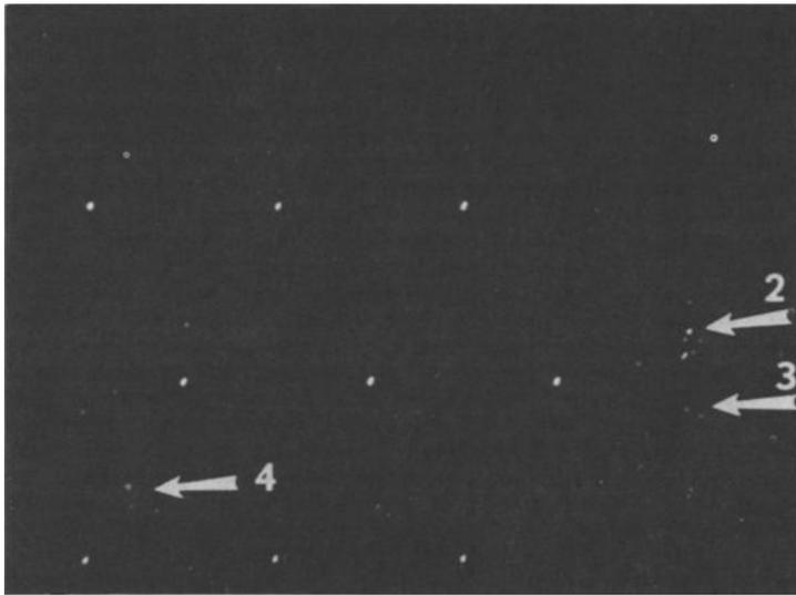
FIG. 14—CRT display of emission sources for KEMA pressure Cycle 3 (2.8 to 3.7 MN/m<sup>2</sup>).
