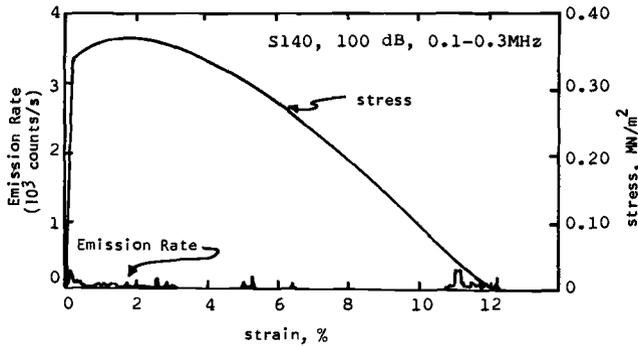
FIG. 21—Acoustic emission stress strain plot for fatigue precracked specimen of AMMO steel.
