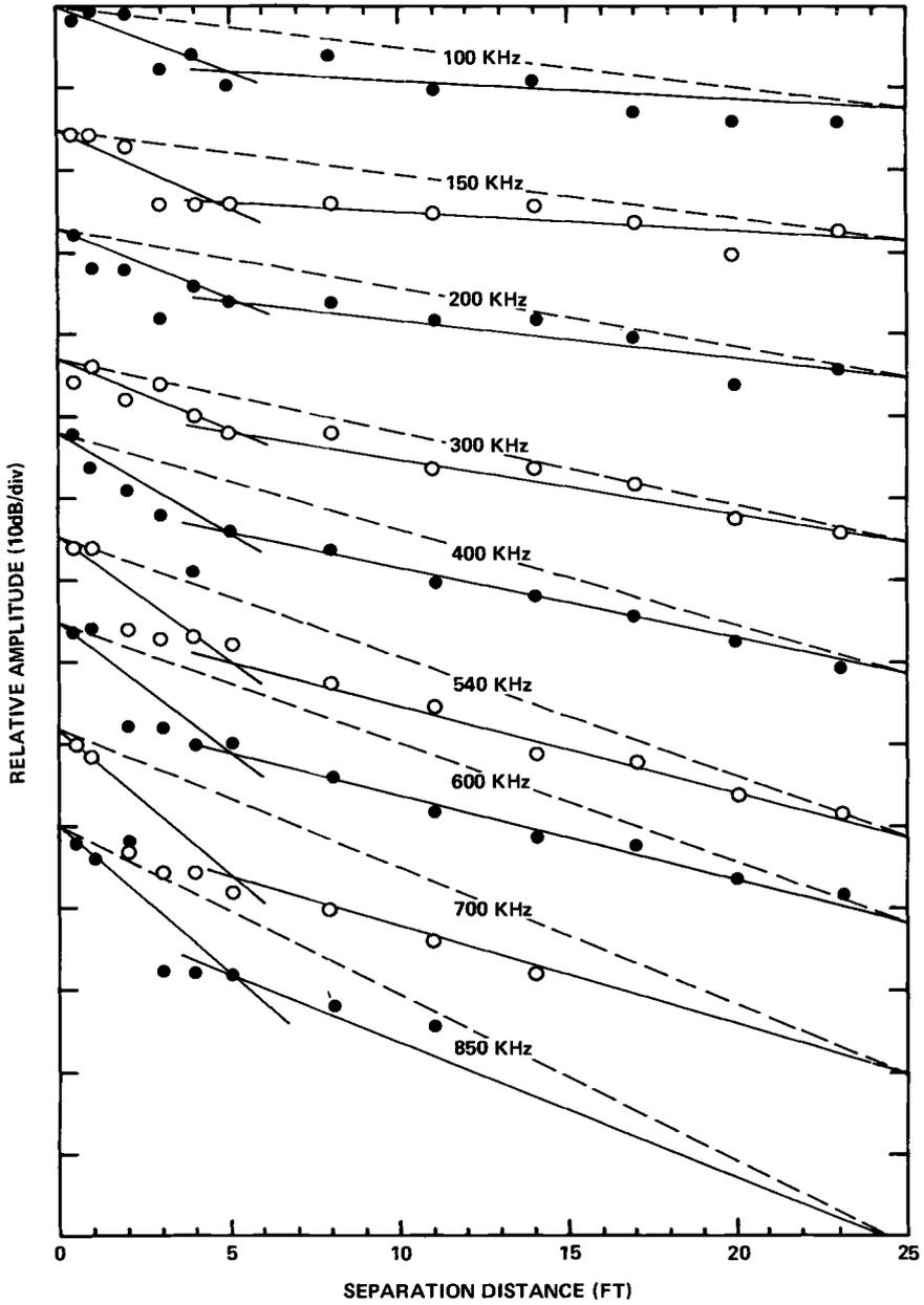
FIG. 13—Signal loss as a function of distance and frequency along the outer surface of the gas pressure vessel of Fig. 12a.
