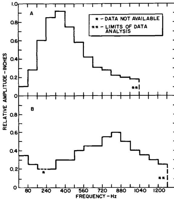
FIG. 14—Frequency spectra of typical acoustic emission signal (A) and background (B).
