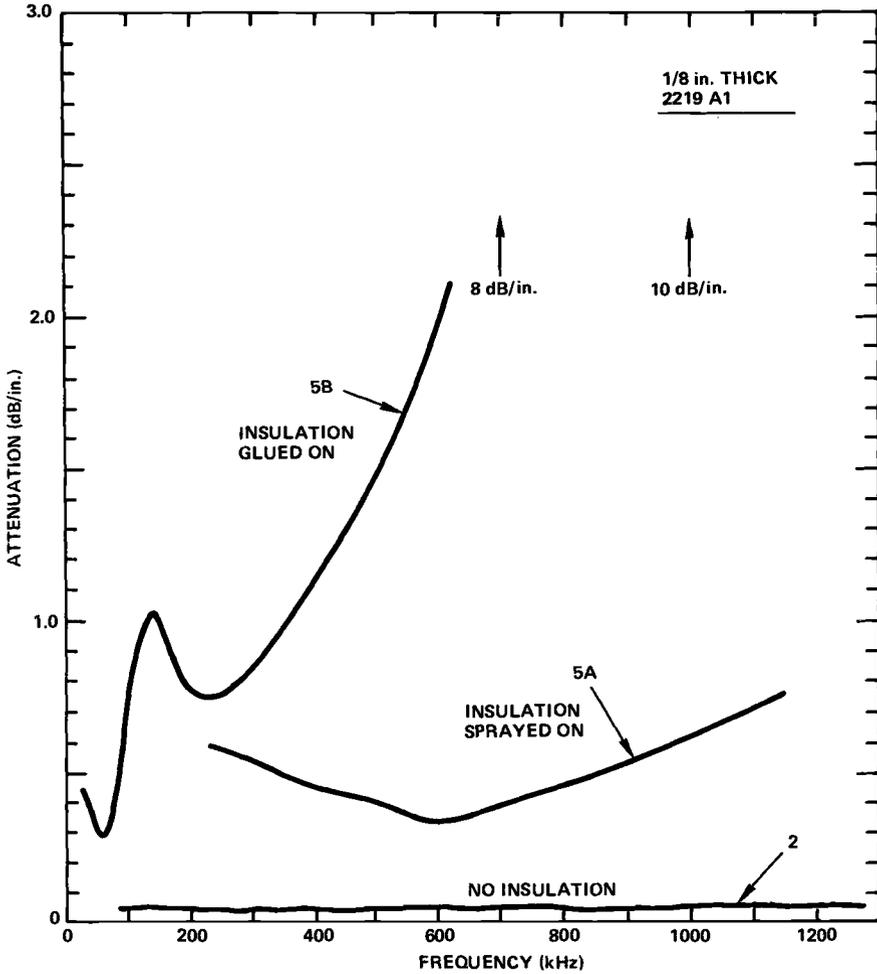
FIG. 16—Acoustic attenuation of aluminum sheet having a foam insulation material on its reverse side.
