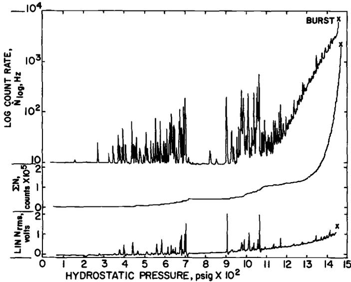
FIG. 4—Comparison of linear root mean square voltage, total emission, and log count rate as a function of pressure for a pressure vessel taken to burst at 1470 psig (Run 561).
