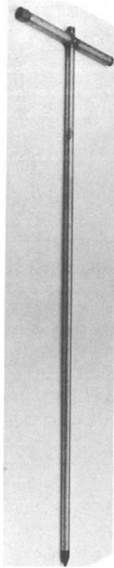
FIG. 14—*Special pipeline acoustic probe.*
