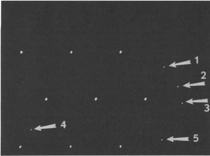
FIG. 9—CRT display of location of simulated emission introduced at the defects in the cylindrical vessel.
