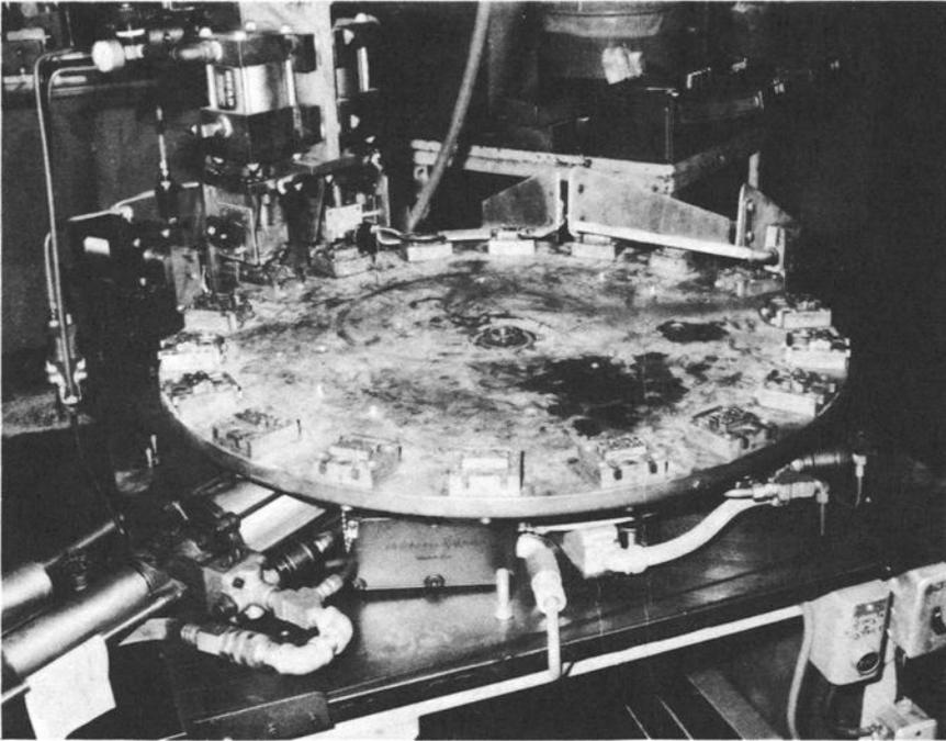
FIG. 3—Proof test machine 40-mm ammunition links.
