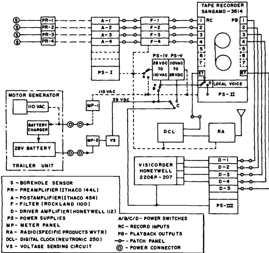
FIG. 1—Block diagram of Penn State acoustic emission field monitoring facility.
