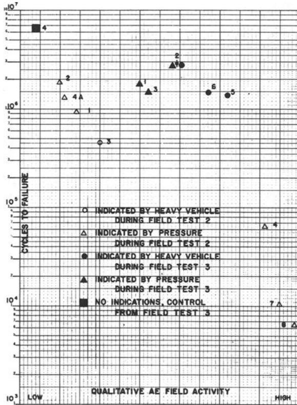
FIG. 7—Fatigue data for whole pipe specimens from Field Test 2 and Field Test 3.
