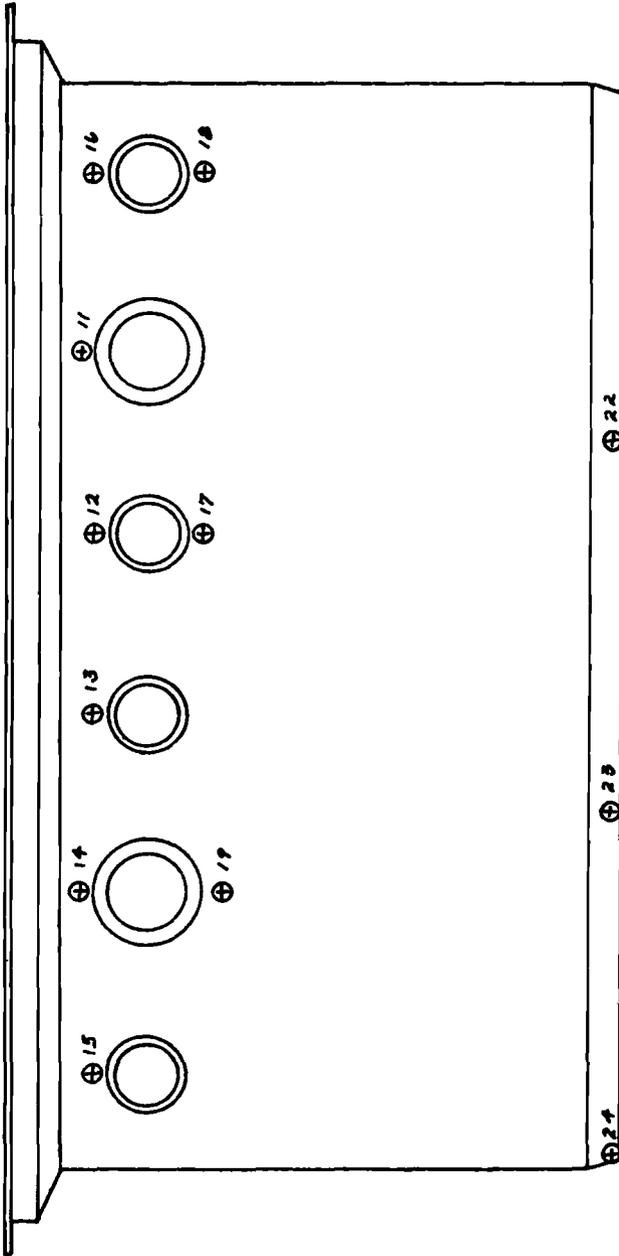
FIG. 18—Reactor pressure vessel transducer locations.
