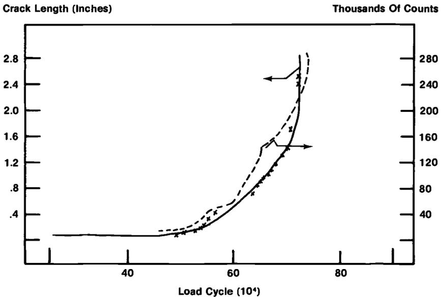
FIG. 10—Crack length and gated counts versus cycles for 4-in. specimen.
