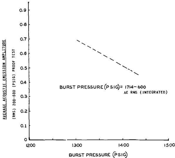
FIG. 1—Integrated acoustic emission amplitude versus chamber burst pressure.
