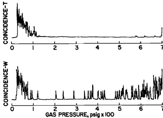
FIG. 8—Coincidence plots of acoustic emission activity in the waist weld area (W) and in the inlet/outlet tube joint area (T) during pressurization to failure of a defective pressure vessel (acoustic emission from burst test plotted in Fig. 7).
