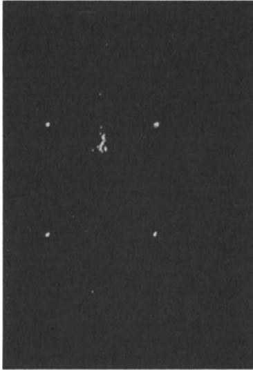
FIG. 3—Location results for punch test on honeycomb. Results for entire test to destruction (Test 1) are shown. Transducers and punch on same side of panel.
