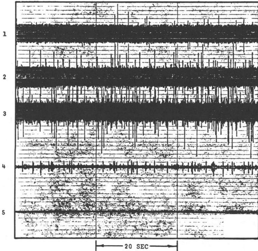
FIG. 12—Acoustic emission signals detected during a 60 s period over a longwall coal mine (recorded using geophones (velocity gages) and monitoring system bandwidth 0 to 2.5 kHz).
