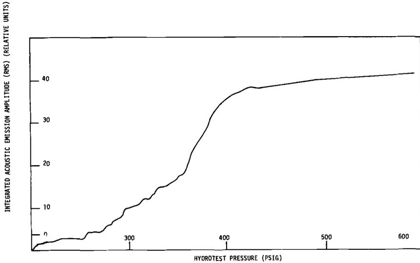
FIG. 2—Integrated acoustic emission amplitude versus hydrotest pressure.
