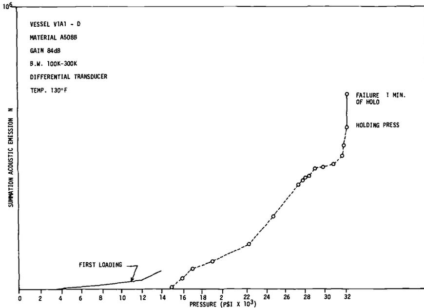
FIG. 9—Summation of acoustic emission versus pressure (composite) Vessel A1-D.
