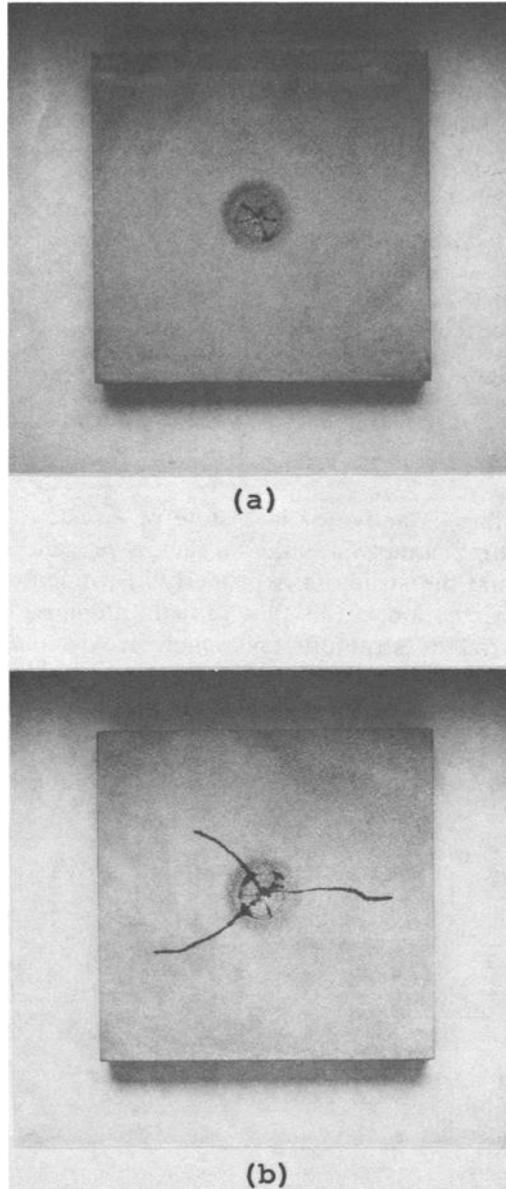
FIG. 15—Beryllium weld test coupons showing crater cracking in Specimen WT-70 (a) and gross cracking in Specimen WT-71 (b).
