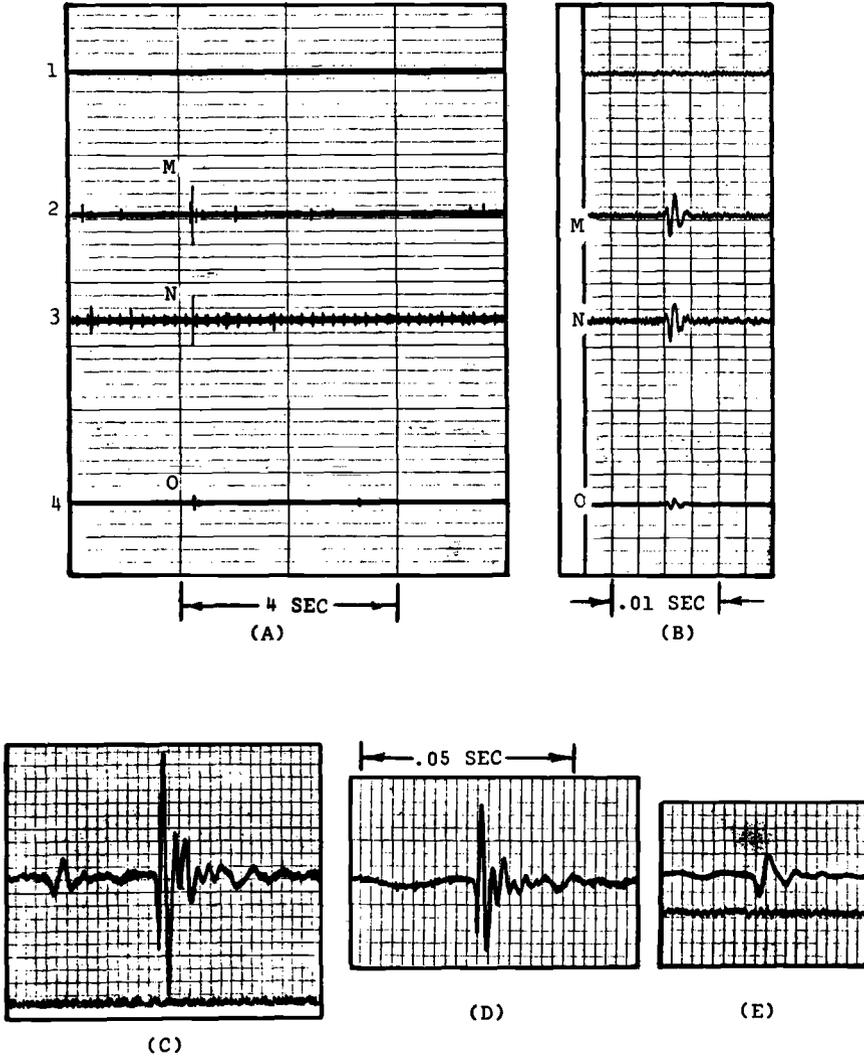
FIG. 13—Typical acoustic emission signals observed over a longwall coal mine (recorded using geophones (velocity gages) and monitoring system bandwidth 0 to 2.5 kHz).
