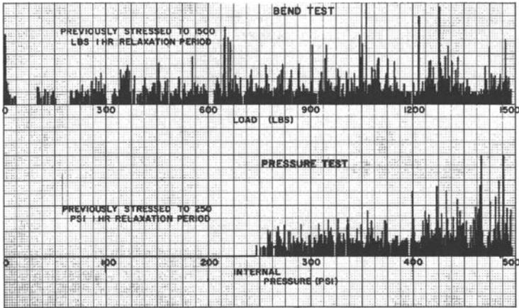
FIG. 14—Comparison of the Kaiser effect for two different types of stressing.
