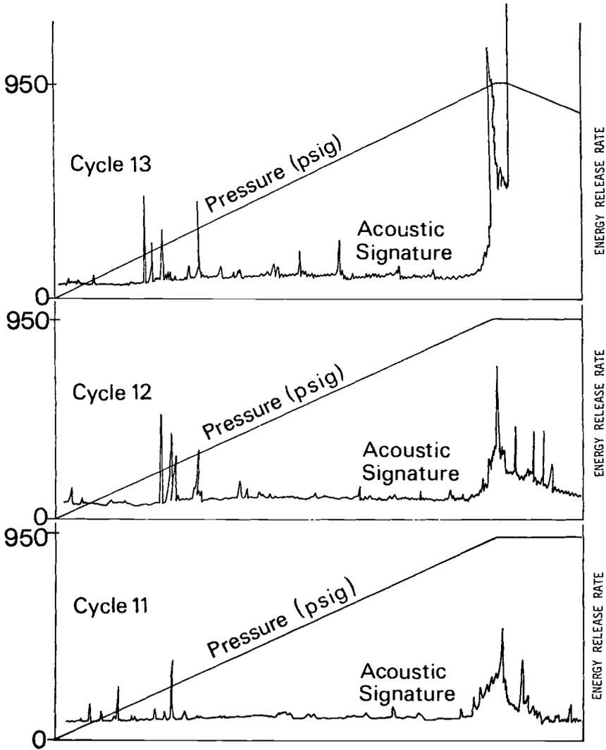
FIG. 10—Acoustic signature of cyclic failure.
