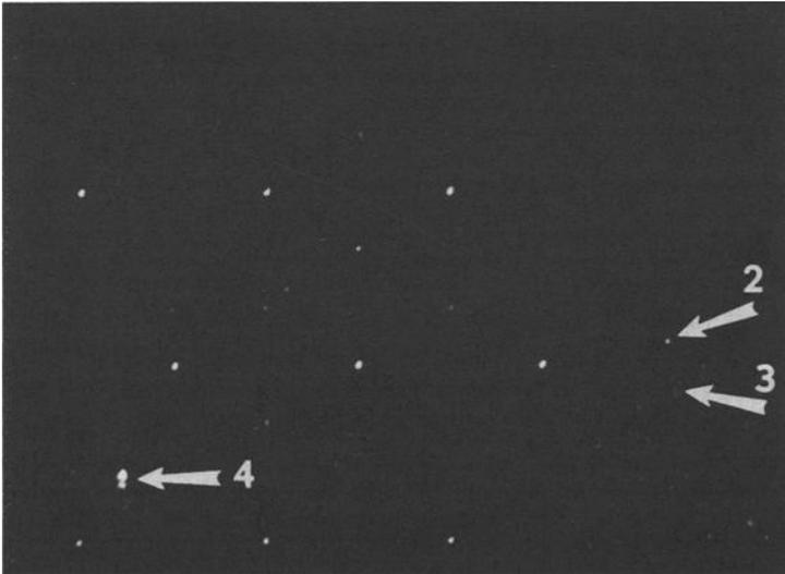
FIG. 13—CRT display of emission sources for KEMA pressure Cycle 3 (2.3 to 2.8  $MN/m^2$ ).
