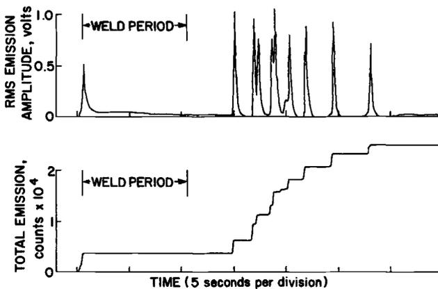
FIG. 17—Acoustic emission record of gross cracking in beryllium weld Specimen WT-71.
