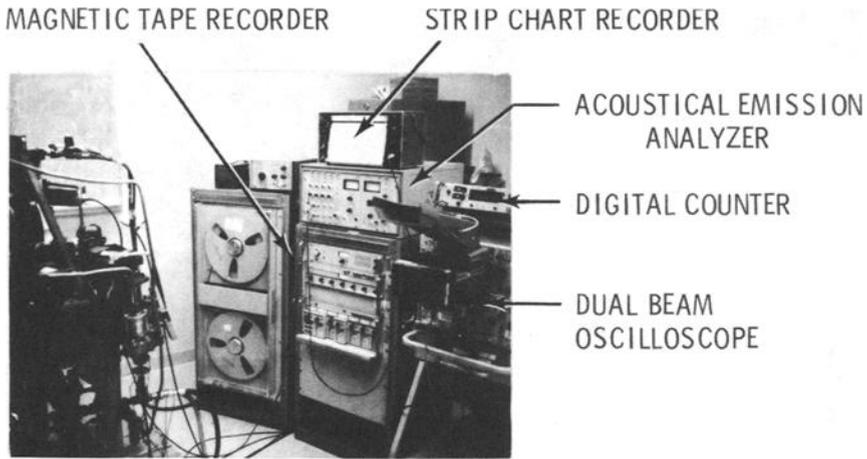
FIG. 7—Instrument system to analyze acoustic emission.
