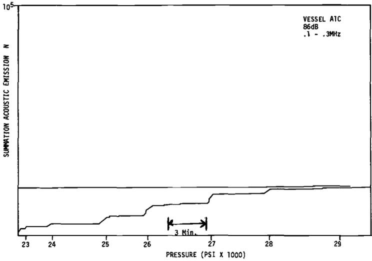
FIG. 7b—Summation of acoustic emission versus pressure 23 to 29 000 psi Vessel A1-C.
