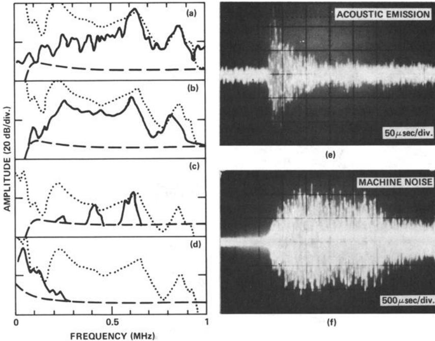
FIG. 8—Examples of acoustic emission and machine noise produced during fatigue of a 2024 aluminum specimen.
