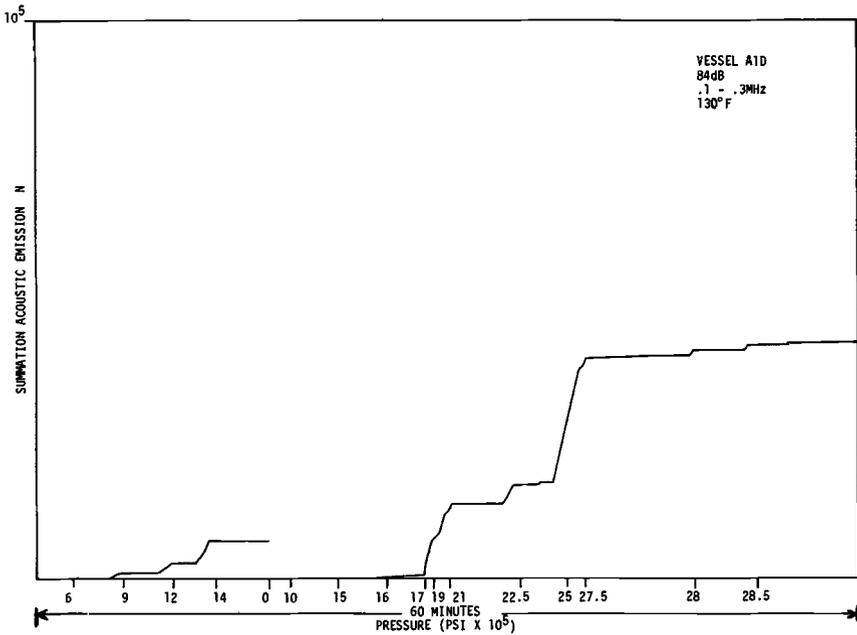
FIG. 10a—Summation of acoustic emission versus pressure 0 to 28 5000 psi Vessel A1-D.
