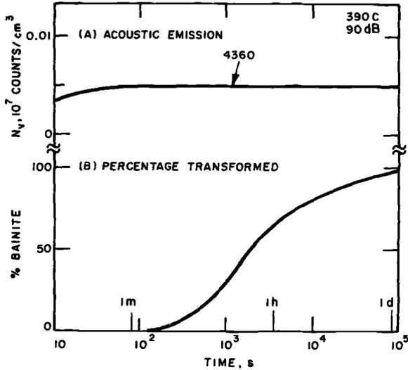
FIG. 4—Absence of acoustic emission during bainite formation in steel.
