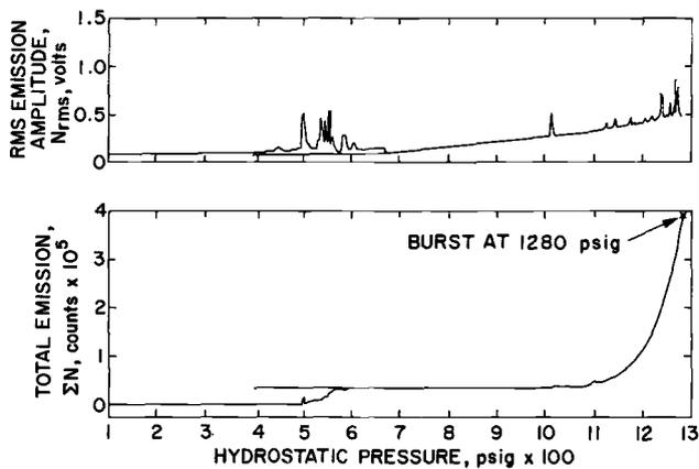
FIG. 2—Typical acoustic emission of a pressure vessel that failed in base metal.
