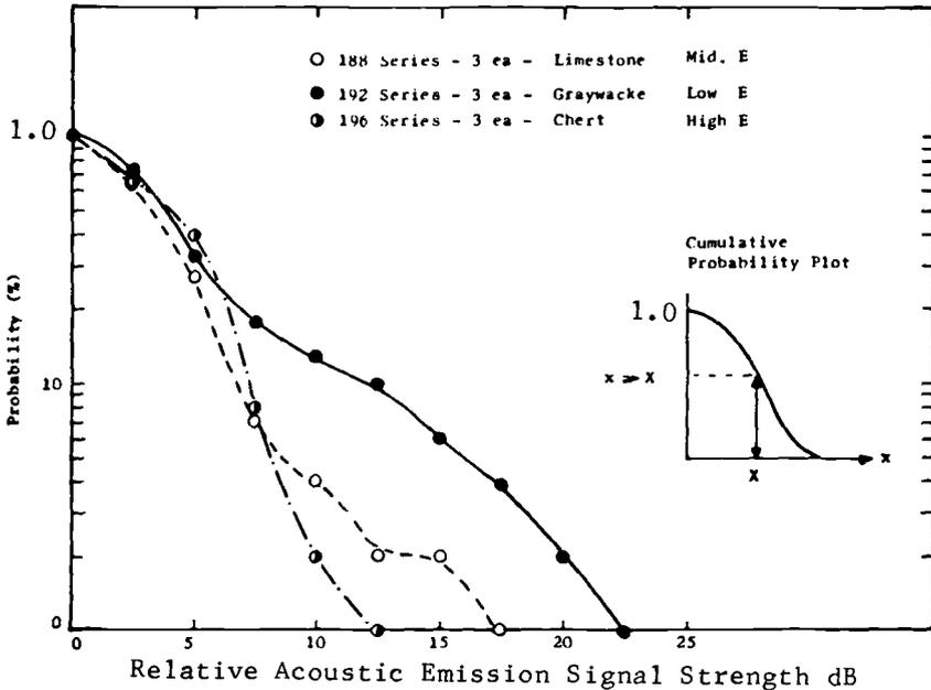
FIG. 11—Probability of  $x > X$  versus relative AE signal strength.
