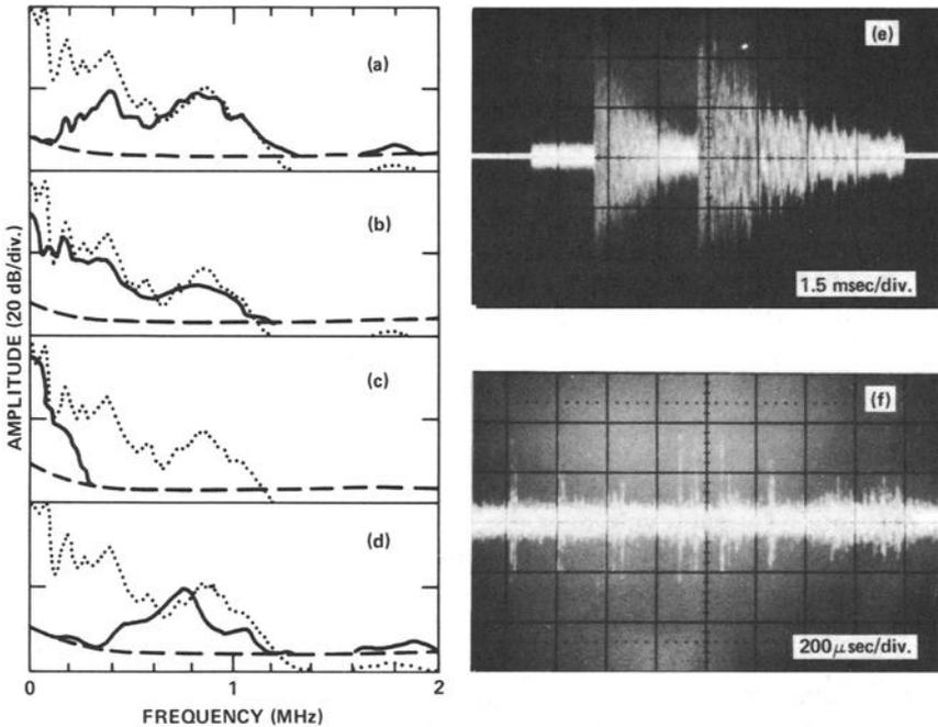
FIG. 6—Examples of distinctive acoustic emissions generated in A533-B low-alloy pressure vessel steel.
