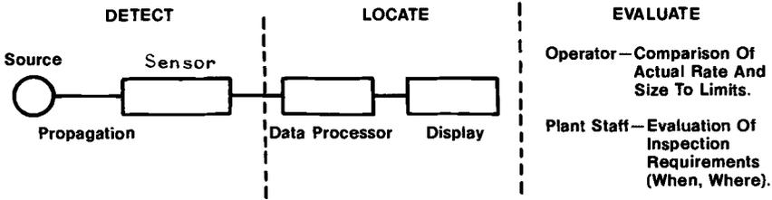
FIG. 1—Various phases of acoustic emission technology.
