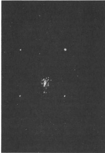
FIG. 4—Location results for punch test on honeycomb. Results for entire test to destruction (Test 2) are shown. Transducers and punch on opposite sides of panel.
