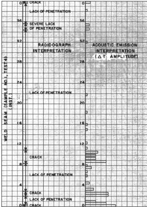
FIG. 12—Comparison between radiograph indications and acoustic emission indications.
