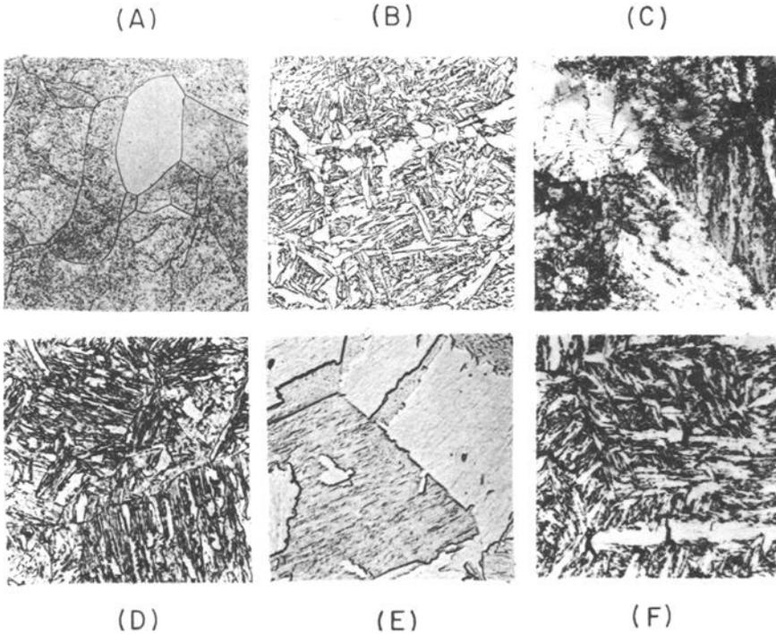
FIG. 12—Microstructures of acoustic emission specimens: (a) iron, (b) line-pipe steel, (c) Fe-0.9C, (d) 9Ni steel, (e) maraging steel, and (f) AISI 52100 steel. (a), (b)  $\times 500$ ; (c) to (f)  $\times 750$ .
