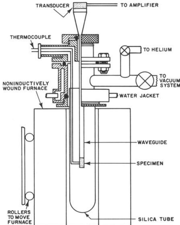
FIG. 1—Furnace for acoustic emission studies at high temperatures.
