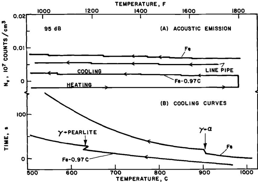
FIG. 3—Absence of acoustic emission during ferrite and pearlite formation in steel.
