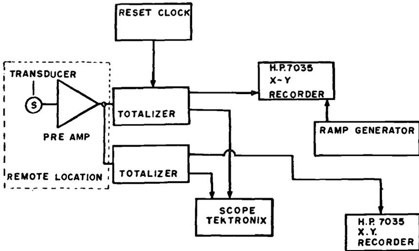
FIG. 5—Acoustic emission system block diagram.
