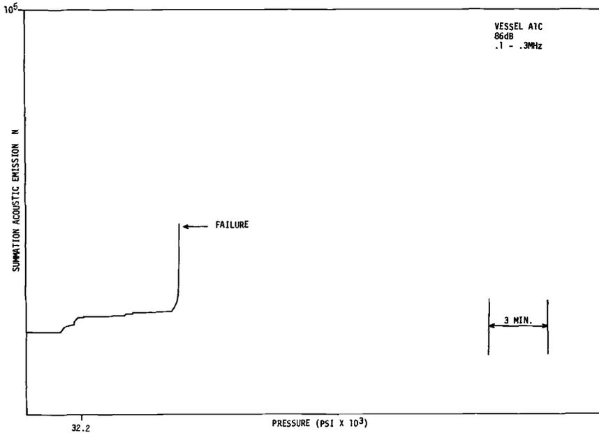
FIG. 7c—Summation of acoustic emission versus pressure 32 200 psi to failure Vessel A1-C.
