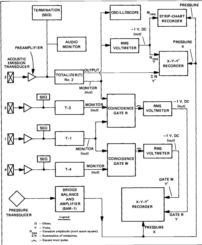
FIG. 5—Block diagram of acoustic emission system with two coincidence gates.
