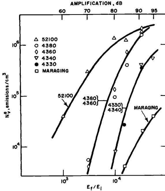
FIG. 11—Effect of amplification on digital-envelope-processed counts for formation of 100 percent martensite in various steels.
