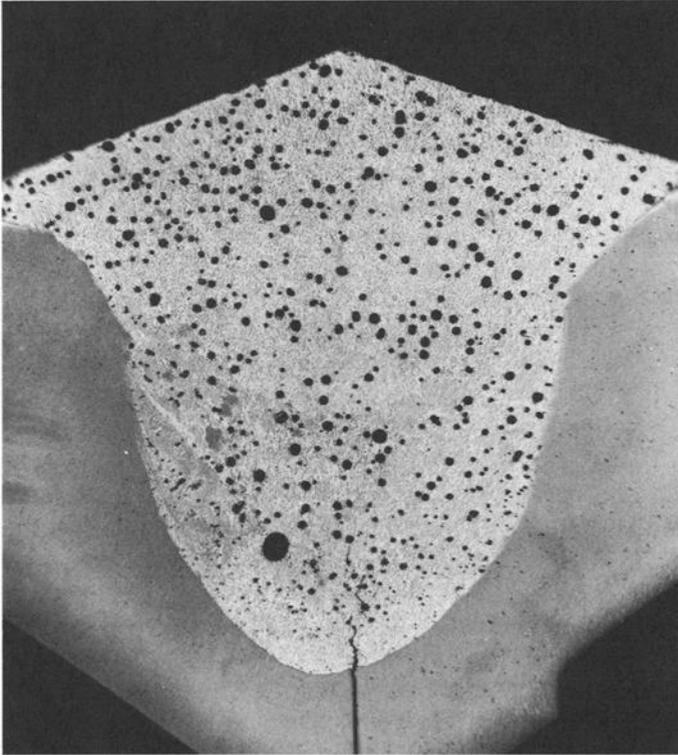
FIG. 9—Cross section of weld joint in beryllium fracture Specimen 617-3 showing excessive porosity and root crack in the aluminum weld deposit (as polished,  $\times 20$ ).
