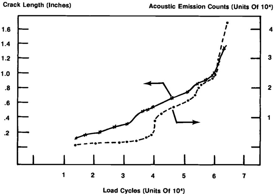
FIG. 11—Crack length and gated counts versus cycles for 2-in. specimen.
