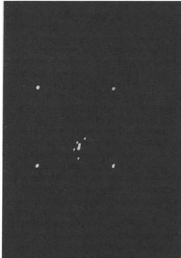
FIG. 6—Emission from honeycomb panel just prior to load drop in Test 2.
