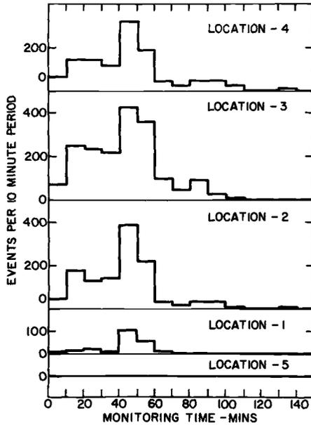
FIG. 15—Rate of acoustic emission activity at different sensor locations during test period.
