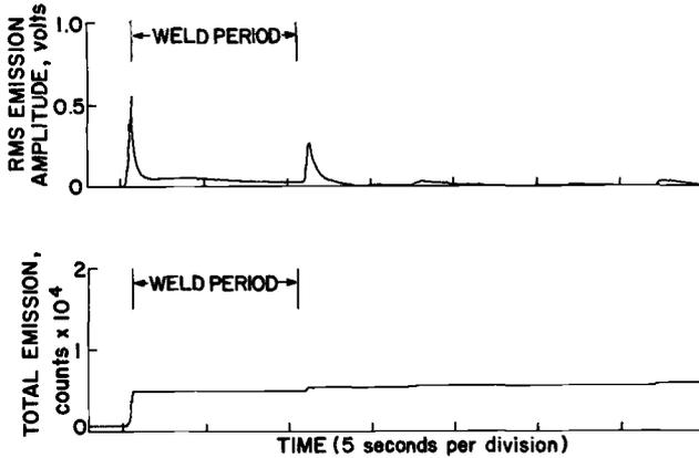
FIG. 16—Acoustic emission record of crater cracking in beryllium weld Specimen WT-70.
