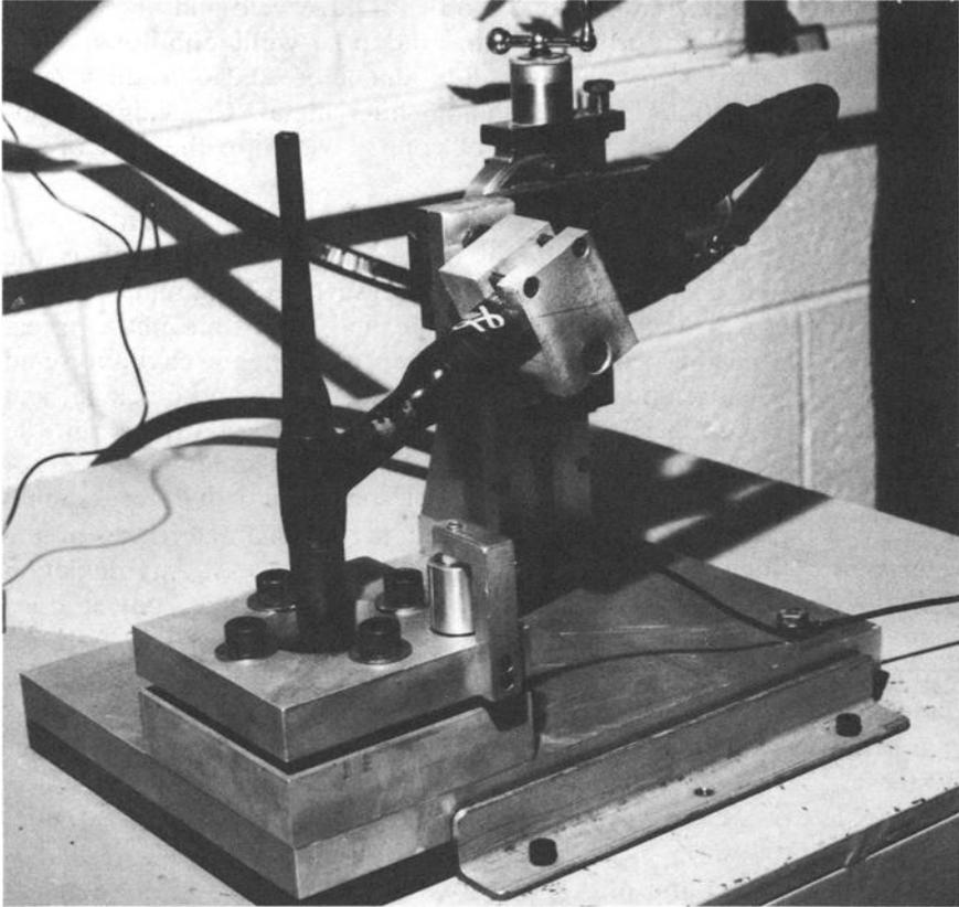
FIG. 12—Clamping fixture used to hold beryllium coupon in determining crack susceptibility by the acoustic emission produced as a result of a thermal shock. The GTA welding torch and acoustic emission sensor are shown in place.
