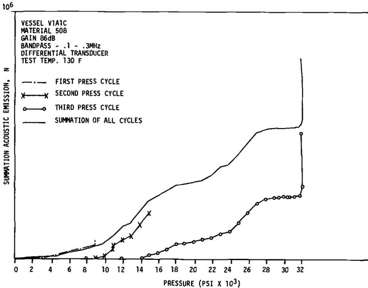
FIG. 6—Summation of acoustic emission versus pressure (composite) Vessel A1-C.
