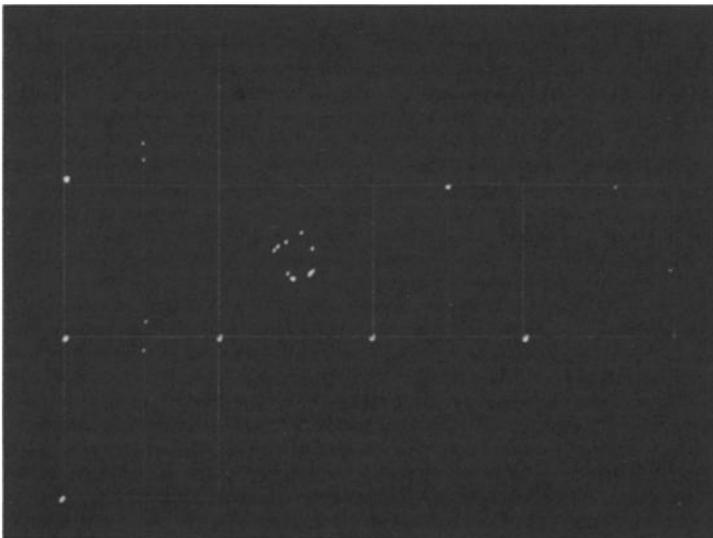
FIG. 18—*CRT display of emission sources for spherical pressure vessel Cycle 1.*
