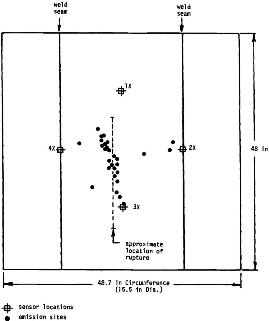
FIG. 1—Emission sources located during hydrotest of vessel.
