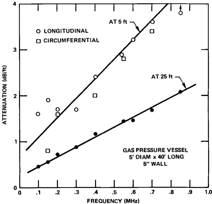
FIG. 14—Acoustic attenuation in the gas pressure vessel of Fig. 12a.
