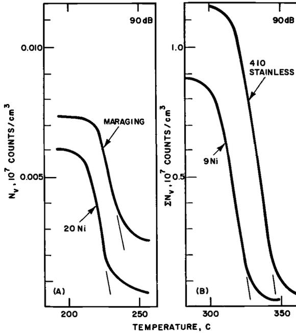
FIG. 5—Acoustic emission resulting from martensite formation in low-carbon steels.
