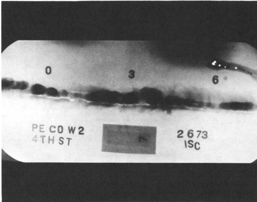
(b) Weld containing existing crack as found in the field.
