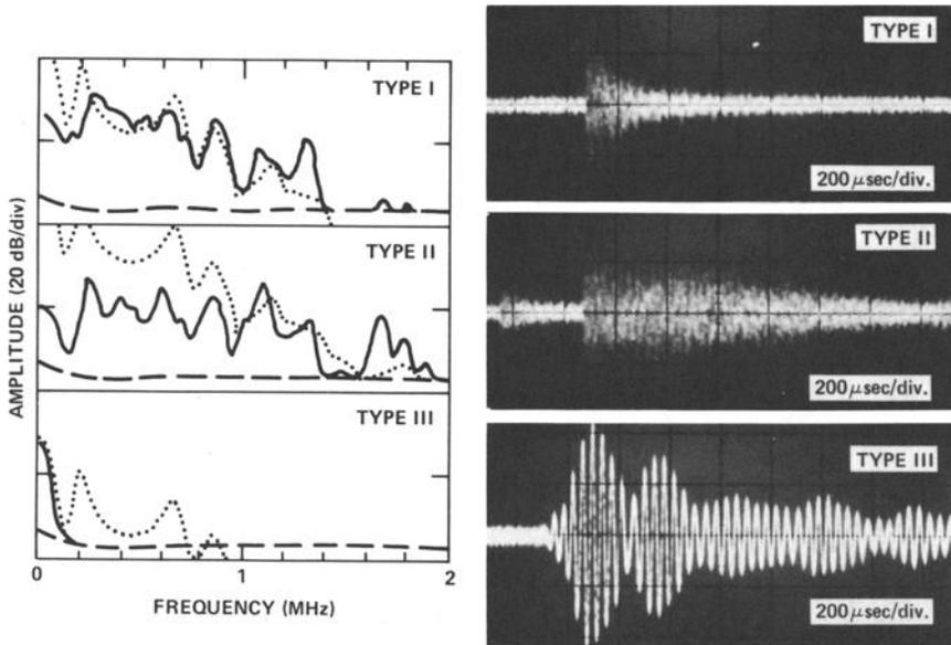
FIG. 9—Examples of acoustic bursts observed during slow crack growth in polycrystalline alumina ceramic.
