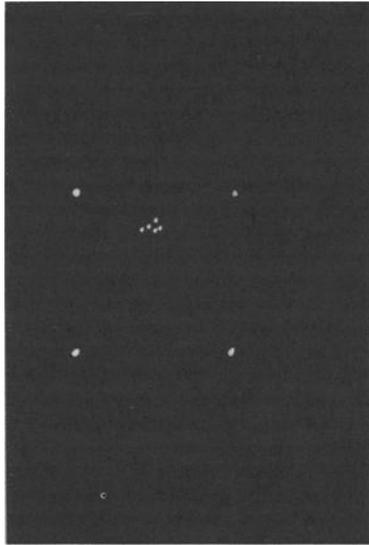
FIG. 5—Emission from honeycomb panel just prior to load drop in Test 1.
