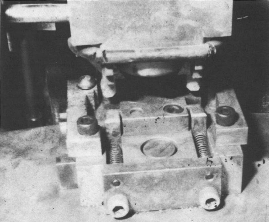
FIG. 4—Link test fixture.
