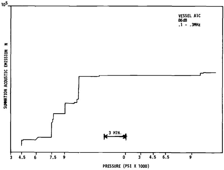
FIG. 7a—Summation of acoustic emission versus pressure to 9000 psi Vessel A1-C.
