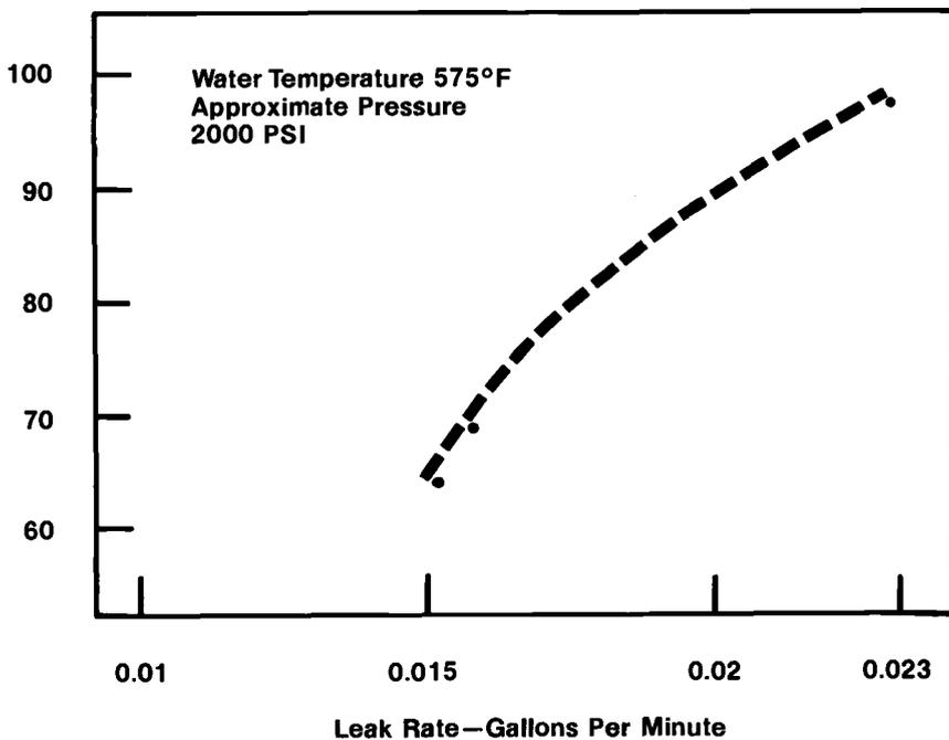
FIG. 7—Acoustic signal level at various leak rates.
