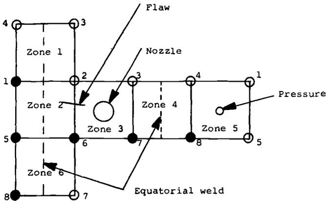
FIG. 16—CRT presentation of sphere with flaw, nozzle, and weld.
