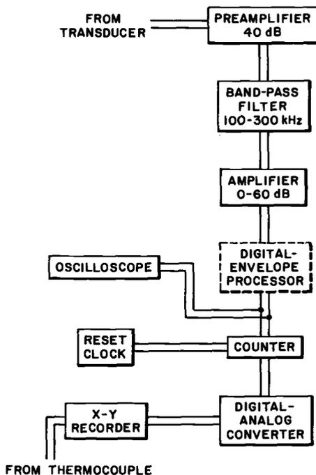
FIG. 2—Block diagram of electronic components.
