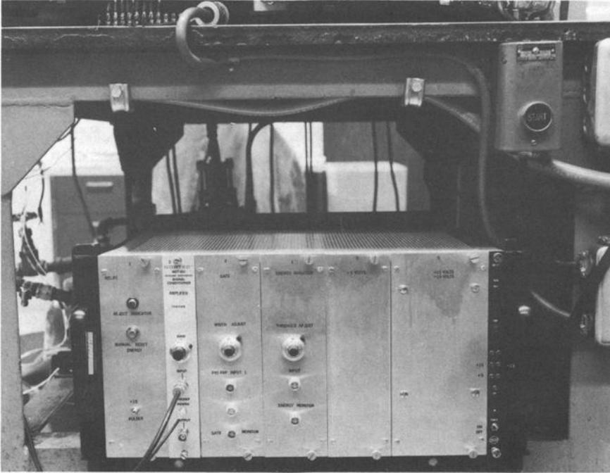
FIG. 13—*Prototype acoustic emission monitor for link welds.*
