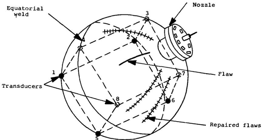
FIG. 15—Position of flaw and transducers in Saclay vessel.
