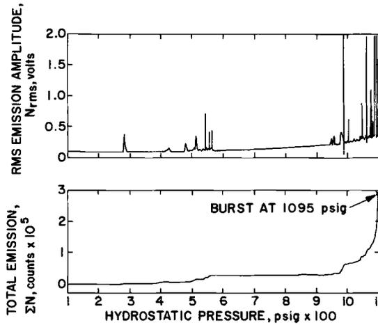
FIG. 3—Typical acoustic emission record of a pressure vessel that failed in the heat-affected zone of the waist weld.
