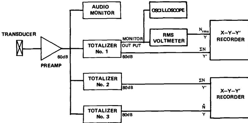
FIG. 14—Block diagram of acoustic emission system used to determine crack susceptibility of beryllium coupons.
