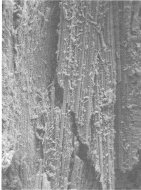
FIG. 13— Splitting within transverse ( 90^\circ ) ply (X88).
