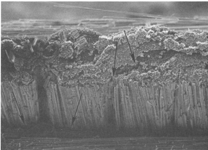
FIG. 12—Axial cracking in 0^\circ ply of 0^\circ/90^\circ composite. Note separation between plies (X43).
