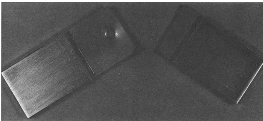
FIG. 14—Typical fatigue failure, impacted Ti-6Al-4V specimen.
